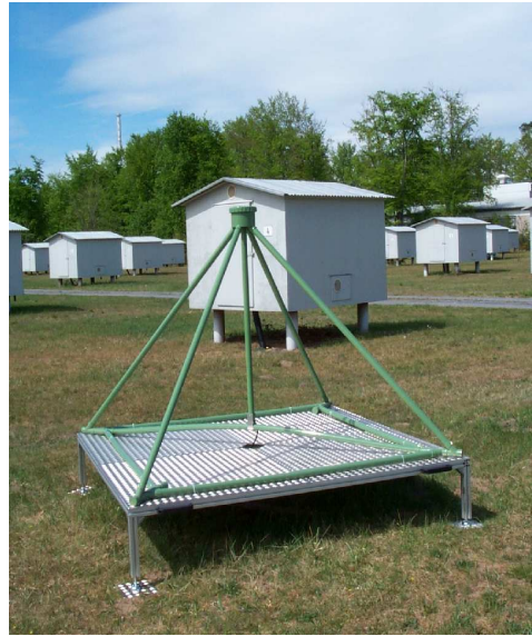
Figure 4.2: LOPES antenna in use up to end of 2009
