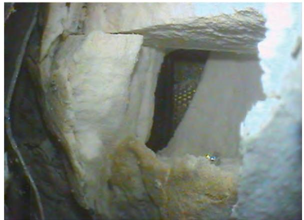
550 mm: ZrO<sub>2</sub> insulation damage under failed shroud
