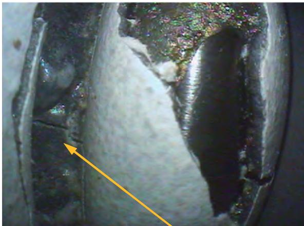
400 mm: relocated frozen melt between rods
