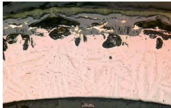
rod 7°, 270°: nitrides *inside* secondary oxide
