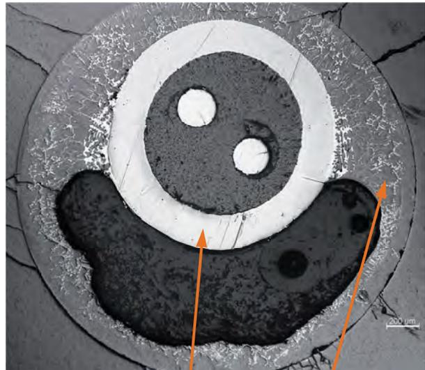
650 mm: intact Ta, relocated molten Zr completely oxidised
