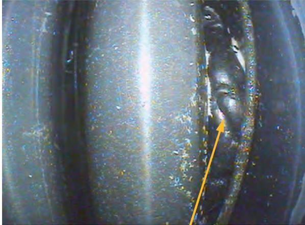
215 mm: relocated frozen melt between rod #21 and shroud
