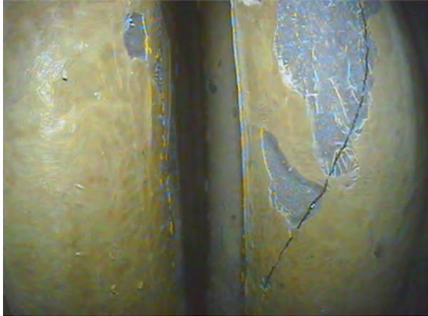
787mm; crack going through oxide layer
