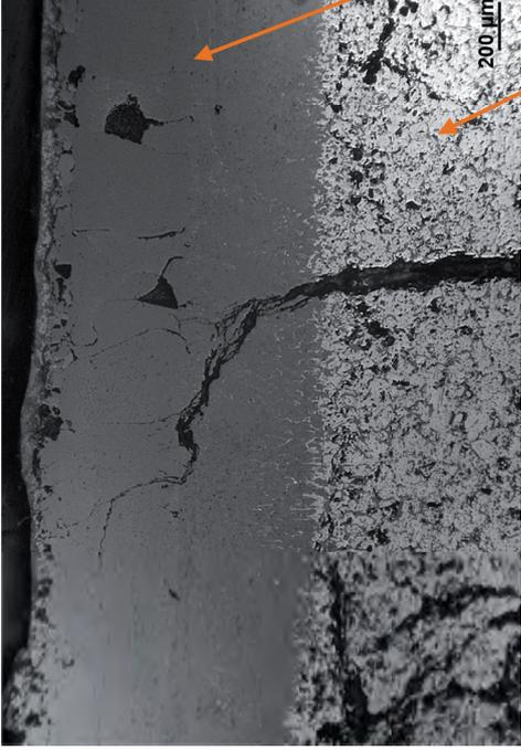
135° (highest circumference temperature): oxidised melt, very thick oxide layer with thin outer porous scale
