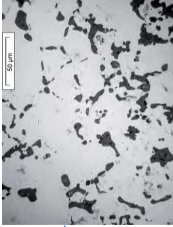
light non porous region; p precipitates area 10% → 8 wt% dissolved oxygen
