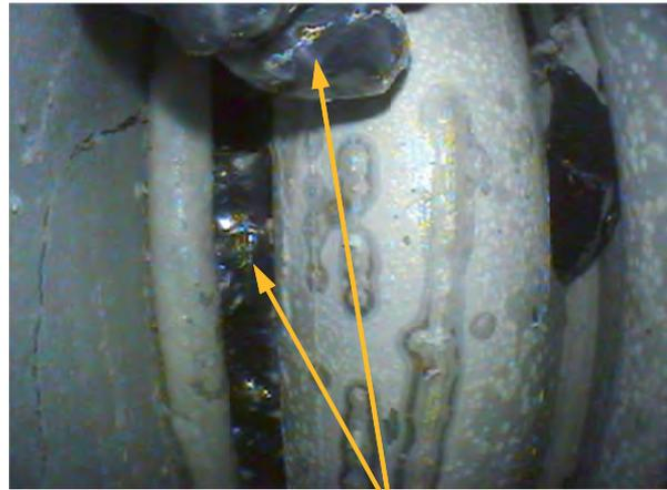
350 mm: frozen metallic melt relocated from upper elevations
