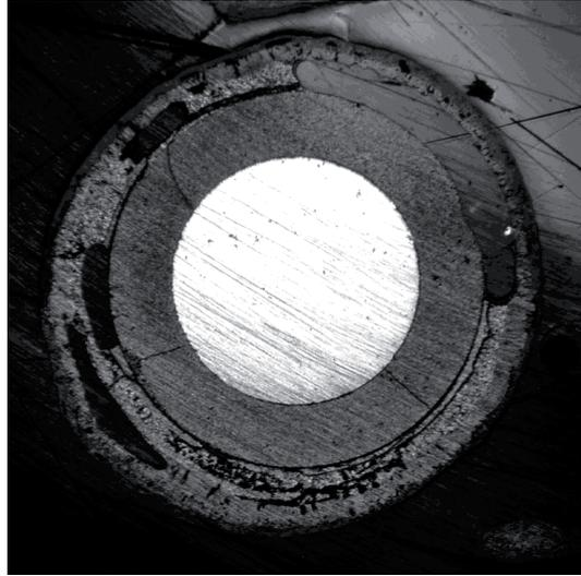
Fig.97: QUENCH-16; Cross section at elevation 550 mm depicting individual test rods 7-12.
