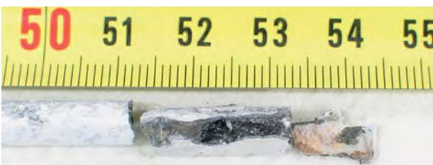
Fig. 49: QUENCH-16; Photographs of corner rod A withdrawn from the bundle after the test, 200-550 mm elevation.
