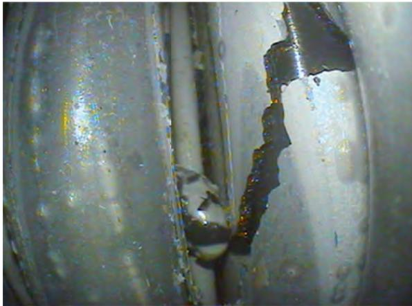
250mm; cladding failure
