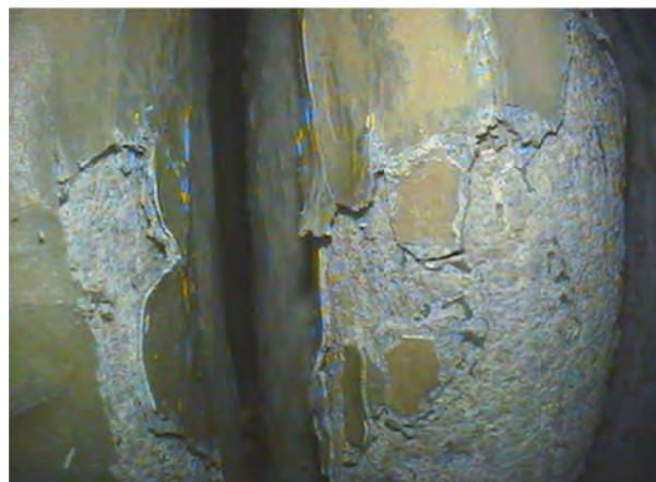
755 mm; spalling of thick oxide scales
