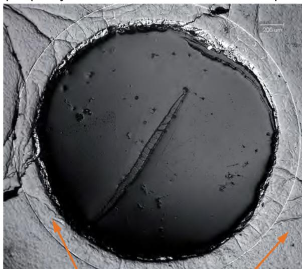
750 mm: residual completely oxidised Zr relocated from upper TCRC 13 and stuck at the surrounded  $ZrO_2$  pellet
