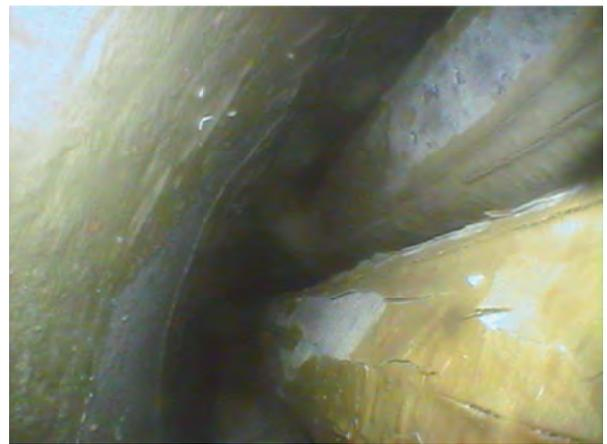
1000 mm: spalling of yellowed ZrO<sub>2</sub> scales from oxide layer
