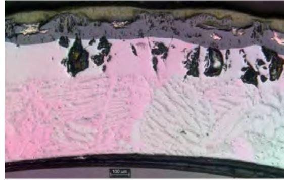
rod 3, 90°: nitrides between two oxide sub-layers
