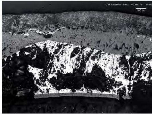
rod 2, 45°: residual nitrides between two outer oxide sublayers, inner oxide at the melt boundary
