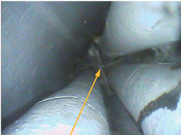
450 mm: cracks going through the oxidised cladding; piece of relocated oxidised GS#3
