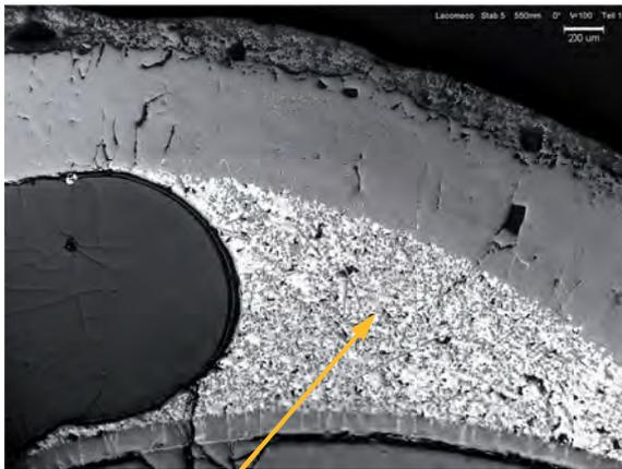
rod 5, 0°: melt with ceramic precipitates (oxygen content in prior melt 18 wt%)
