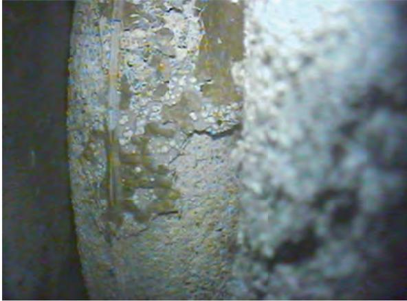
775mm, spalling at rod#9 (centre); rod#21 (right); bottom of yellowed oxide
