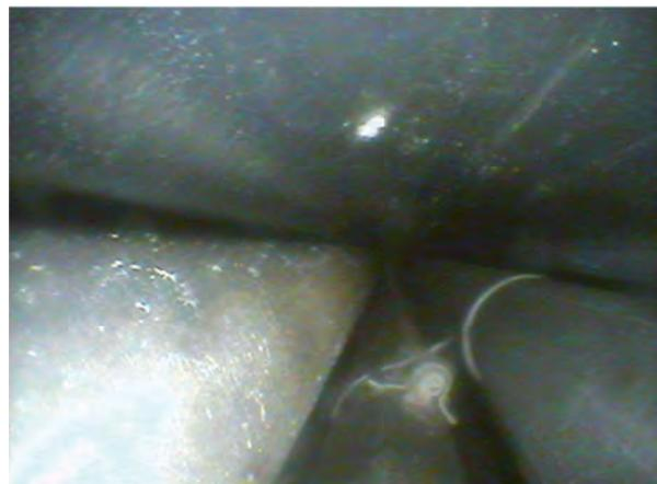
1150 mm: intact dark oxidised surface of claddings
