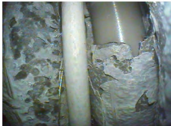
595 mm; palling of white oxide; cladding failure
