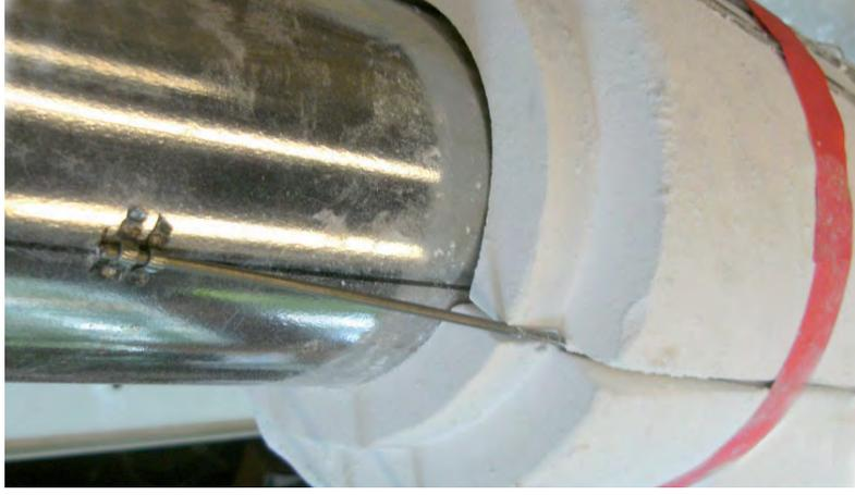
TC installed at shroud
