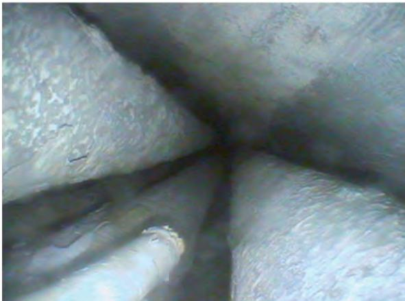
650 mm: absence of upper spalled oxide scales
