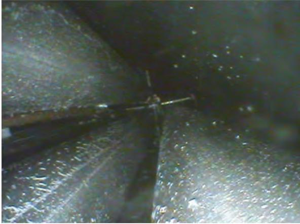
0 mm: relocated small oxidised debris adhered to surface of lightly oxidised claddings
