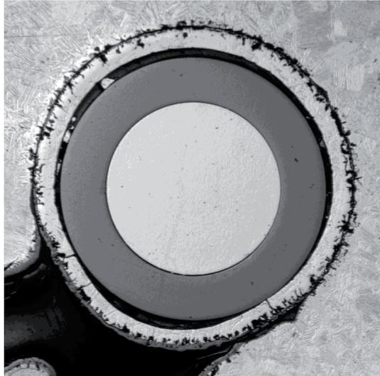
Fig.81: QUENCH-16; Cross section at elevation 350 mm depicting individual test rods 13-18.
