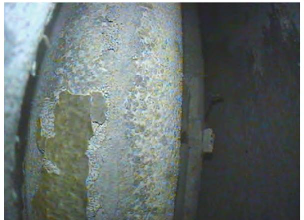
670 mm, spalling at rod#21; shroud
