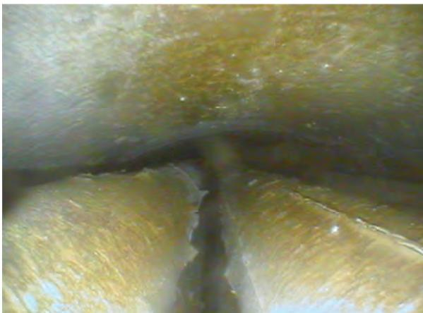
700 mm: spalling of yellowed ZrO<sub>2</sub> scales from oxide layer
