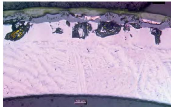
rod 9, 180°: nitrides between two oxide sub-layers
