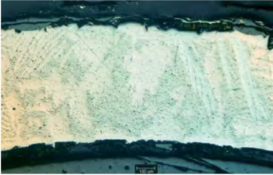
0°: nitrides; outer ZrO<sub>2</sub> spalled; homogeneous ZrO<sub>2</sub> developed during quench
