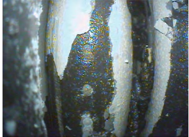
280mm, spalling at rods #9 and #21
