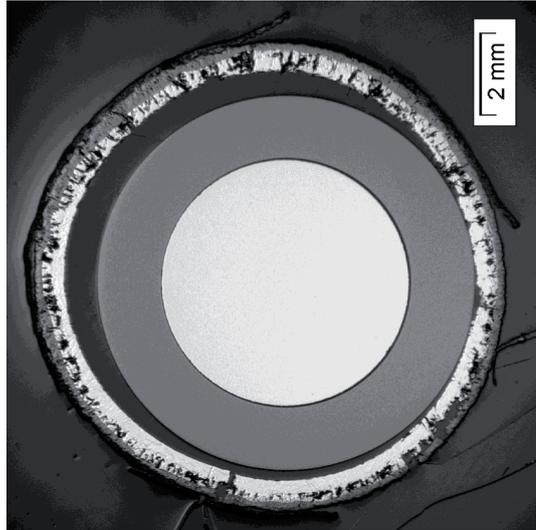
Fig.114: QUENCH-16; Cross section at elevation 850 mm depicting individual test rods 19-21.
