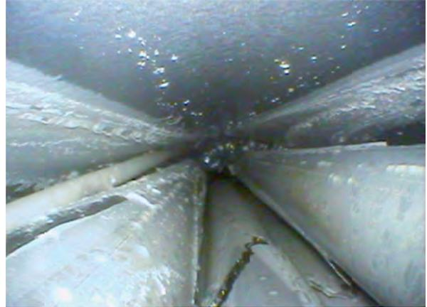
350 mm: oxide cracks; between rods – melt relocated from upper elevations
