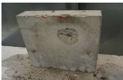
Result of an ablation experiment. Concrete was exposed to microwave radiation at f=2.45 GHz and an RF power of 8 KW for about 15 s.
