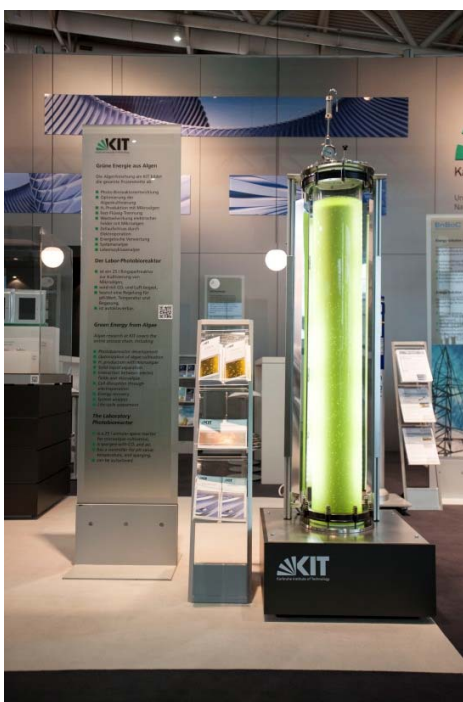
Annular airlift photobioreactor with a half shell of the LED illumination at the main KIT stand, Hannover Messe 2012.
