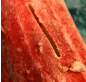
Figure 11.11.: Bone Cut from robot is smooth and consistent.
