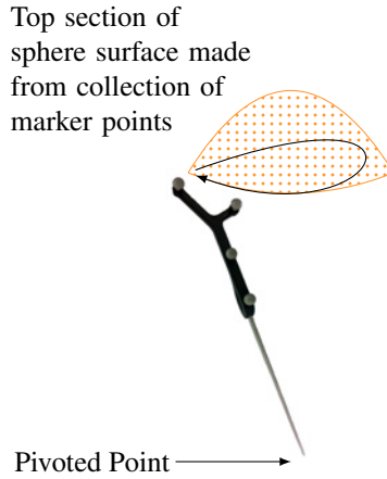
Figure 2.10.: Pivotalisation with Optically Tracked Tool
