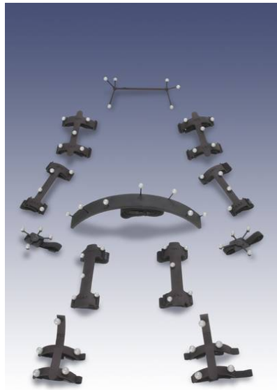
Figure 2.8.: Example marker configurations
