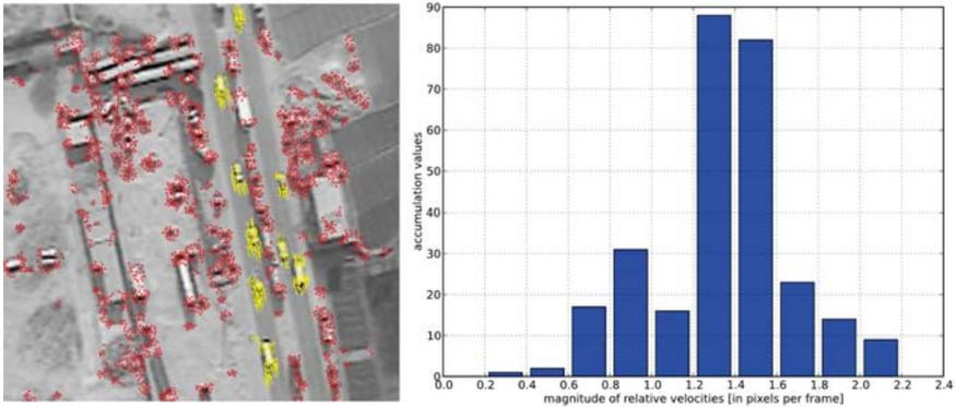
**Figure 2.2:** Example scene with stationary local features in red and moving local features in yellow. The histogram visualizes the related vector absolutes in pixels.
