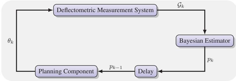
**Figure 1.1:** Planning takes place in a loop. At time step  $k$  a sensor configuration  $\theta_k$  is chosen based on the current estimation of the surface. This leads to a new measurement, which in turn is used to update the estimation  $p_k$ .
