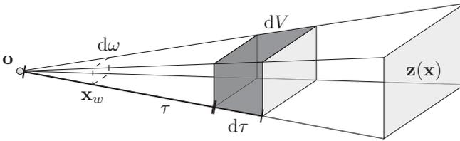
**Figure 3.3:** Backscattering of a volume element on sight line
