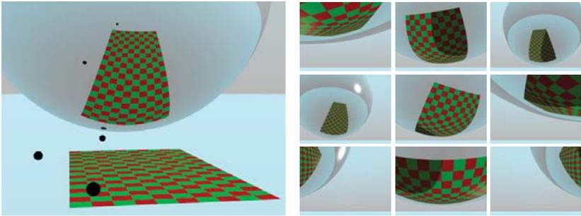
(a) Simulated scene with the studied object (specular sphere) at the initial position, three cameras (marked with the black spheres), and the pattern screen.
