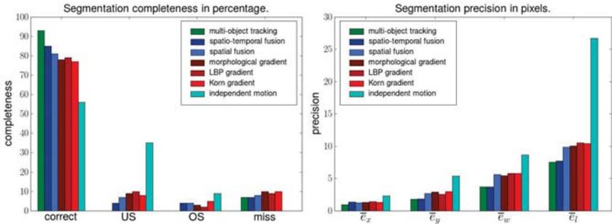
**Figure 3.3:** Evaluation of completeness (left) and precision (right) of object segmentation using different approaches. Completeness is given in percentage of correct, under-segmented (US), over-segmented (OS), and missed segmentations, precision is given in mean pixel error for object position ( $x, y$ ) and size ( $w, l$ ).
