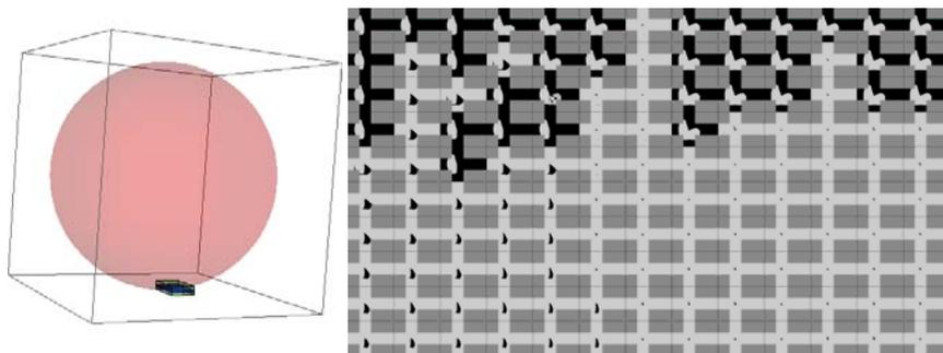
**Figure 4.1:** Right: location of voxelized volume and a “slice” of reconstructed voxels; left: resulting NVMs reconstructed from a sequence of 200 observations.
