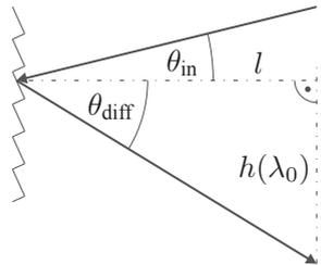
**Figure 3.1:** Relationship between height  $h(\lambda_0)$  and center wavelength  $\lambda_0$  using the grating equation.
