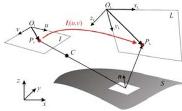
**Figure 2.1:** Principle of the deflectometric registration from [Wer11].
