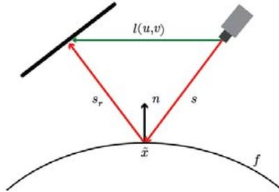
**Figure 2.1:** This figure shows the inverted deflectometric light path of a ray from the camera pixel  $(u, v)$  to the display (red arrows). A deflectometric measurement provides a mapping  $l(u, v)$  from camera pixel to display points (green arrow).
