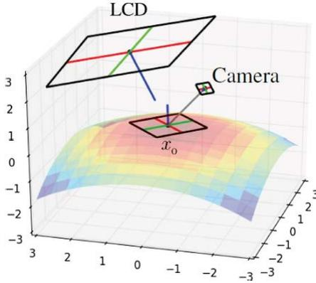
**Figure 4.1:** This figure depicts the sensor configuration, i.e. the focus point  $x_0$  with the attached frame and the camera as well as the LCD.
