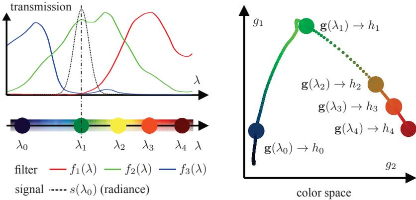
**Figure 1.2:** Measuring principle: A multichannel camera with optical filters ( $f_1, f_2, f_3$ ) acquires a spectrum  $s(\lambda_0, \lambda)$  which is centered around  $\lambda_0$ . Each center wavelength  $\lambda_0$  causes a unique grey value vector  $\mathbf{g}(\lambda_0)$  in color space. After an acquisition the center wavelength can be deduced from the color coordinate  $\mathbf{g}(\lambda_0)$ . (partly taken from [TB12])
