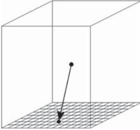
**Figure 2.2:** Rasterized cube surface as the parameterization of solid angles as viewed from the center of the cube.
