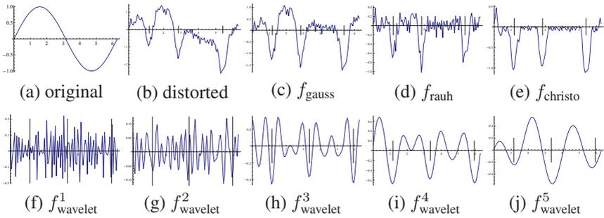
**Figure 4.1:** Comparison of filters (c)-(j) in spatial space to amplify defects in distorted signal (b) of signal (a).
