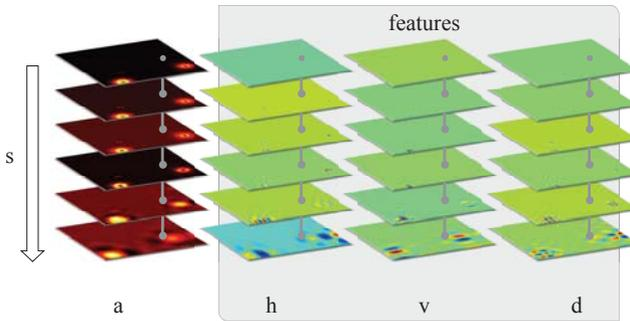
**Figure 4.2:** The feature vector contains each detail coefficient (horizontal, vertical and diagonal) of the (discrete, stationary) wavelet transform in several scales.
