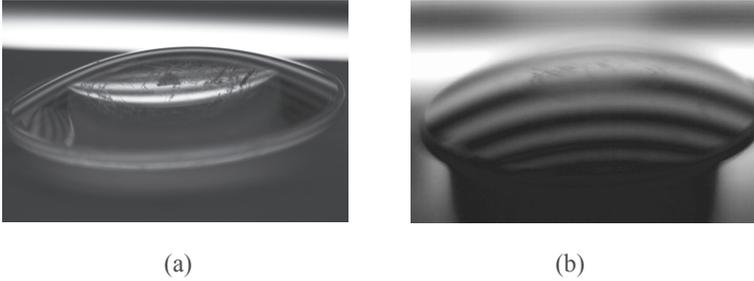
**Figure 2.2:** Images of a glass lens in the visible light spectrum between 400 – 700  $nm$  (a) and in the thermal infrared spectrum between 8 – 14  $\mu m$  (b). In the visible spectrum the stripe pattern in the background is seen multiple times because of internal reflections, while the thermal spectrum shows only the reflection on the surface.
