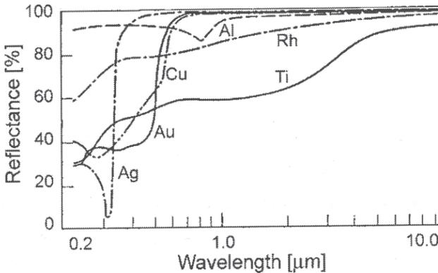
**Figure 2.1:** Reflectance of different metals as a function of wavelength. With increasing wavelength most metals become nearly fully reflective. (Source: [Dan10])
