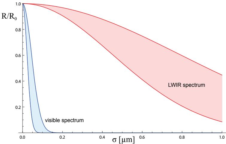
**Figure 2.3:** Ratio of the reflectances  $R/R_0$  as a function of  $\sigma$ , the mean square roughness of the surface. The blue plot stands for the visible spectrum and the red plot for the LWIR spectrum ( $8 - 14\mu m$ ). The longer wavelength shows a significant increase in reflectivity for the same surface roughness.
