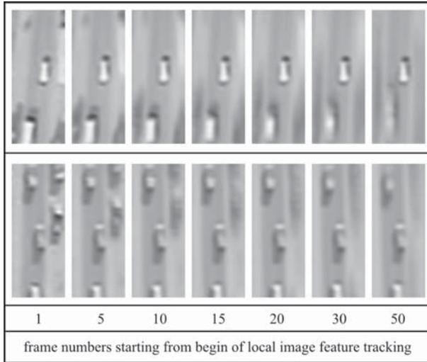
**Figure 3.2:** Temporal fusion (image stacking) for two local features tracked along 50 frames [TK12b]. The central vehicle is moving and stacked.
