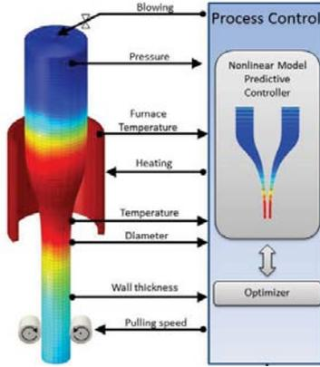
**Figure 3.1:** Industrial glass drawing process
