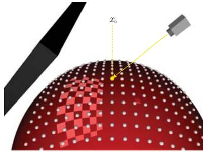
**Figure 4.2:** The sensor configuration set  $\Omega$  is partially discretized by choosing the focus point component from a finite set. The figure depicts the focus points as balls distributed on a grid.
