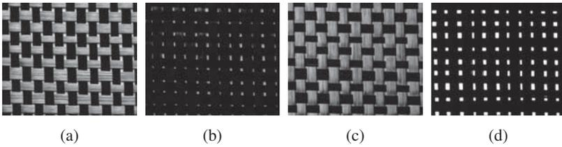
**Figure 4.1:** Example for the investigation of a weave structure by variable lighting: (a) perpendicular to weft yarns, (b) not perpendicular to a yarn direction, (c) perpendicular to warp yarns, (d) transmitted light [VWZ12].
