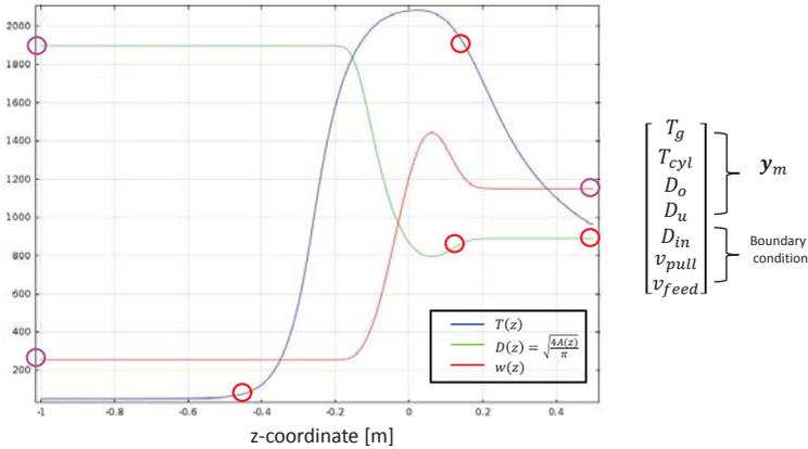
**Figure 3.2:** The stationary solution of glass forming process and the illustration of sensors
