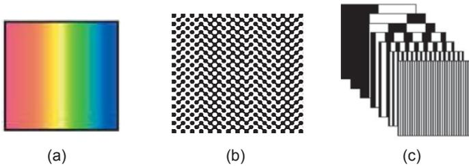
**Figure 3.1:** Examples for different categories of coding techniques: (a) color pattern for direct coding of the position, (b) resulting pattern of a De Bruijn graph, (c) binary pattern sequence of a time-multiplexing method (Source: [SPB04]).
