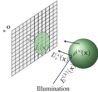
**Figure 3.2:** Illustration of the radiometric scene
