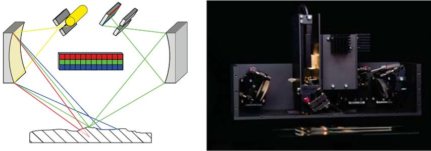
**Figure 1.1:** On the right, prototype of a CCT sensor. On the left, principle optical setup of a CCT sensor with highlighted RGB line scan sensor. Important detail: Only the green illustrated wavelength can reach the RGB sensor.
