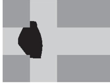
**Figure 2.3:** Unfolded normal vector map. Black pixels mark the allowed, light gray – the excluded directions.
