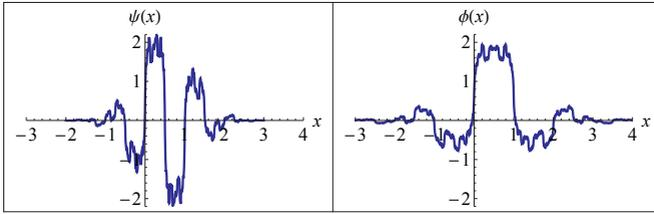
**Figure 3.1:** Biorthogonal wavelet with five vanishing moments and corresponding scaling function.
