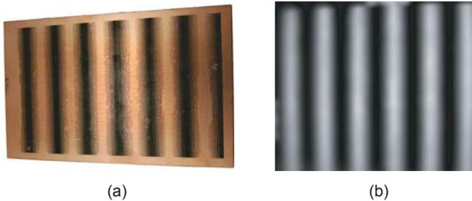
**Figure 3.2:** Examples for a static code pattern for the thermal infrared spectrum on a printed copper board (a). The imprinted color reveals its temperature due to its high emissivity, while the bare copper exhibit near zero emissivity. By modulating the ratio of areas with high and low emissivity by the use of dithering, even gray values can be produced in the thermal image (b) while the whole pattern has actually the same temperature.
