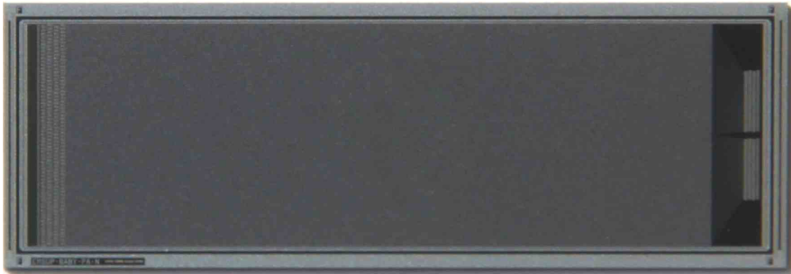
Figure 5.12.: Picture of the Baby_PA. The sensor has an integrated pitch adapter (on the right) in the first metal layer.
