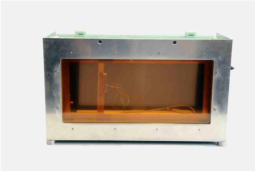
Figure 4.2.: Front view of the irradiation box. The objects to be irradiated are fixed to the aluminium frame that is inserted into the box. During irradiation, the box is flooded by cooled N_2 , setting the temperature in the box to about -30^\circ C in order to avoid annealing.
