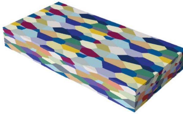
Fig. 4: Elongated Voronoi network model [6] to describe the zeolite layer with coffin-shape crystals.
