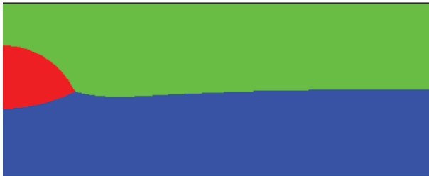
Figure 3.9.: The peritectic \gamma -solid growth on top of a properitectic \delta -substrate. The dynamics of dissolution is driven by diffusion of solute in the liquid phase.
