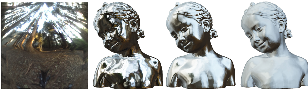
Figure 7.6: This image shows screen-shot of a rendering with SATs created from octahedron environment maps to adjust surface glossiness at real-time. The creation of the 512 \times 512 pixel SAT takes about 3.3ms on a NVIDIA 8800GTX. Illustration: Engelhardt and Dachsbacher [2008].
