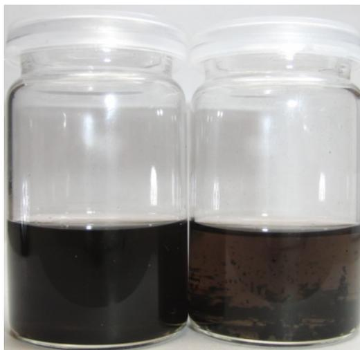
**Figure A14.** Digital photograph of the dispersions prepared after 1 minute ultrasonication of 1 mg of **SWCNT-1** (left) and **SWCNT-0** (right) in 10 mL of  $\text{CHCl}_3$  after 5 days.
