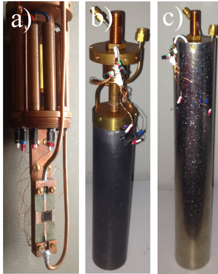
Figure 3.7: a) Sample glued and bonded to a sample holder. Set of dc twisted pairs and a couple of microwave lines are exploited. b) Sample holder covered by a superconducting lead shield. c) Sample holder with the second \mu -metal shield attached, ready to be inserted into a cryostat.
