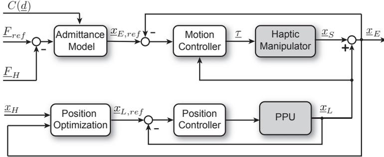
Fig. 6.3.: Control overview of the haptic interface.
