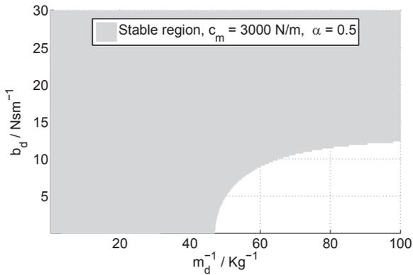
Fig. 6.10.: Stability boundaries of the semi-mobile haptic interface in the  $(m_d, b_d)$  parameter space for human compliance reduced by a factor  $\alpha = 0.5$ .
