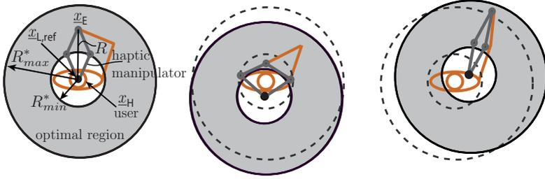
Fig. 6.5.: Prepositioning algorithm for the SMHI with mirror setup configuration.
