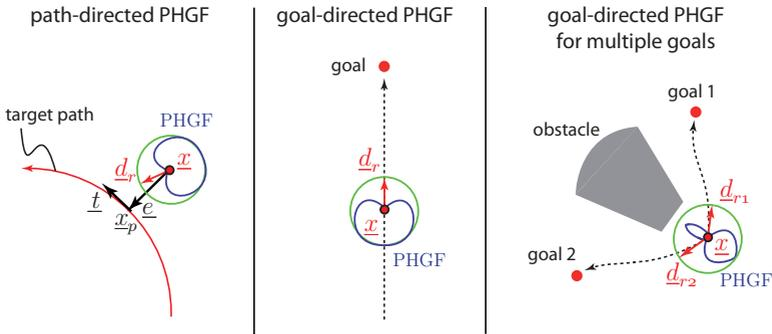
Fig. 4.7.: PHGFs for different types of haptic guidance. In path-directed guidance (left), the user motion is controlled so as to be along a certain path. In goal-directed guidance (middle), the user is guided toward a specific target. In goal-directed guidance with obstacles (right), the user is kept away from obstacle regions. When goal-directed guidance for multiple simultaneous goals is used (right), the user can choose which target he/she wants to walk to.
