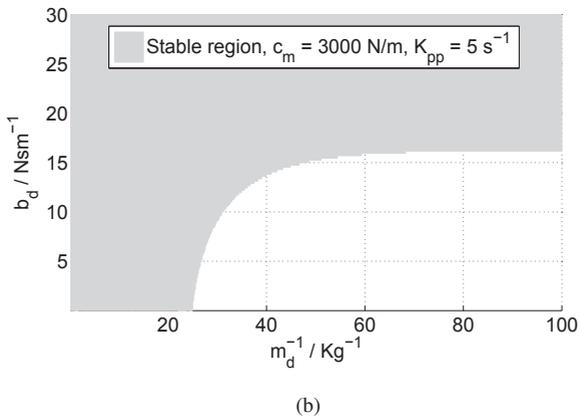
Fig. 6.8.: Stability boundaries of the semi-mobile haptic interface in the  $(m_d, b_d)$  parameter space with (a) high position gain of PPU  $K_{pp} = 500 \text{ s}^{-1}$ , and with (b) low position gain of PPU  $K_{pp} = 5 \text{ s}^{-1}$ .
