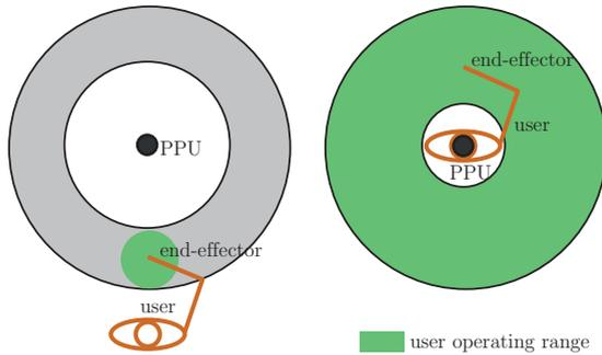
Fig. 7.7.: Operating range of the user at a certain position: with the old setup (left), and with the new setup (right).
