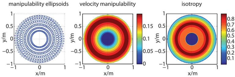
Fig. 7.5.: Manipulability ellipsoids (left), velocity manipulability (middle), and isotropy (right) in the reachable workspace of the manipulator.
