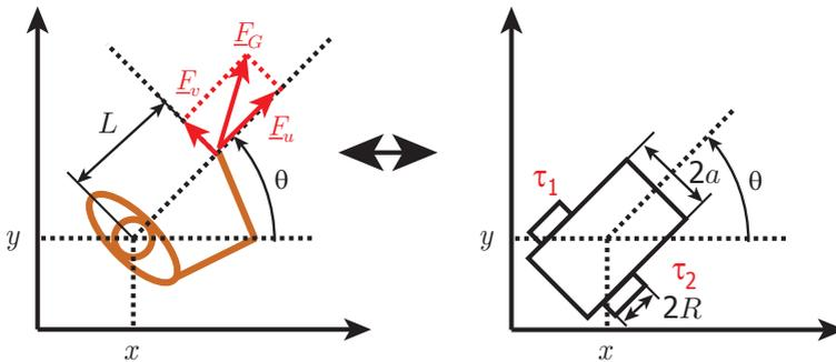
Fig. 5.1.: User modeled as a car-like wheeled mobile robot moving on a plane.
