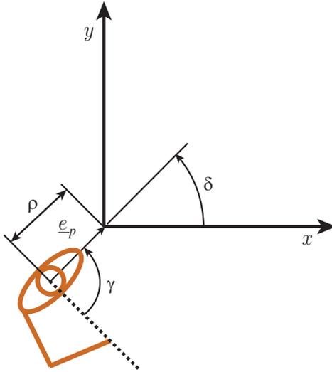
Fig. 5.2.: Posture regulation problem for an underactuated system.
