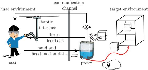
Fig. 1.1.: Extended range telepresence system with haptic interaction.
