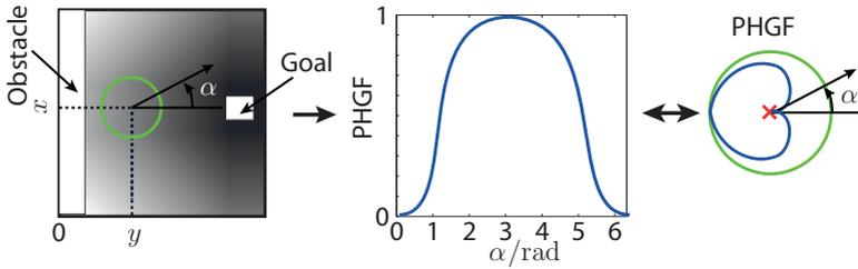
Fig. 4.3.: Normalized PHGF for an exemplary scenario. In the middle picture, the PHGF is plotted for a given position as a function of the orientation. In the right picture, the same function is displayed in polar coordinates (blue line) inside the unit circle (green line).
