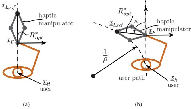
Fig. 6.4.: Two prepositioning algorithms for the SMHI with frontal setup configuration based on optimal manipulability. (a) The PPU is prepositioned at the maximum distance from the user. (b) The PPU is prepositioned by considering the instantaneous path curvature.
