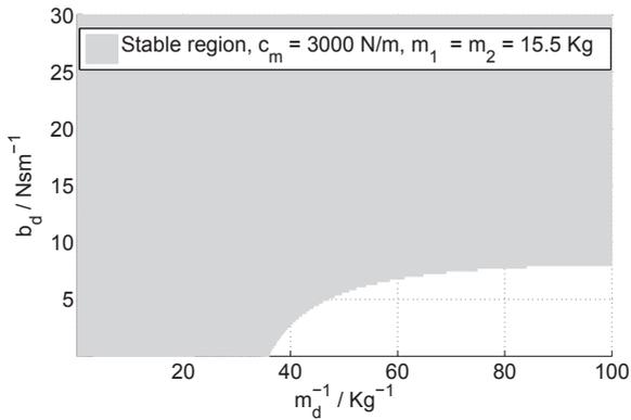
Fig. 6.9.: Stability boundaries of the semi-mobile haptic interface in the  $(m_d, b_d)$  parameter space for manipulator mass  $m_1 = m_2 = 15.5 \text{ Kg}$ .
