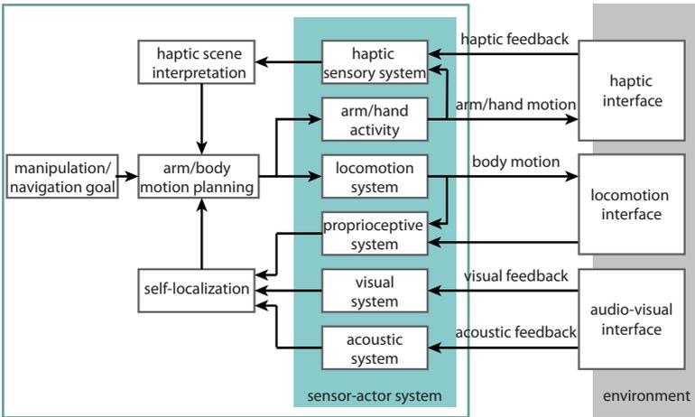
Fig. 3.3.: Abstract representation of sensory, actuator, and cognitive processes of the user in extended range telepresence with haptic guidance.
