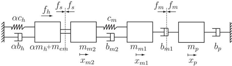
Fig. 6.6.: Compliant model of semi-mobile haptic interface and human.
