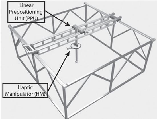
Fig. 2.2.: Model of an exemplary Semi-mobile Haptic Interface.
