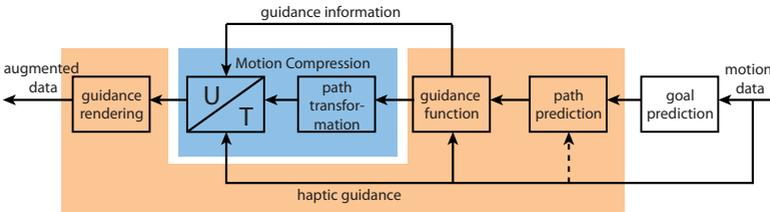
Fig. 3.4.: Algorithmic framework of the proposed wide-area haptic guidance.
