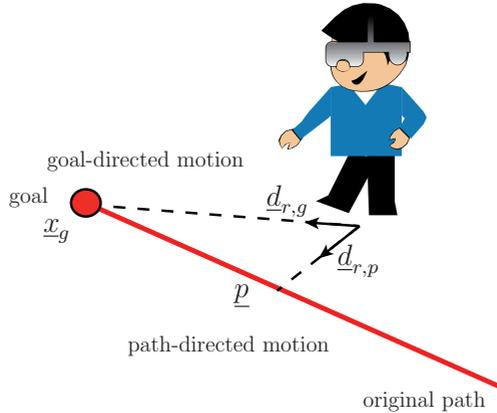
Fig. 4.4.: Human navigation models. In the goal-directed locomotion model, the goal position is the reference point. In the path-directed locomotion model, the user tries to return to the originally planned target path and the reference point is an arbitrary point on the path.
