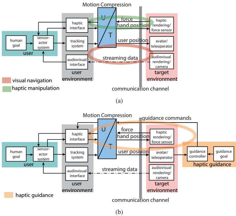
Fig. 3.2.: Data flow in the extended range telepresent system, (a) with haptic feedback, and (b) with additional haptic guidance.
