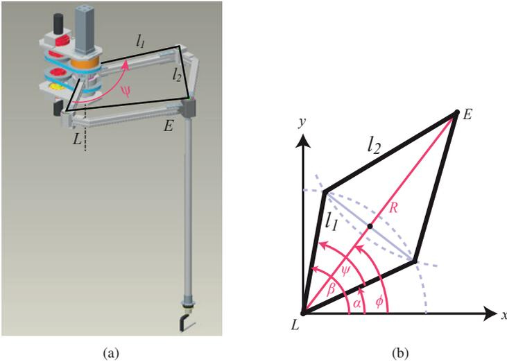
Fig. 7.3.: New manipulator design. (a) 3D-CAD Model of the haptic manipulator as a Parallel Selective Compliance Assembly Robot Arm (SCARA) with four links, two proximal links of length  $l_1$  and two distal links of length  $l_2$ . (b) Geometrical model of the manipulator.
