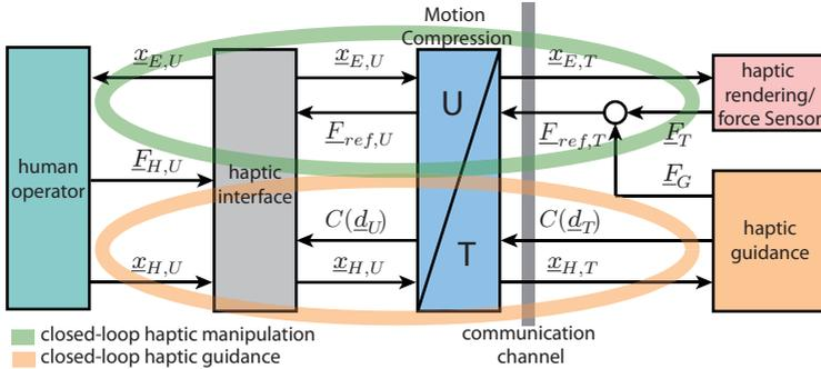
Fig. 6.2.: Overall haptic control of the extended range telepresence system with haptic guidance.
