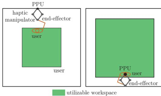
Fig. 7.8.: Utilizable area in the user environment: with the old setup (left), and with the new setup (right).
