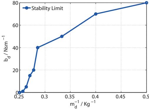
Fig. 7.9.: Experimentally identified limit of stability region of the admittance-controlled semi-mobile haptic interface.
