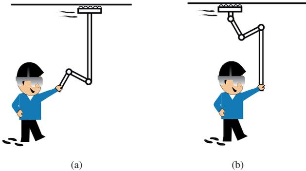
Fig. 6.1.: Two possible system configurations for the SMHI. (a) In the *frontal configuration*, the haptic manipulator is opposite the user. (b) In the *mirror configuration*, the haptic manipulator is atop the user and reflects his/her motion.
