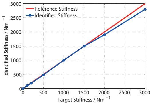
Fig. 7.10.: Experimentally identified stiffness of the admittance-controlled semi-mobile haptic interface.
