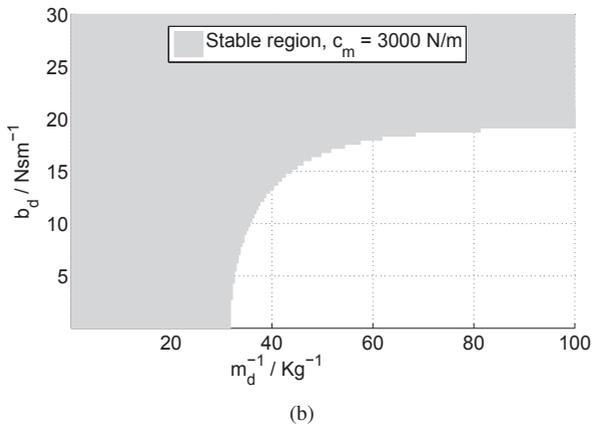
Fig. 6.7.: Stability boundaries of the semi-mobile haptic interface in the  $(m_d, b_d)$  parameter space for (a) high manipulator rigidity  $c_m = 30000 \text{ Nm}^{-1}$ , and for (b) low manipulator rigidity  $c_m = 3000 \text{ Nm}^{-1}$ .
