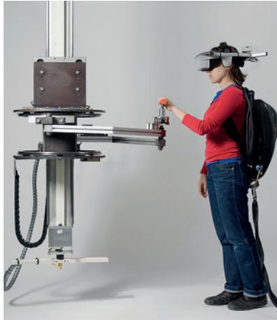
Fig. 7.1.: Prototype of the semi-mobile haptic interface with frontal setup configuration.
