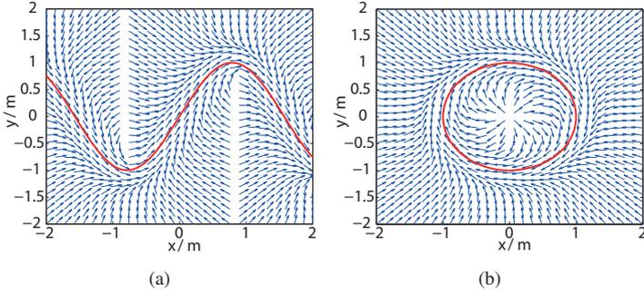
Fig. 4.5.: Guidance fields with parameters  $K_1 = 0.5$  and  $K_2 = 2$  for two exemplary target paths (red line).
