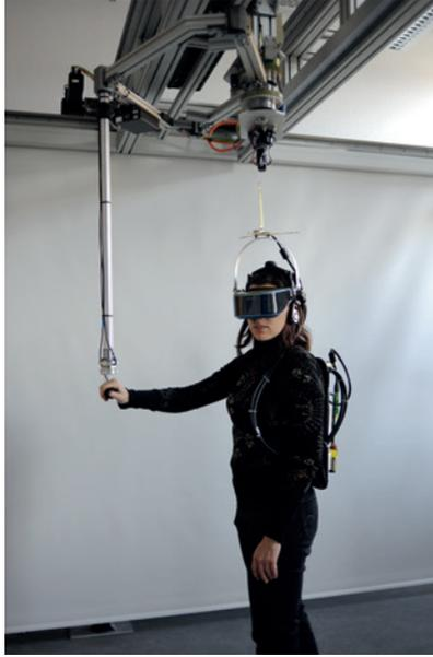
Fig. 7.12.: Human system interface of extended range telepresence system.
