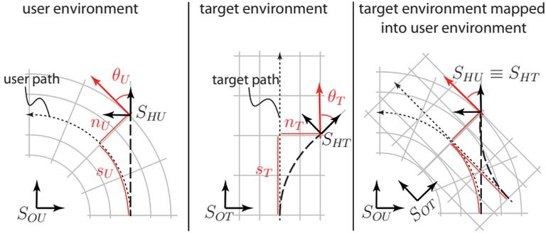
Fig. 3.5.: User position in both curvilinear coordinate systems defined by  $n$ ,  $s$ ,  $\theta$ .
