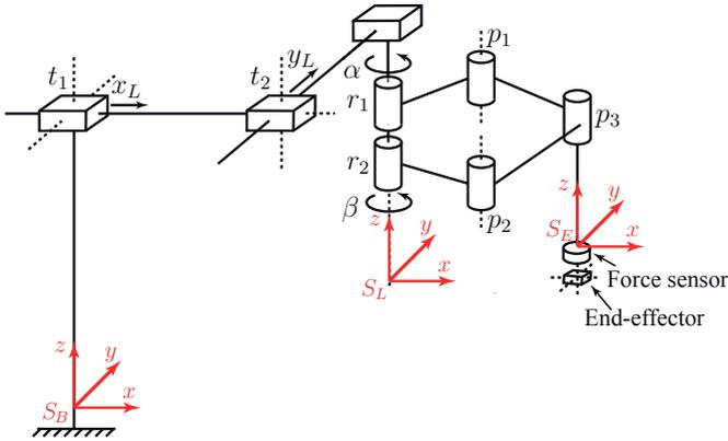
Fig. 7.2.: Kinematic model of the new semi-mobile haptic interface. Joints  $t_1$  and  $t_2$  locate the haptic manipulator at  $S_L$  (atop the user), joints  $r_1$  and  $r_2$  are actively driven and determine the end-effector pose at  $S_E$ , joints  $p_1$ ,  $p_2$ , and  $p_3$  are passive. This haptic interface is redundant in the planar degrees of freedom.
