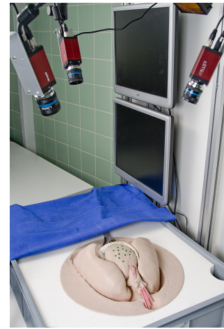
Figure 6. In computer-assisted beating heart surgery, an intervention area of a beating heart should be visually stabilized. With regard to this application, the artificial beating heart is observed by a camera system.
