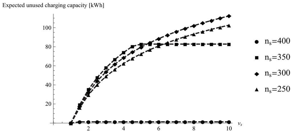
Figure 7.25: Unused capacity arising from capacity protection for  $C = 1760$
