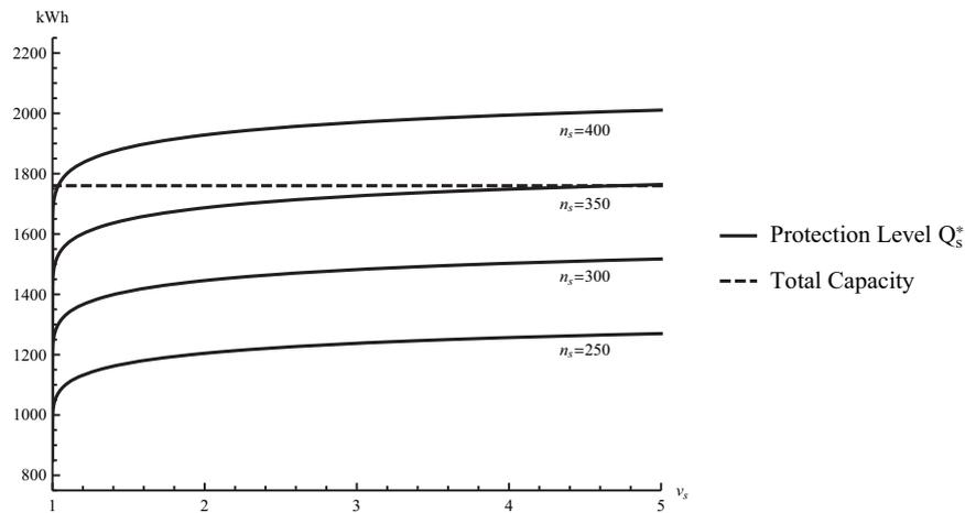
Figure 7.22: Optimal protection level over different spot valuations,  $v_s \in \{1, 5\}$
