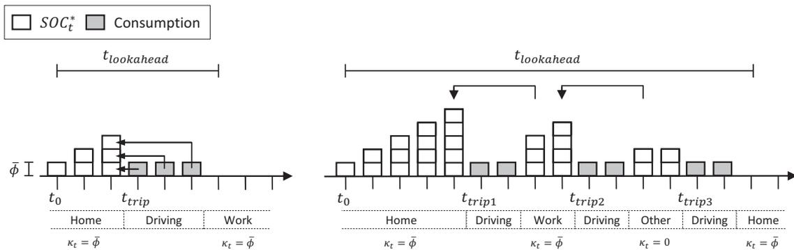
**Figure 6.12:** Determination of critical battery level  $SOC_t^*$  (For illustration purposes I simplify consumption per time slot to match  $\bar{\phi}$ .)
