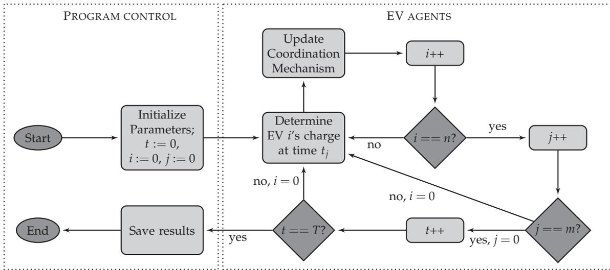
Figure 7.7: Model work flow for time-based aggregation with charging granularity
