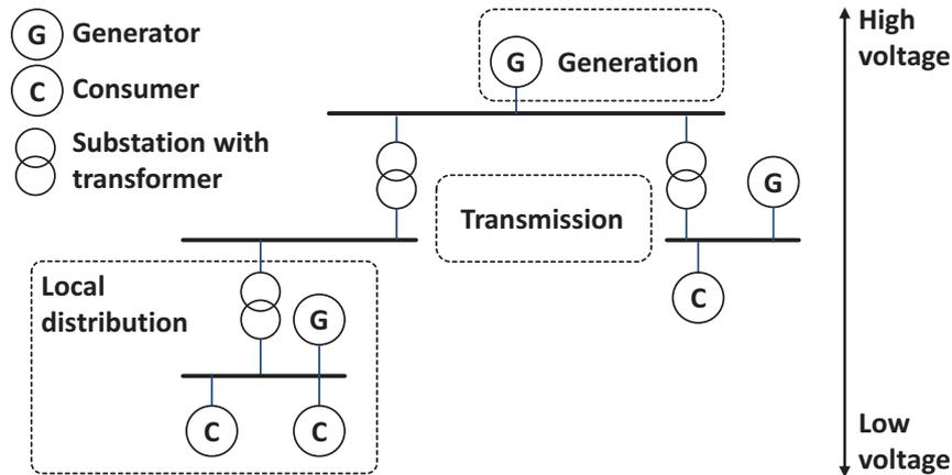
Figure 2.4: Basic structure and components of the electricity system
