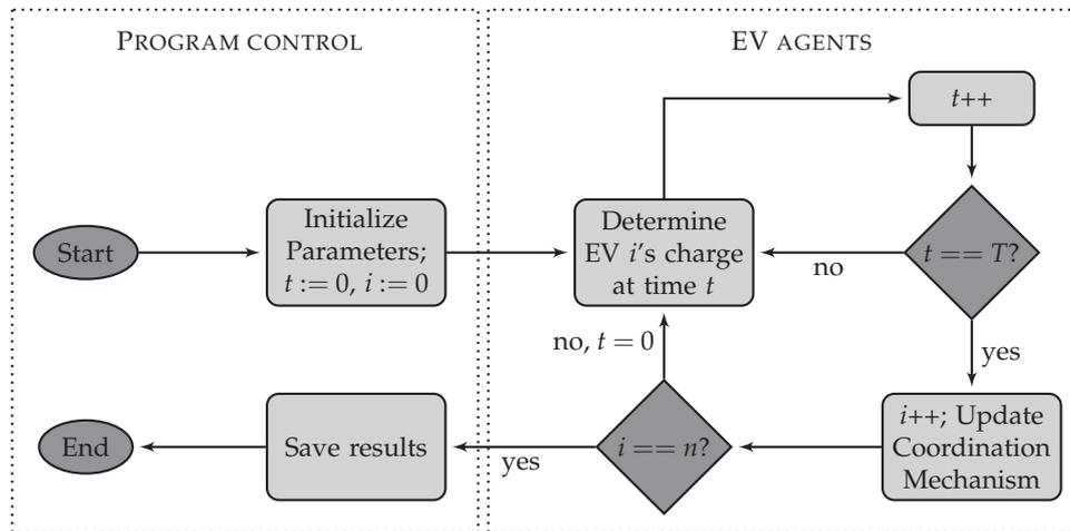
Figure 7.6: Model work flow for vehicle-based aggregation
