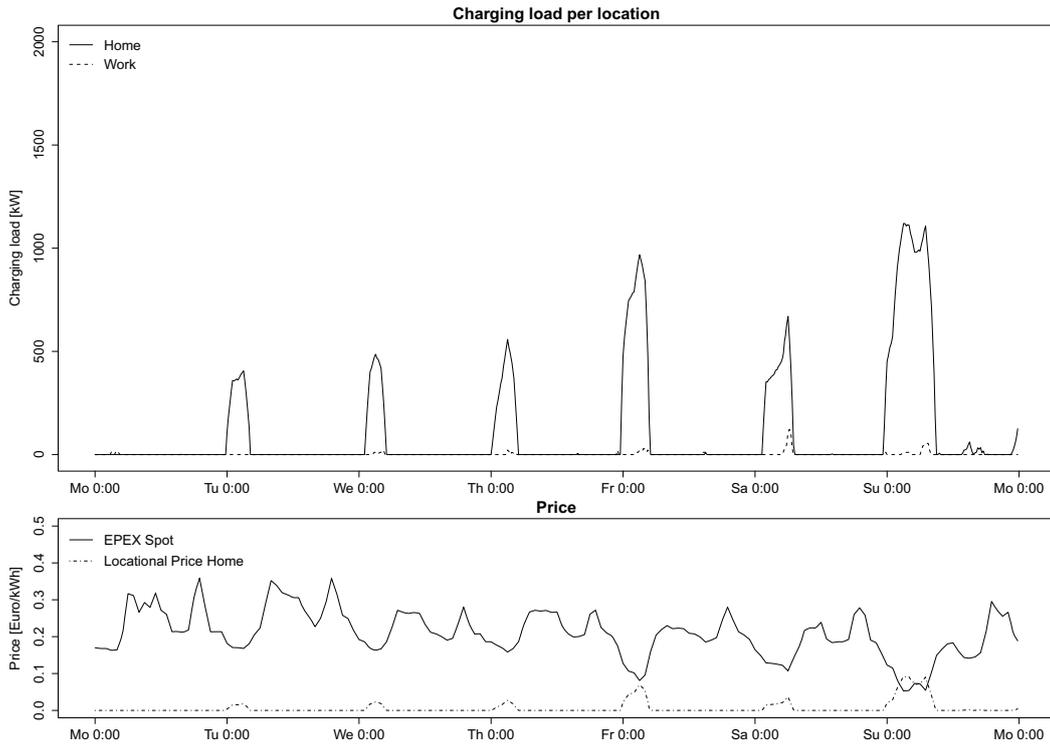
**Figure 7.9:** Aggregate load under optimal smart charging with area pricing ( $\bar{\phi} = 11kW$ ,  $SOC_0 = 100\%$ ,  $SOC_T = 90\%$ )
