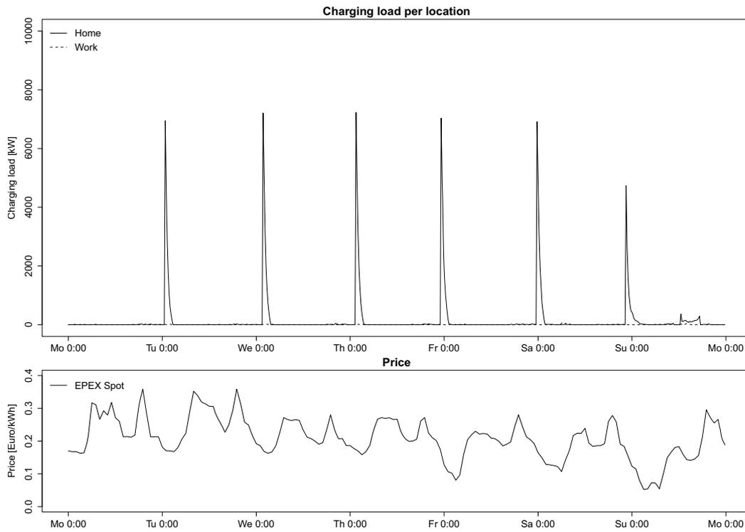
**Figure 7.4:** Aggregate Load under heuristic smart charging ( $\bar{\phi} = 11kW$ ,  $SOC_0 = 100\%$ ,  $SOC_T = 90\%$ ,  $p = 0.3$ )
