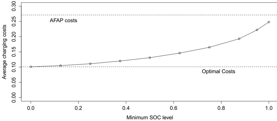
**Figure 6.17:** Average charging costs for different minimum SOC levels (11kW,  $SOC_0 = SOC_T = 0.5$ )
