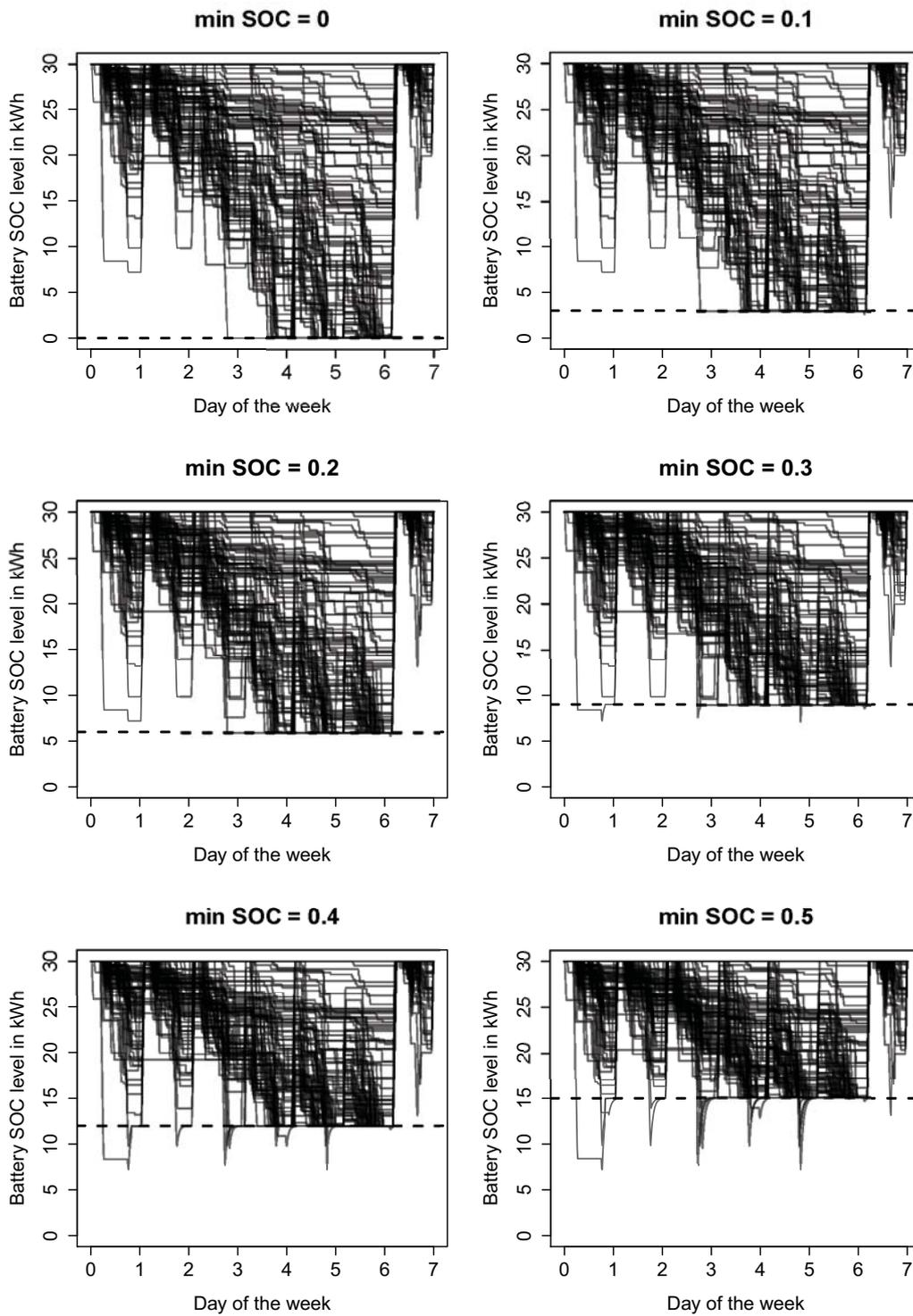
Figure 6.9: Cost-optimal SOC trajectories for different minimum thresholds
