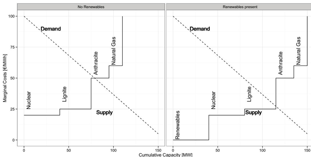
**Figure 2.3:** Merit order curve of electricity generation and the impact of renewable energy sources (Sensfuss et al., 2008)
