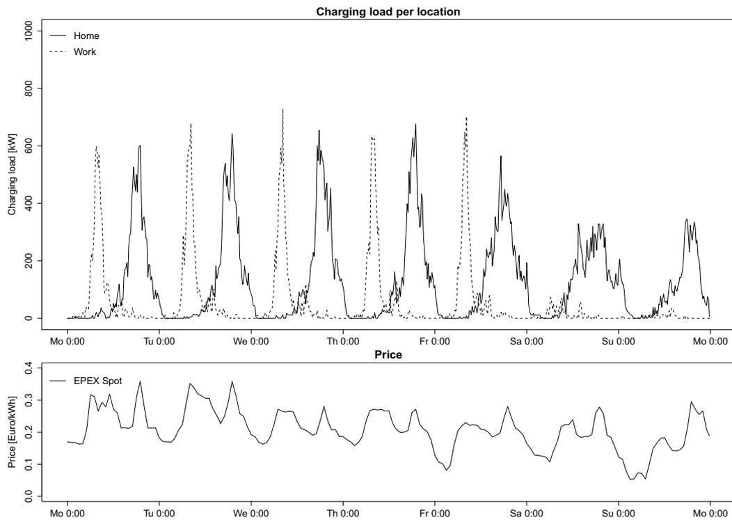
Figure 7.2: Aggregate load under AFAP charging ( $\bar{\phi} = 11kW$ ,  $SOC_0 = 100\%$ )
