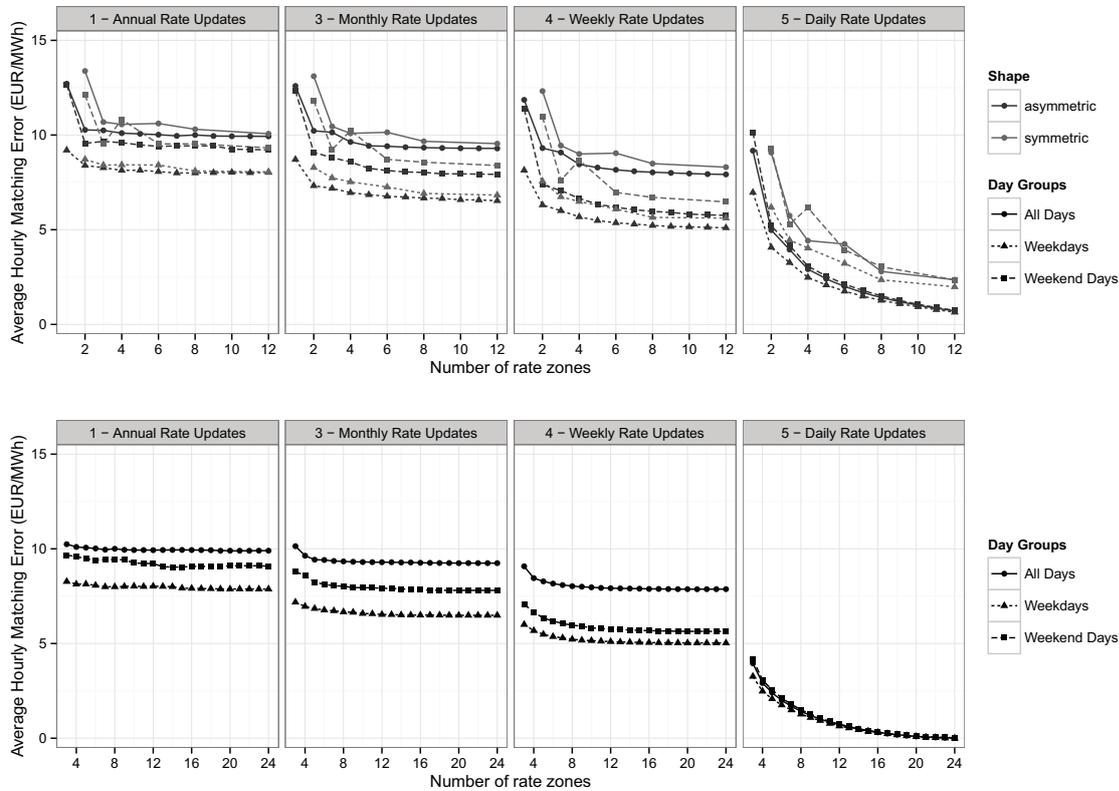
**Figure 5.8:** Efficiency of different rate granularity levels and rate zone symmetry constraints (absolute weighting of errors, upper panel:  $Z \in \{1, 2, 3, 6, 12\}$ , lower panel:  $Z \in \{2..24\}$ )
