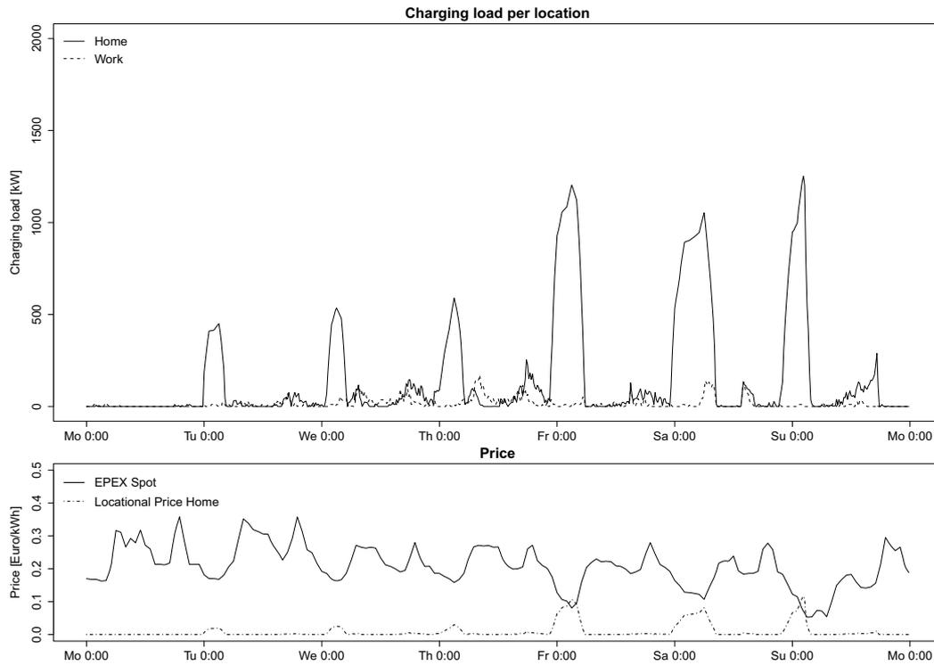
**Figure F.2:** Aggregate load under heuristic smart charging with area pricing ( $\bar{\phi} = 11\text{kW}$ ,  $SOC_0 = 100\%$ ,  $SOC_T = 90\%$ ,  $p = 0.4$ ,  $\underline{SOC} = 0.15$ )
