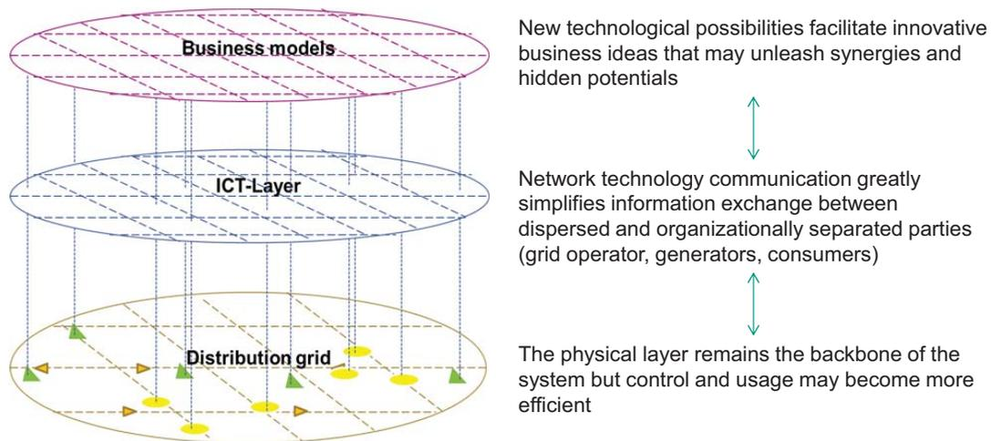
Figure 1.1: ICT connects physical and market layer in the smart grid (Block et al., 2008)
