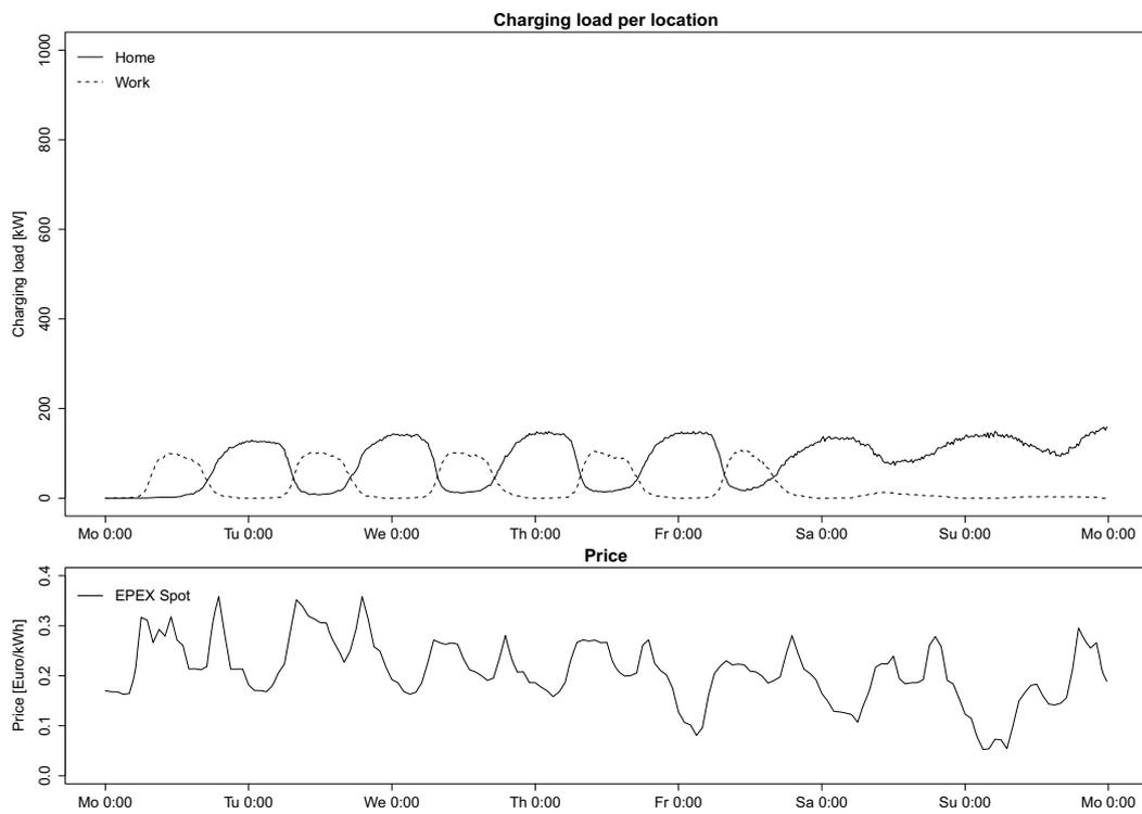
Figure 7.3: Aggregate load under minimal maximum load charging ( $\bar{\phi} = 11kW$ ,  $SOC_0 = 100\%$ ,  $SOC_T = 50\%$ )
