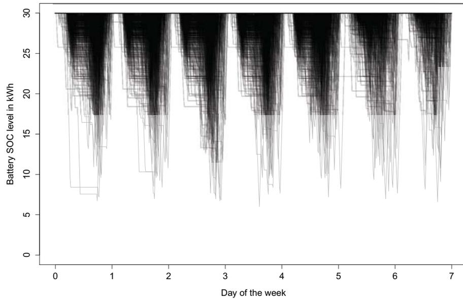
**Figure 6.6:** Battery level evolution of electric vehicle population under as fast as possible charging (charging at home, one week)
