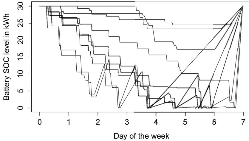
Figure 6.15: SOC level evolution of individual EVs under uniform ALAP charging
