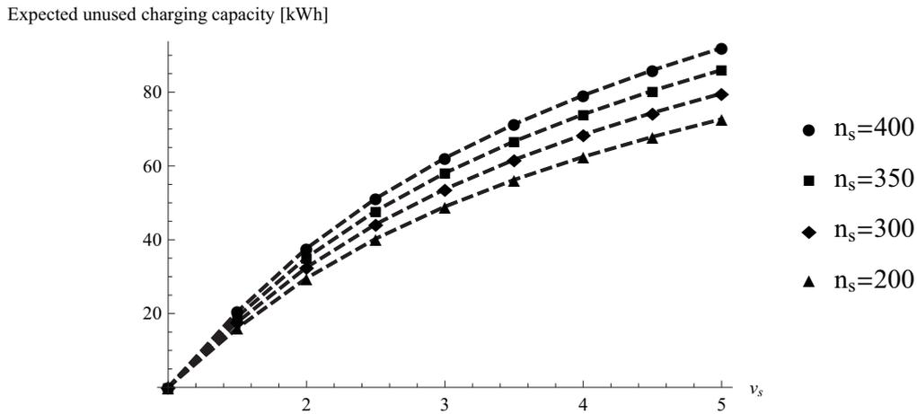
Figure 7.24: Unused capacity arising from capacity protection for  $C = \infty$
