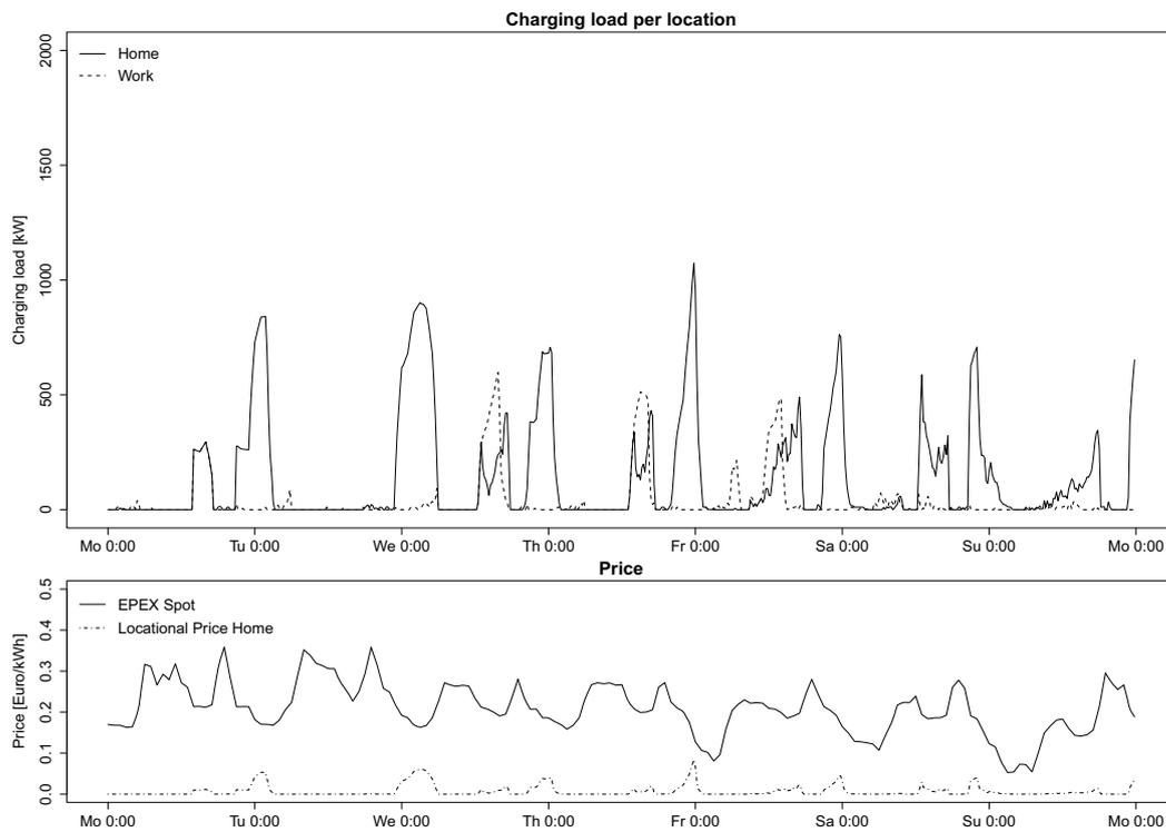
**Figure F.3:** Aggregate load under heuristic smart charging with area pricing ( $\bar{\phi} = 11\text{kW}$ ,  $SOC_0 = 100\%$ ,  $SOC_T = 90\%$ ,  $p = 0.7$ ,  $\underline{SOC} = 0.3$ )
