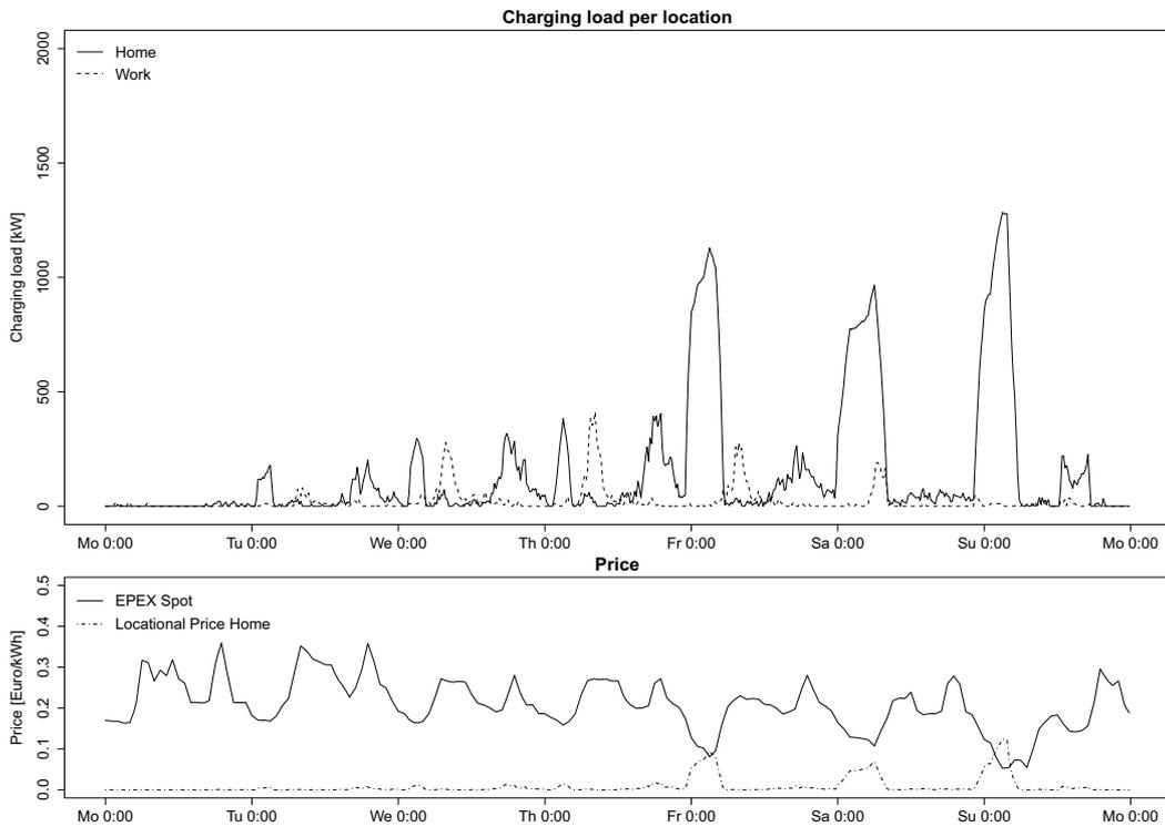
**Figure 7.10:** Aggregate load under heuristic smart charging with area pricing ( $\bar{\phi} = 11kW$ ,  $SOC_0 = 100\%$ ,  $SOC_T = 90\%$ ,  $p = 0.3$ )
