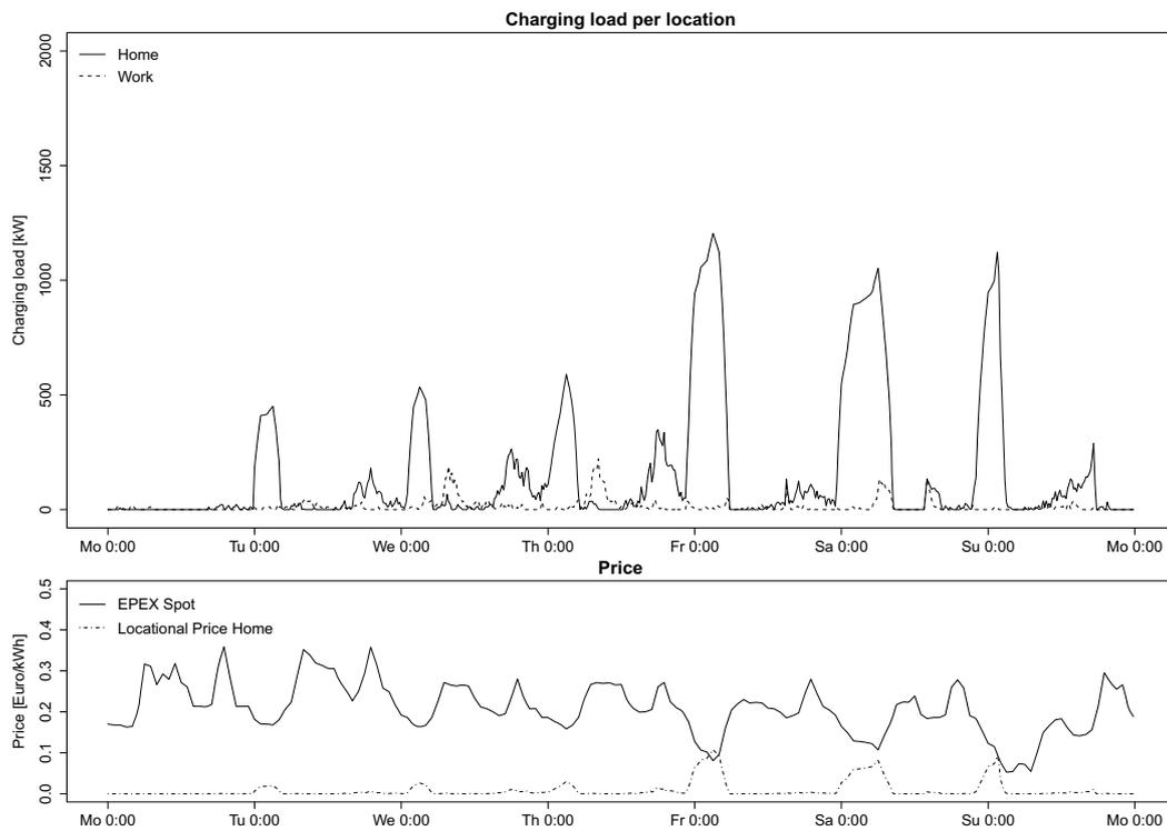
**Figure F.1:** Aggregate load under heuristic smart charging with area pricing ( $\bar{\phi} = 11\text{kW}$ ,  $SOC_0 = 100\%$ ,  $SOC_T = 90\%$ ,  $p = 0.4$ ,  $\underline{SOC} = 0.3$ )
