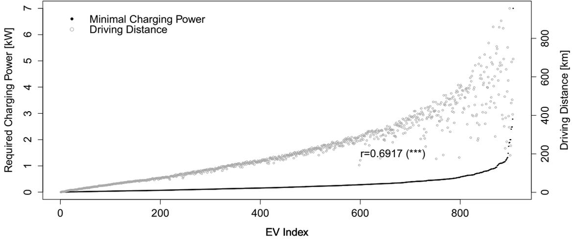
**Figure 6.11:** Charging power required for EV profile feasibility and driving distance
