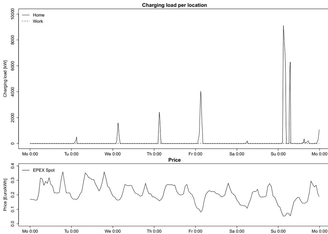
**Figure 7.5:** Aggregate Load under optimal smart charging ( $\bar{\phi} = 11kW$ ,  $SOC_0 = 100\%$ ,  $SOC_T = 90\%$ )
