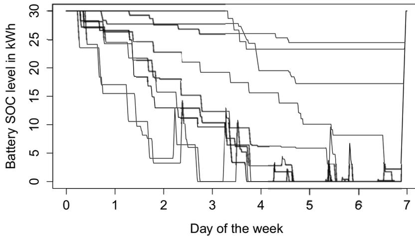
**Figure 6.13:** Battery level evolution of individual EVs under ALAP charging
