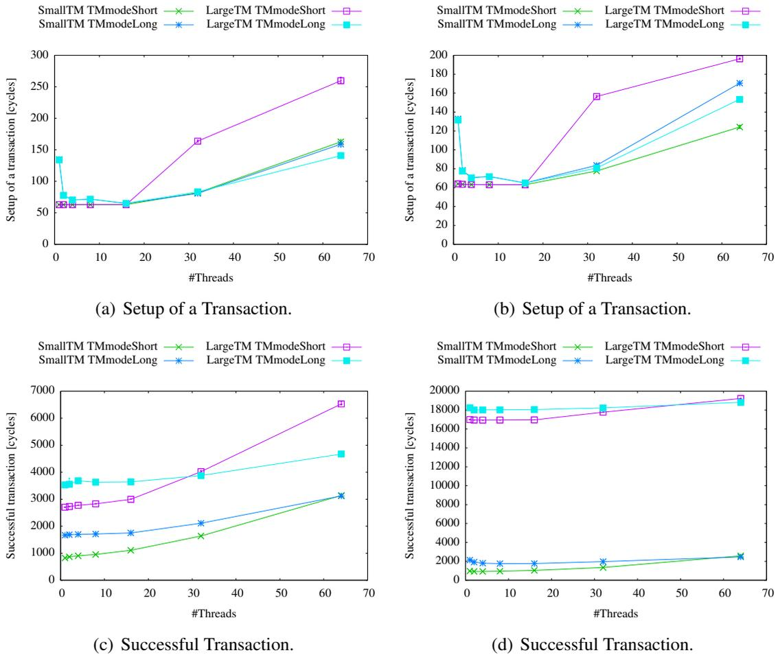
Figure 9.5: Detailed breakdown of a transaction in time for setup and execution distinguishing between execution in long-running or short-running mode across the number of threads. Left hand side run with `clomp_tm_divide1 -1 1 64 100 128 None 3 1 0 6 100` and right hand side with `clomp_tm_divide1 -1 1 256 128 256 stride1,1,stride1%/2 10 1 0 6 100`.
