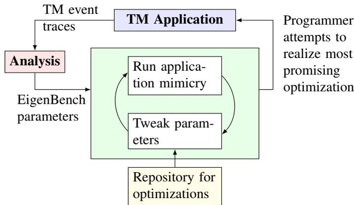
Figure 6.29: Components and interactions to illustrate the optimization workflow with *EigenOpt*.
