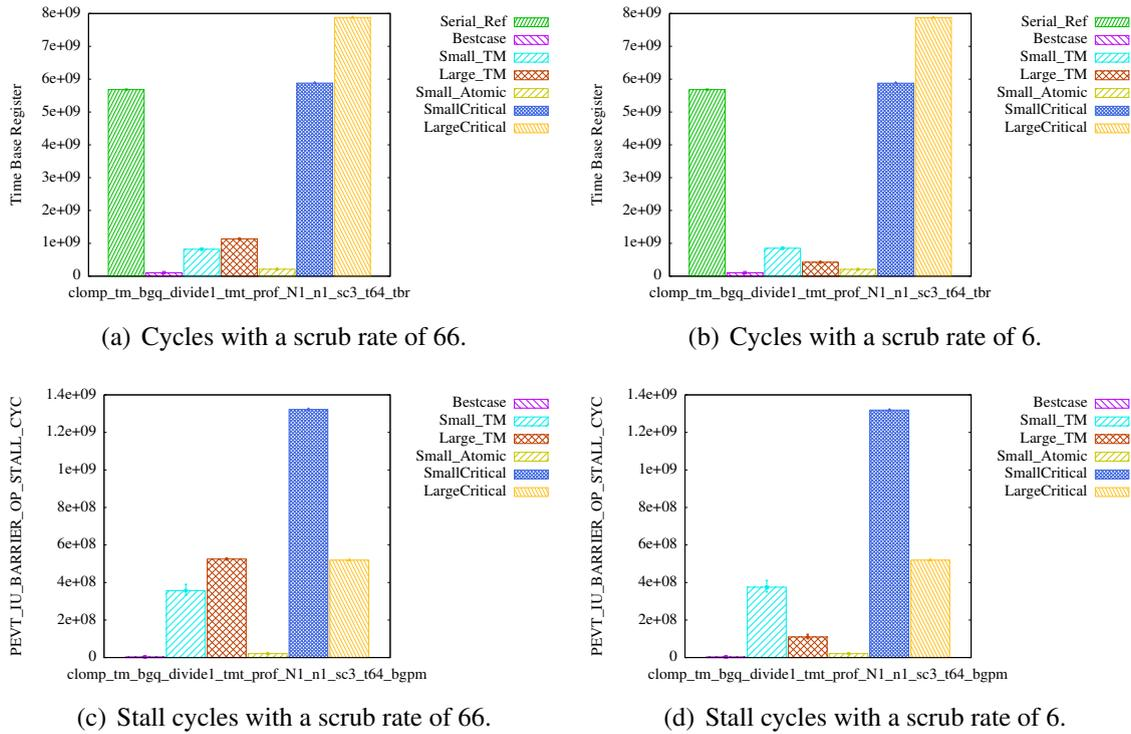
Figure 9.9: Stall cycles as an indicator for adjusting the scrub rate in the short-running mode. Run with `clomp_tm_divide1 64 1 64 100 128 None 3 1 0 sr 100`.
