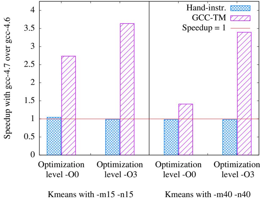
Figure 7.6: Speedup of gcc-tm-4.7 over gcc-tm-4.6 measured with `kmeans` with high (left hand side) and low contention (right hand side) to study the impact of optimizations on hand-instrumented and compiler-instrumented transactions.
