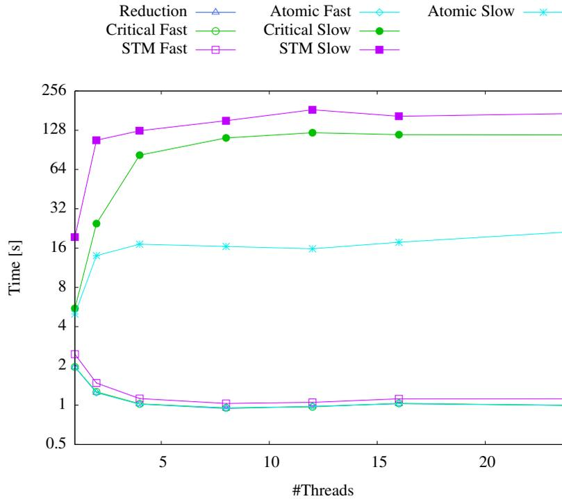
Figure 6.11: Execution time of normal CG with 1 to 24 threads on ExpX5670.
