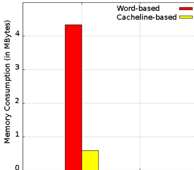
Figure 7.7: Comparing the memory consumption of a word-based (left bar) and a cache line-based (right bar) conflict detection scheme (similar to [173, 59]).
