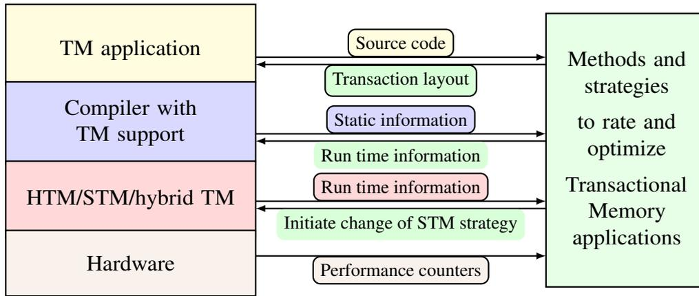
Figure 4.1: Schematic interaction of components in a system with TM software stack.
