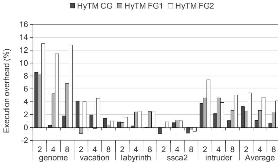
Figure 5.10: Run time overhead in % for different Hybrid TM tracing levels, core counts and applications. Each bar is an average over 20 runs – taken from [189].
