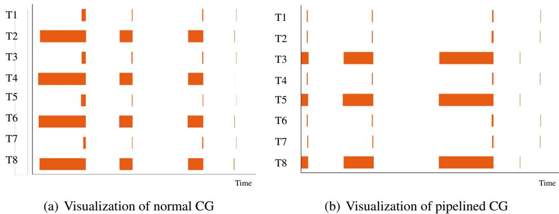
Figure 6.14: Visualization of normal and pipelined CG with 8 threads on ExpX5670. Zoomed to relate transaction time (in green) with barrier wait time (in orange). Figure similar to [176].
