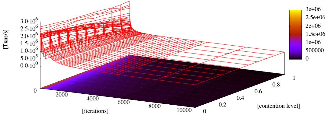
Figure 6.2: Throughput in Txns/s with PSTMA depending on the contention level and the number of loop iterations inside transactions on ExpX5670.
