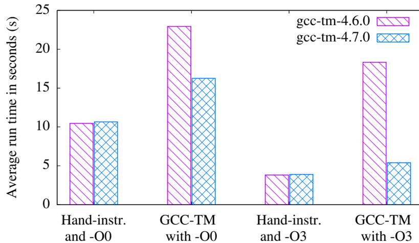
Figure 7.4: Comparison of the run times of Kmeans with low contention and hand-instrumented or compiler-instrumented transactions compiled with gcc-tm-4.6 or gcc-tm-4.7.
