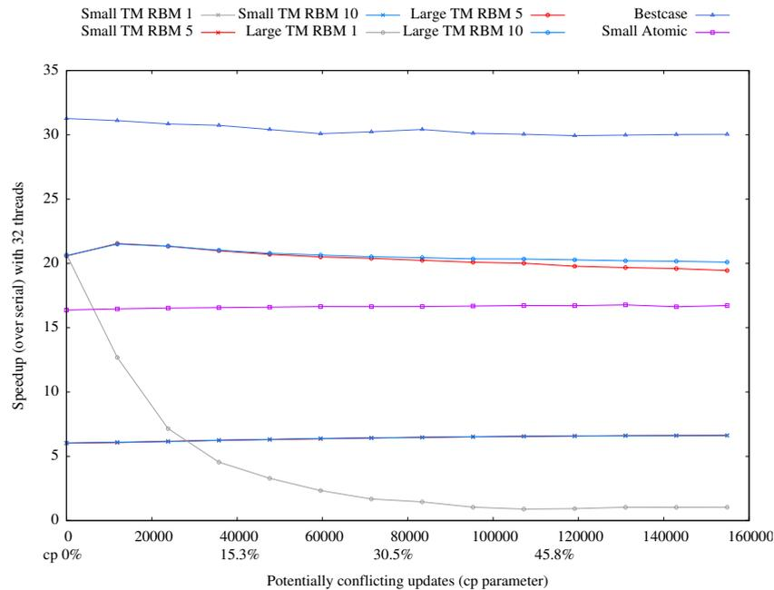
Figure 8.6: Studying the influence of setting `TM_MAX_NUM_ROLLBACK` with CLOMP-TM and changing the level of contention [171]. Run with `clomp-tm-bgq-divide4 32 1 256 128 256 stride1, cp, stride1%/2 10 1 0 6 100`.
