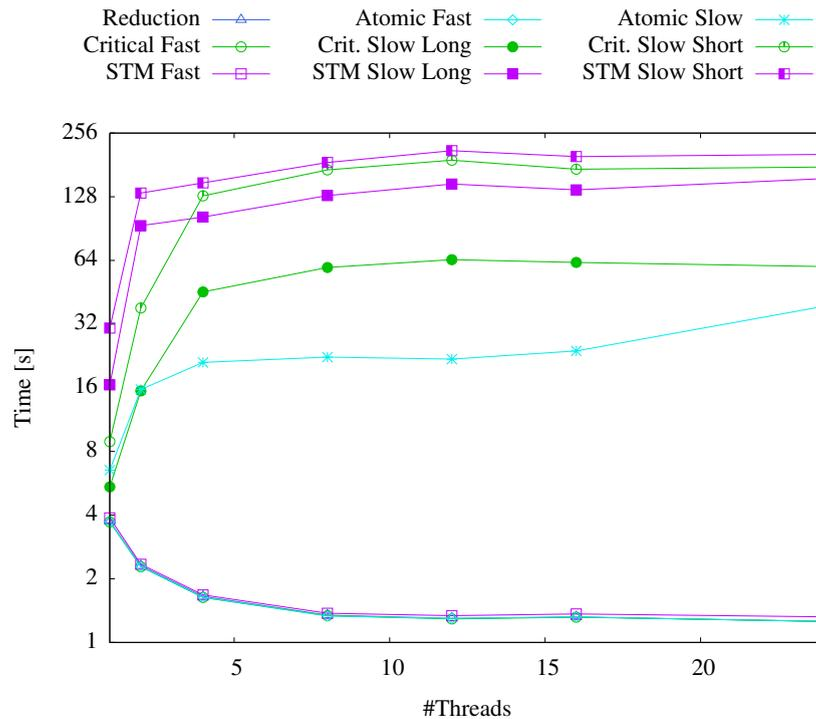
Figure 6.12: Execution time of pipelined CG with 1 to 24 threads on ExpX5670. Figure as in [176].
