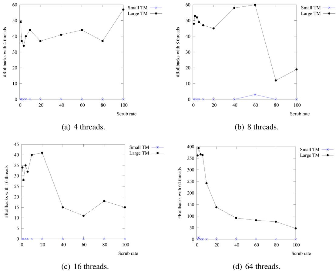
Figure 8.8: Influence of the scrub rate for SpecIds on the amount of rollbacks. Run with `clomp-tm-bgq-divide1 -1 1 64 100 128 InPart,10,firstParts 10 1 0 sr 100`
