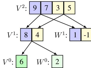
Figure 6.25: Haar wavelet transform of the digital signal [196].
