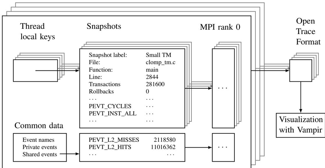
Figure 9.2: Overview of the tracing tool for TM with data structures and work flow.
