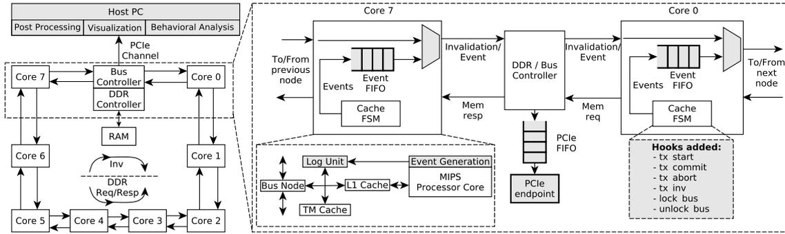
Figure 5.9: An 8-core TMbox system block diagram and modifications made to enable logging of events (shown in gray) – taken from [189].
