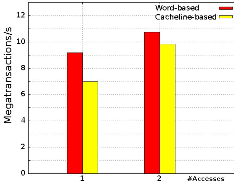
Figure 7.8: False sharing in the context of transactional memory: the throughput of a word-based (left bar) and a cache line-based (right bar) conflict detection scheme are compared (taken from [173, 59]).
