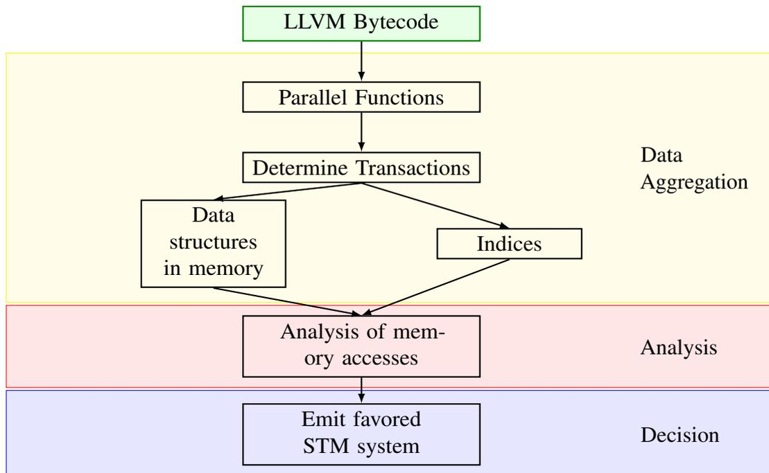
Figure 7.9: The LLVM compiler pass is divided in three logical phases: data aggregation, analysis and deciding which STM to select (cf. to [173, 59]).
