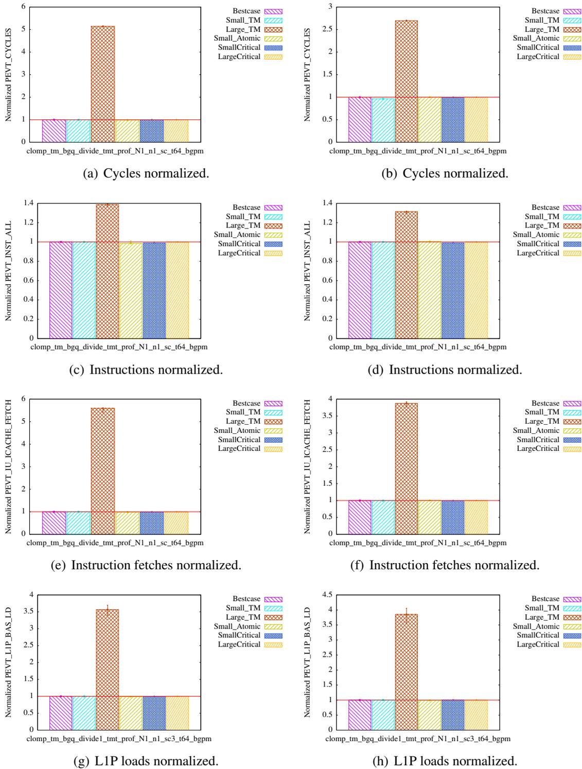
Figure 9.6: Studying the influence of setting the scrub rate from 66 to 6 on transactions in the long-running mode (left hand side) and short-running mode (right hand side). Run with `clomp_tm_divide1 -1 1 64 100 128 None 3 1 0 6 100`.
