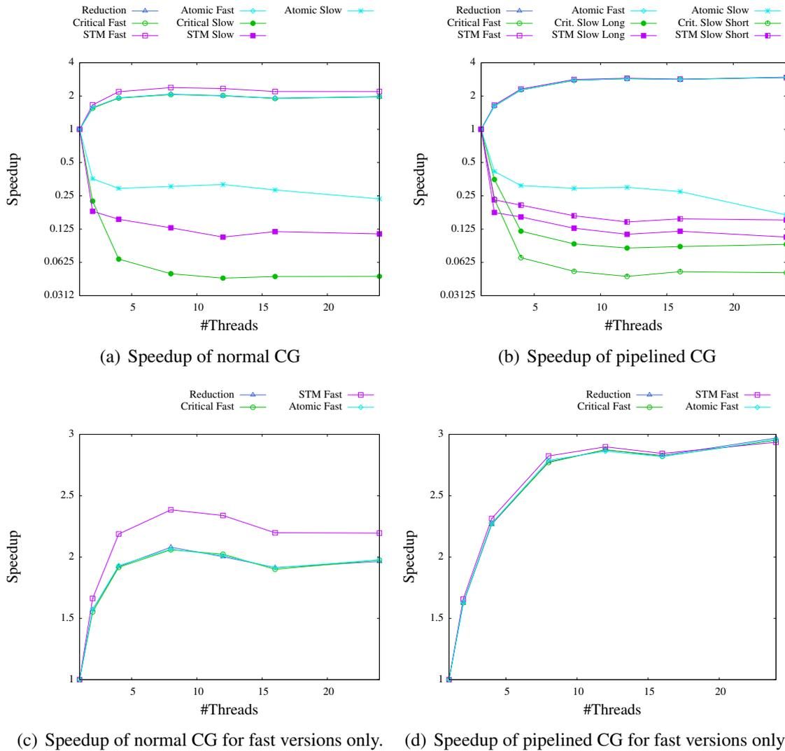
Figure 6.15: Speedup with normal and pipelined CG with the number of threads ranging from 1 to 24 on ExpX5670. Figure similar to [176].
