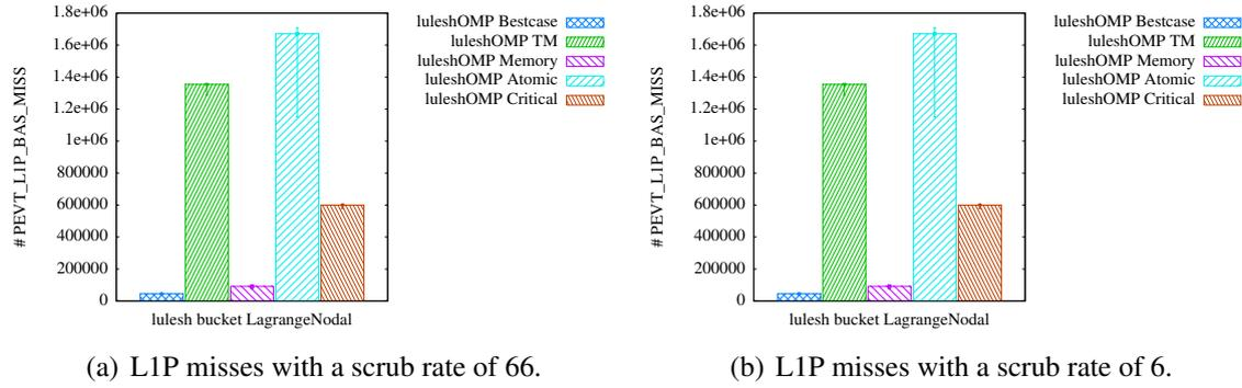
Figure 9.21: L1P misses with LULESH and 16 threads executed in long-running mode.
