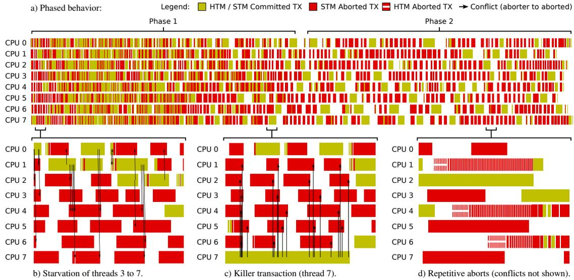
Figure 6.9: `Intruder` benchmark from the STAMP suite [24] executed on the TMbox system with 8 threads. `Intruder` exhibits two execution phases, a starvation pattern involving threads 3, 5, 6, and 7, a killer transaction executed by thread 7 and repetitive aborts. Figure is taken from [189].
