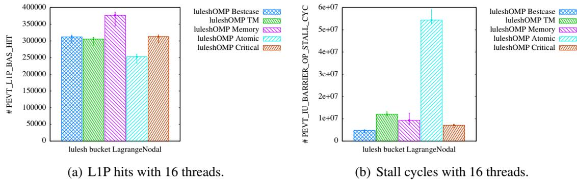
Figure 9.22: L1P hits and stall cycles with LULESH and 16 threads executed in short-running mode with a scrub rate of 6.
