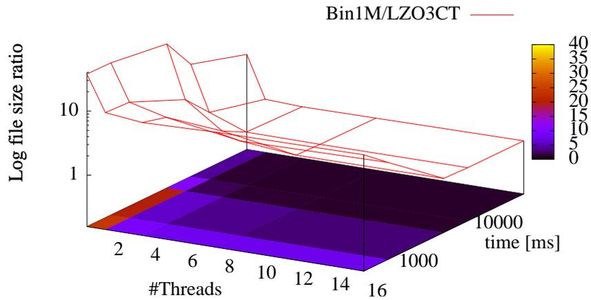
Figure 5.5: Compression factor computed as  $\frac{Size_{Bin1M}}{Size_{LZO3CT}}$  as a function of thread count and computation time (with logarithmic z scale).
