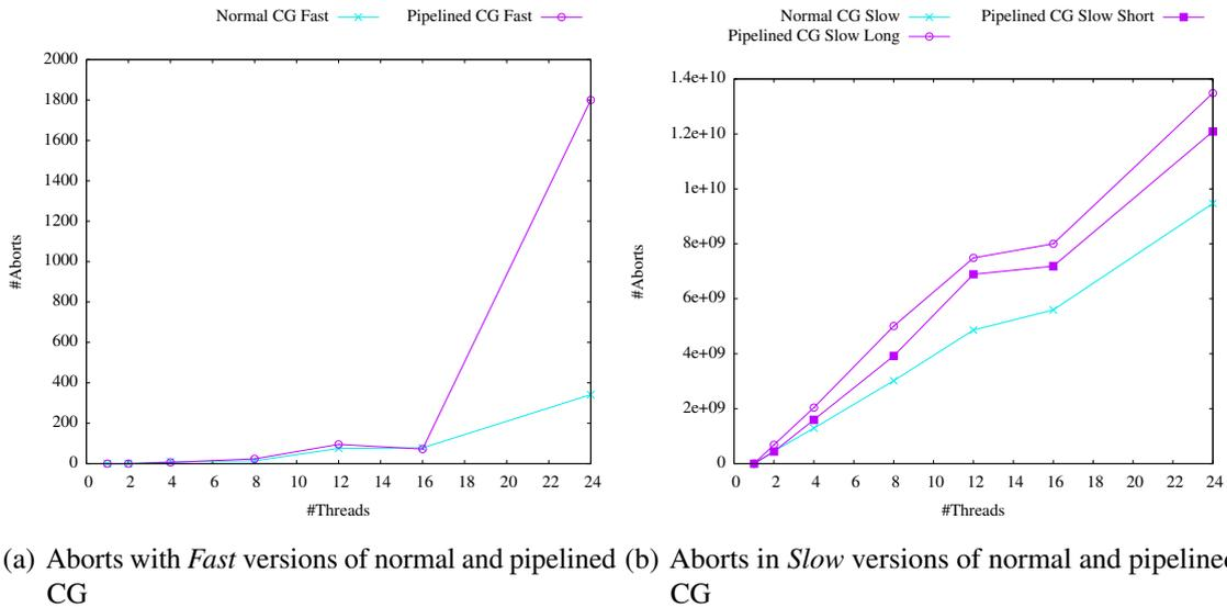
Figure 6.13: Aborts with normal and pipelined CG with the number of threads ranging from 1 to 24 on ExpX5670. Figure similar to [176].
