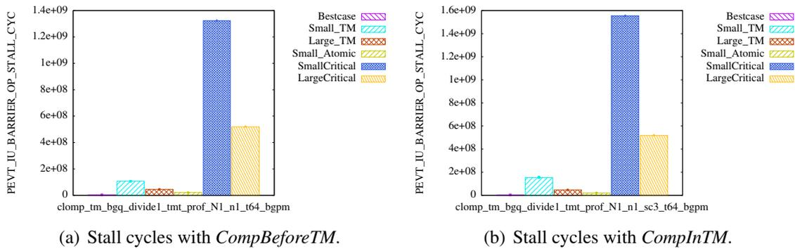
Figure 9.15: Studying the influence of setting the scrub rate on the stall cycles with the long-running mode. Run with `clomp_tm_divide1 64 1 64 100 128 None 3 1 0 6 100`.
