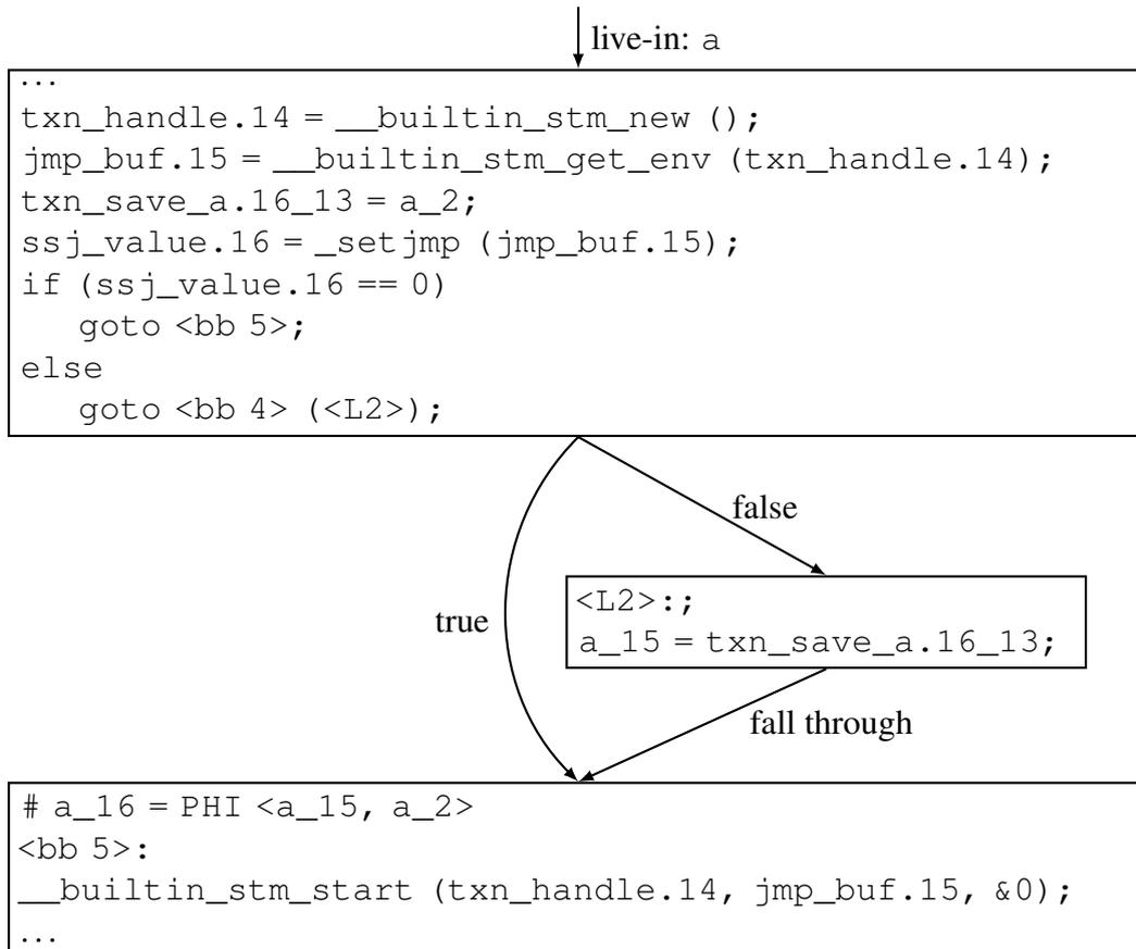
Figure 7.1: Checkpointing mechanism after the `gtm_checkpoint` pass.
