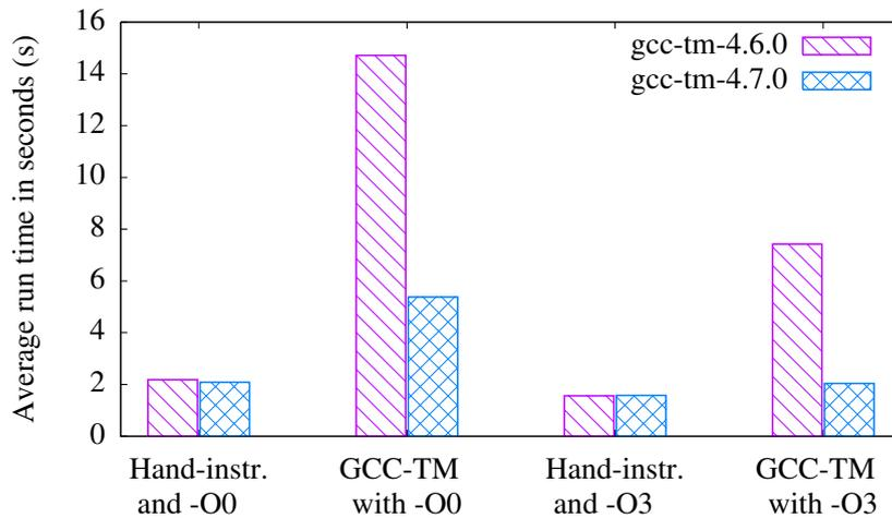
Figure 7.5: Comparison of the run times of `kmeans` with high contention with `gcc-tm-4.6` and `gcc-tm-4.7` and hand-instrumented and compiler-instrumented transactions.
