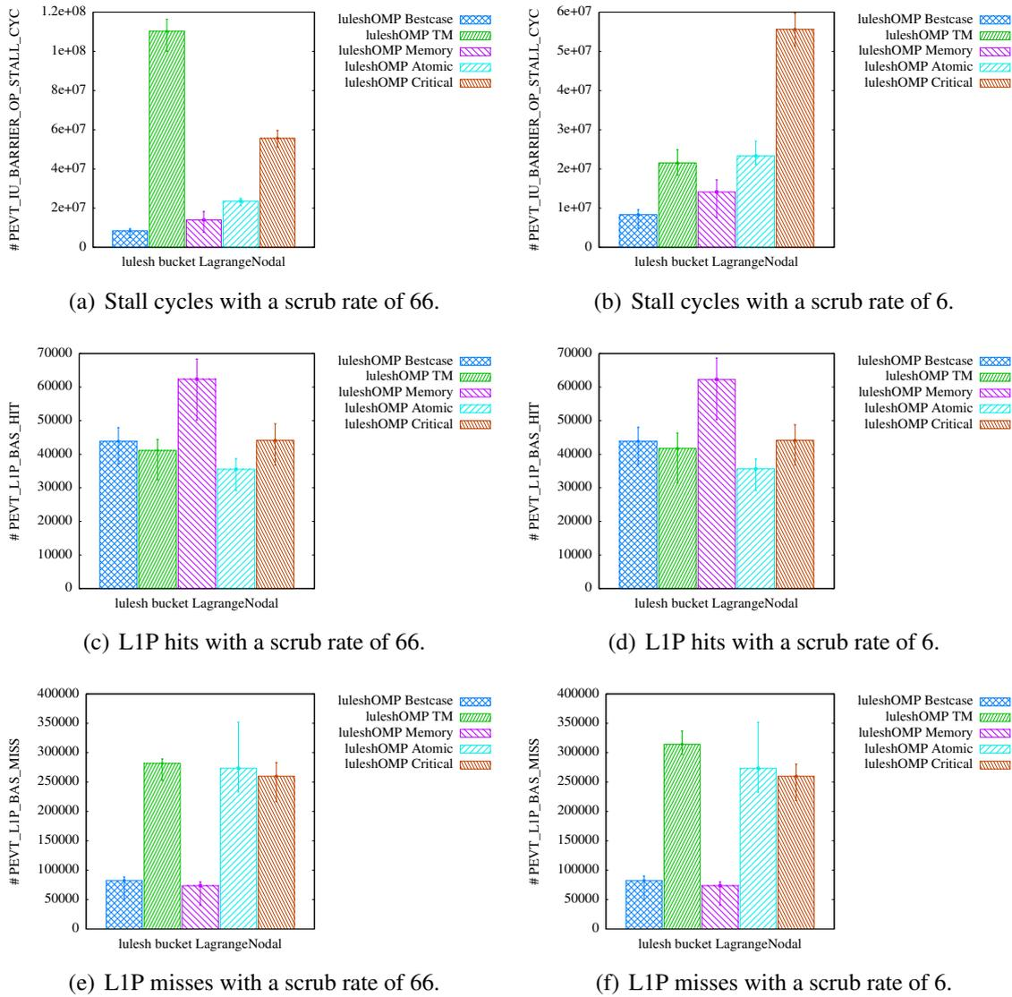
Figure 9.19: LULESH with BGPM events executed with different scrub rates and short-running TM mode.
