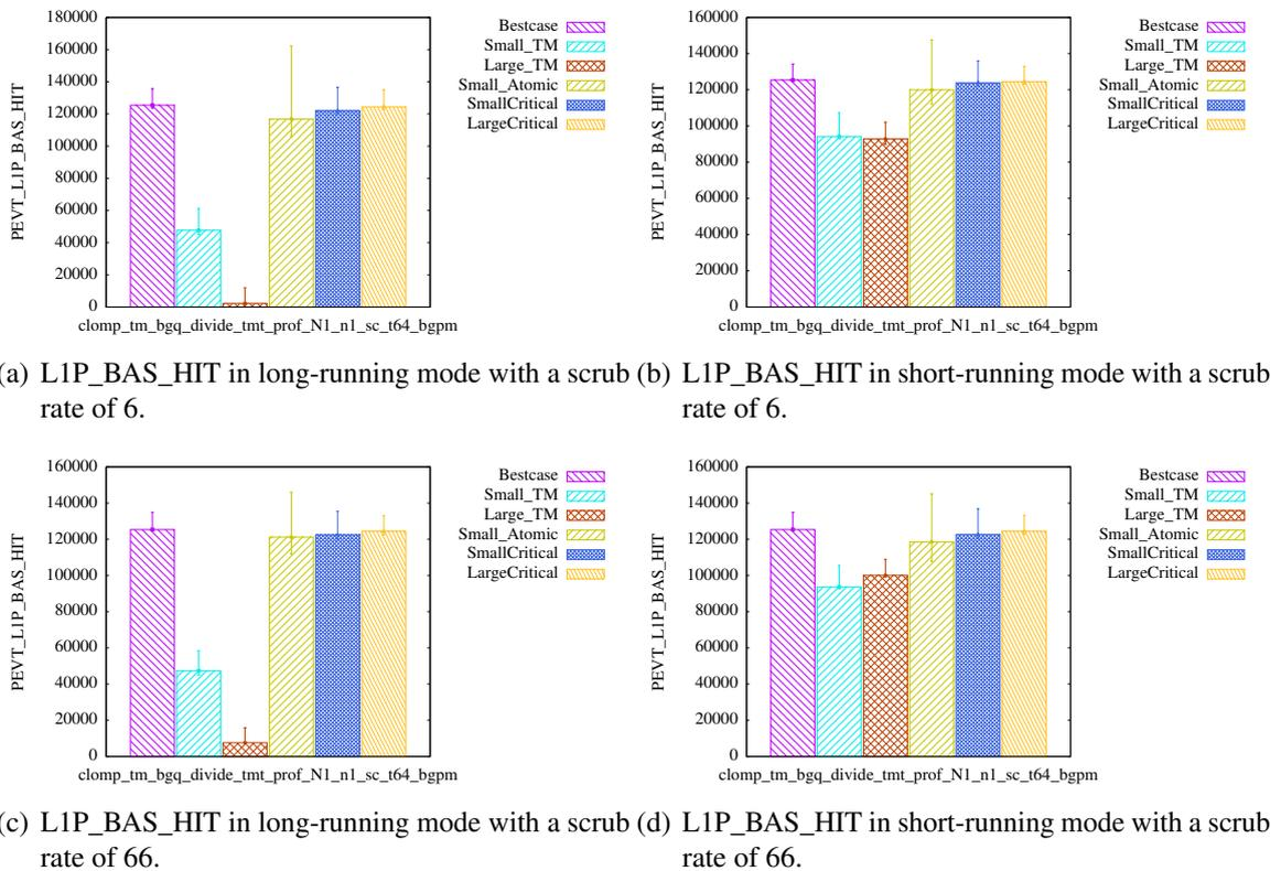
Figure 9.10: LIP utilization in the long-running and short-running mode. Run with `clomp_tm_divide1 64 1 64 100 128 None 3 1 0 6 100`.
