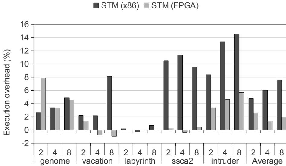
Figure 5.11: Runtime overhead in % for STM-only (x86-host) vs. STM-only (FPGA) with different core counts and applications. All bars represent averages over 20 runs – taken from [189].
