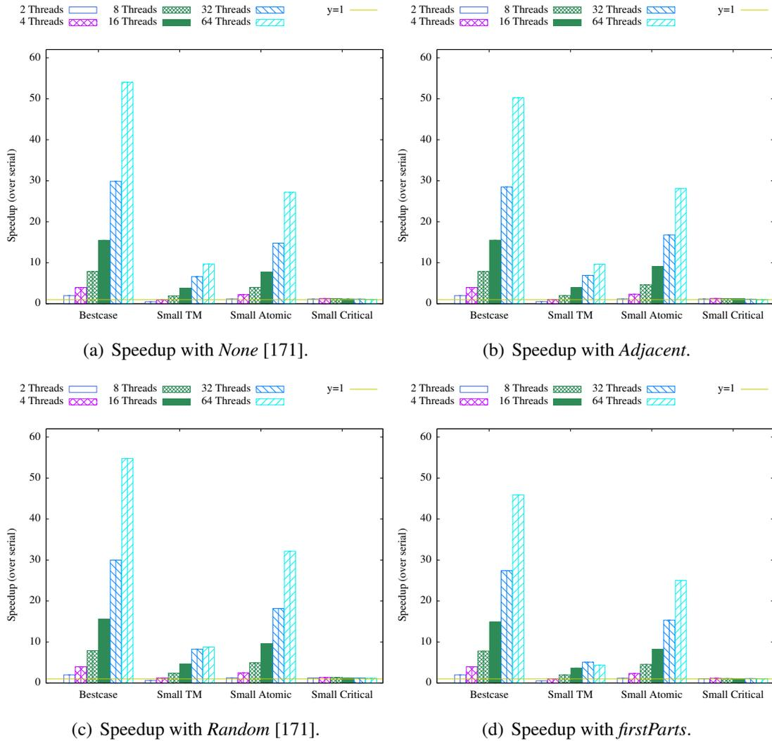
Figure 8.2: CLOMP-TM performing 8 divide operations per zone update with small critical sections [171].
