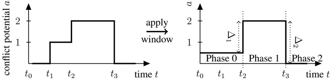
Figure 6.24: Digital Signal created from conflict potential of concurrently running transactions on the left hand side. After applying the window of fixed size, the phase detection is performed.
