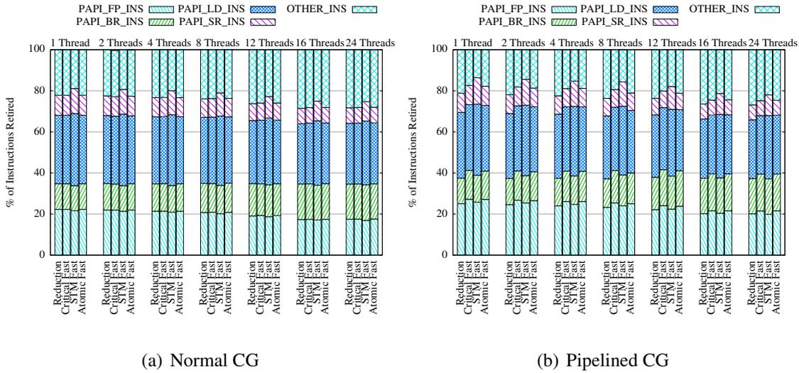
Figure 6.21: Breaking down the total amount of instructions in CG on ExpX5670. Figure similar to [176].
