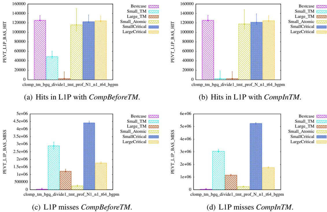
Figure 9.14: Studying the influence of moving the computation inside the transaction in the long-running mode. Run with `clomp_tm_divide1 -1 1 64 100 128 None 3 1 0 6 100`.
