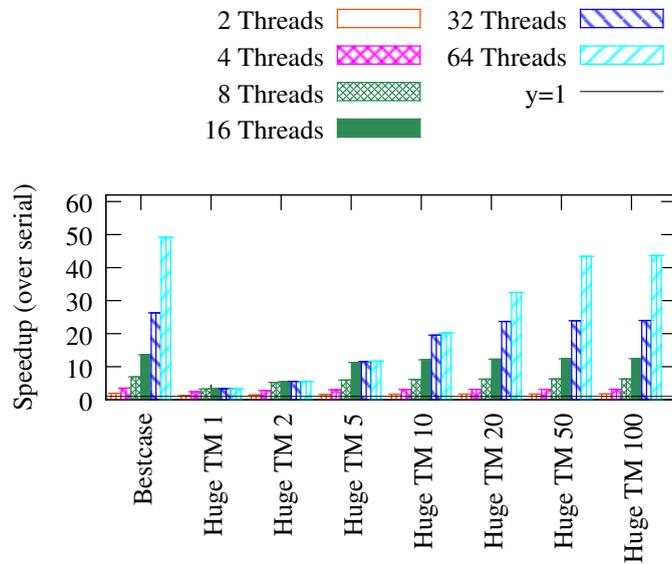
Figure 8.4: CLOMP-TM (v. 1.36) performing 8 divide operations per zone update with huge critical sections. Speedup shown with *None* [171].
