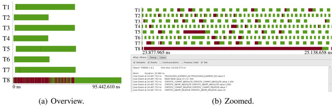
Figure 6.6: Paraver visualizing the StarvingElder pattern generated with the EigenBench microbenchmark.
