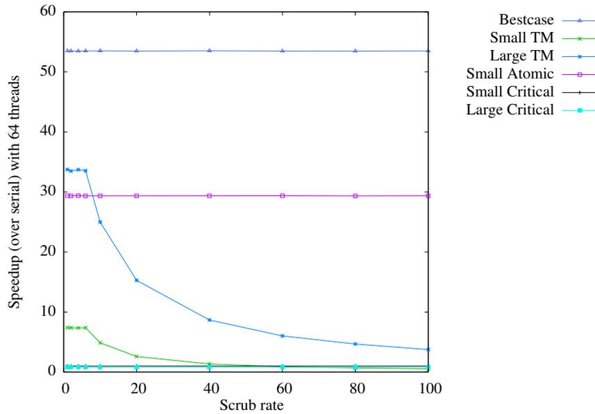
Figure 8.7: Influence of the scrub rate for SpecIds on performance with 64 threads [171]. Run with `clomp-tm-bgq-divide1 -1 1 64 100 128 InPart,10,firstParts 10 1 0 sr 100`
