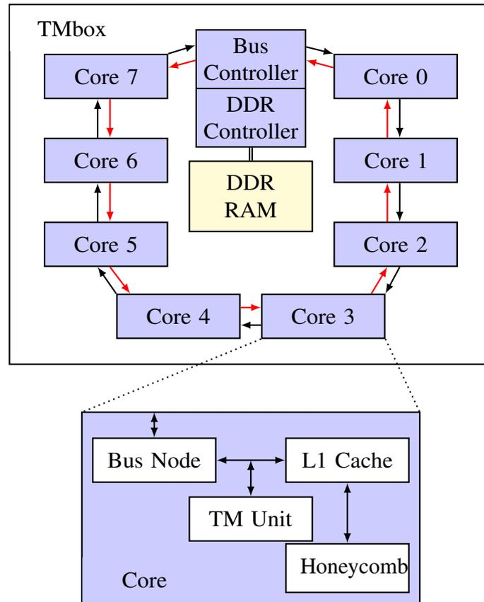
Figure 5.8: Overview of the TMbox system, showing a bi-directional ring bus that connects 8 cores and a bus controller (similar to [190]).
