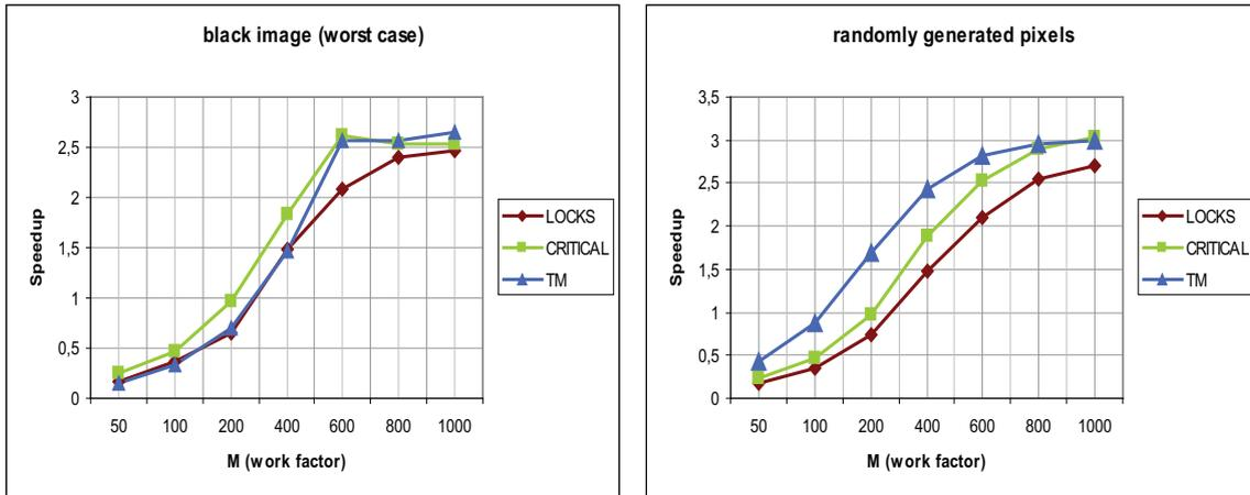
Figure 7.2: Speedup over sequential execution using locks, OpenMP critical sections, and transactions; first published in [172].
