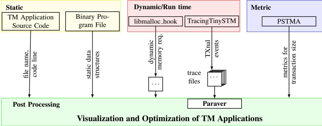
Figure 6.1: Components and interplay in the TM Visualization and Optimization framework.
