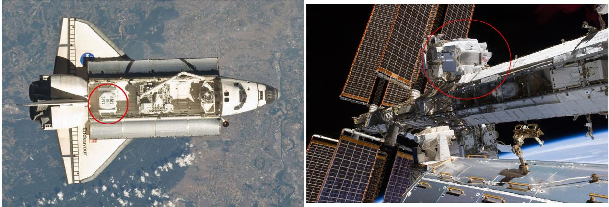
Figure 3.3.: *AMS-02 in space*. Left: AMS-02 in the cargo bay of Space Shuttle Endeavour on the way to the ISS, right: AMS-02 installed in its final location on the ISS. credit: NASA [121]
