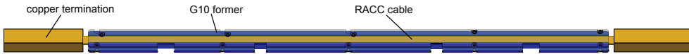
Figure 4.11: Schematic drawing of a G10 jacket for the impregnation of a 15x5 RACC cable from IRL (shown in dark yellow). The jacket consists of two parts, a U-shaped former (shown in blue) and T-shaped cap (shown in transparent gray).
