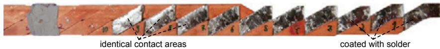
Figure 5.23: Second step in assembling a stair shaped contact for RACC cables. The contact areas of the tapes of the RACC cable have to be coated with solder.
