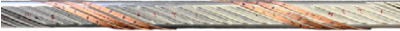
Figure 6.14: Sub-size CCRC consisting of 3 RACC subcables with a width of 4 mm. Picture from [Kar12].
