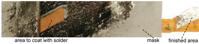
Figure 5.20: Mask made of paper to coat a well defined area of a REBCO tape with solder.
