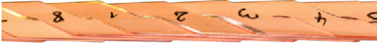
Figure 5.4: Roebel Assembled Coated Conductor (RACC) cable consisting of 10 strands. Picture from A. Kario.
