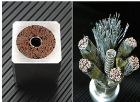
Figure 3.5: Cable in conduit conductors of the ITER magnet system: central solenoid and poloidal field coil conductor (left), toroidal field coil conductor (right). Pictures from [ENE].
