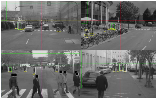
Figure 6.7 Examples for challenging tracking scenarios: Only some pedestrians are detected by the camera in crowded scenes. Pedestrian groups are tracked as one pedestrian if the single pedestrians occlude each other. The foot point of a pedestrian has to be within the image to enable a detection by the camera. Partial occlusion of pedestrians often hinders stable detection and tracking.
