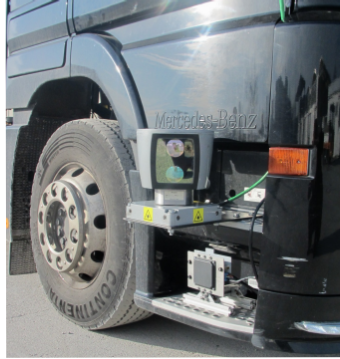
Figure 4.5 Mounting positions of blind spot radar and laser scanner at right vehicle side.
