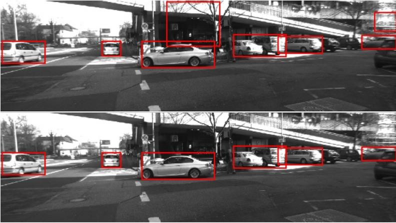
Figure 5.10.: **Improving Object Detection.** By using context from our model for re-weighting object hypothesis our algorithm (bottom) is able to eliminate false positives of state-of-the-art part-based object detectors [60] (top).
