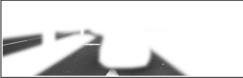
Figure 1.1.: **Intersection from a Lane Detector's Point of View.** This figure shows a typical traffic scene with all non-road pixels masked. Note how difficult it is to correctly assess the intersection geometry using this information alone. To see the full picture, please turn over to Fig. 1.2 on page 4.
