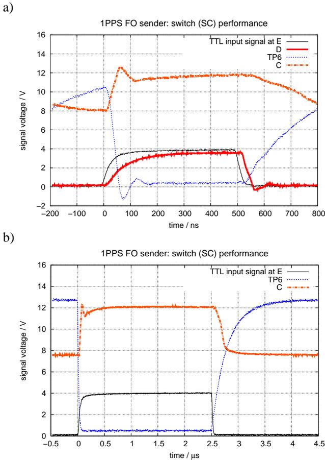
**Figure 5:** 1 PPS distributor: Switching circuit (SC) performance on two different time scales. black: TTL input signal (E). thick red: signal at switching circuit input (D). dotted blue: signal at collector of switching transistor T2 (TP6). thick dotted orange: signal at output of switch (C), i.e. collector of switching transistor T3.
