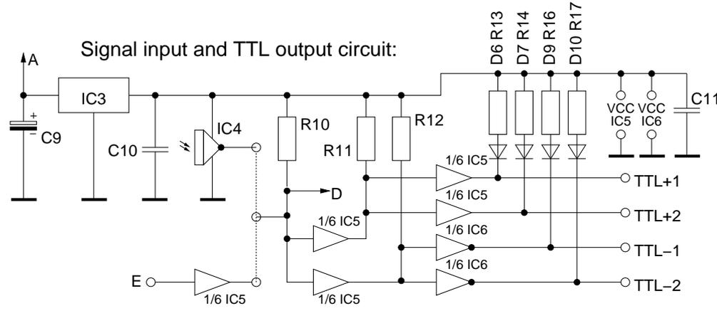
**Figure 9:** 1 PPS distributor: Circuit schematics.
