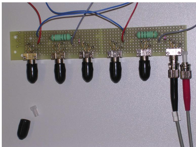
**Figure 12:** 1 PPS distributor: Prototype FO diode board.
