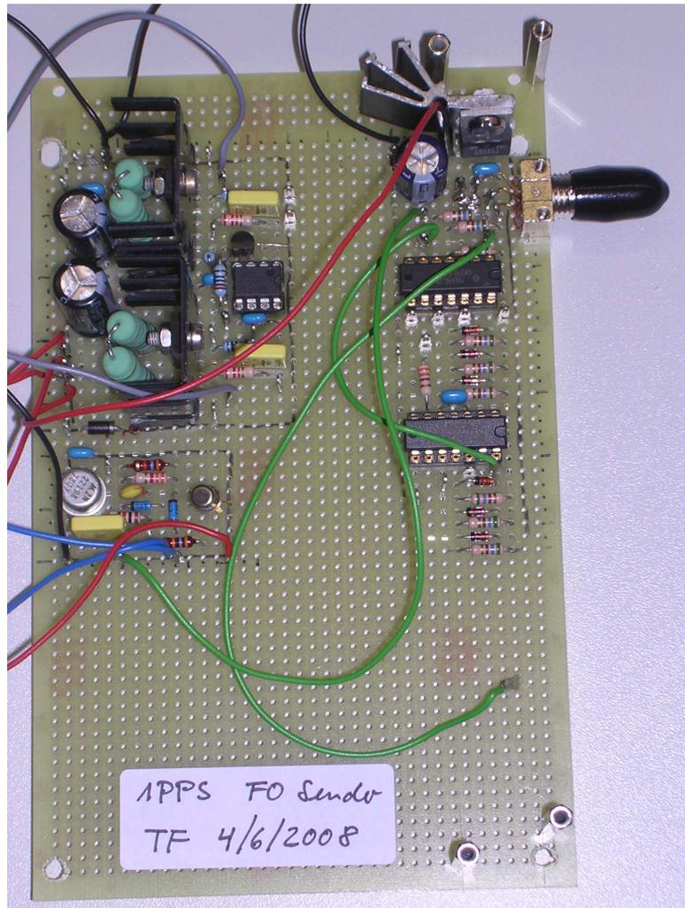
**Figure 11:** 1 PPS distributor: Prototype board.
