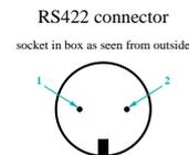
**Figure 2:** 1 PPS signal connector socket in fixed cabinet on vault's wall. Pin location is displayed as seen from outside the housing. The socket is a female Buccaneer 400 PX0412/02S.
