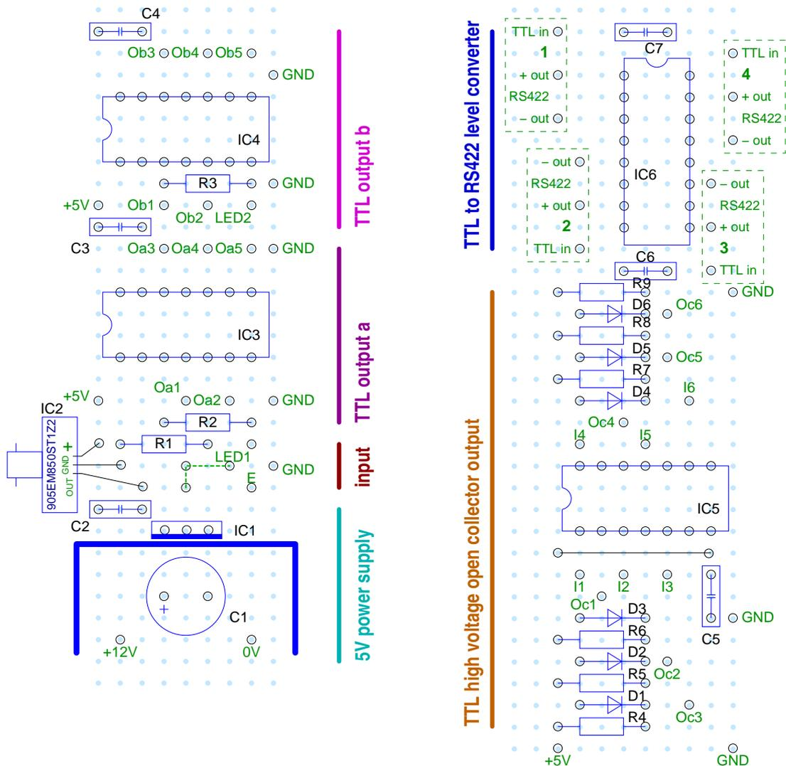
Figure 25: 1 PPS multifunctional receiver with RS-422 output: Board layout parts placement.
