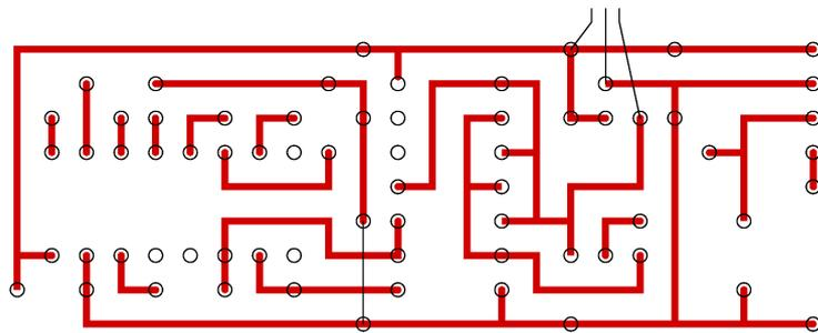
**Figure 18:** 1 PPS FO receiver: Board layout wiring diagram.
