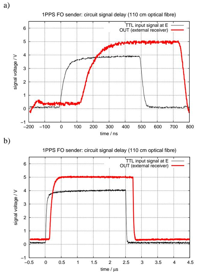
**Figure 4:** 1 PPS distributor: Signal propagation performance. Propagation of TTL input signal (E, black) to the output of an external receiver (thick red) on two different time scales.
