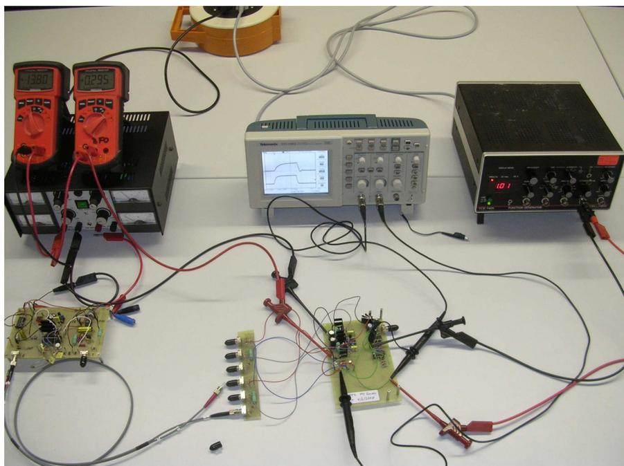
Figure 14: 1 PPS distributor: Performace test setup.
