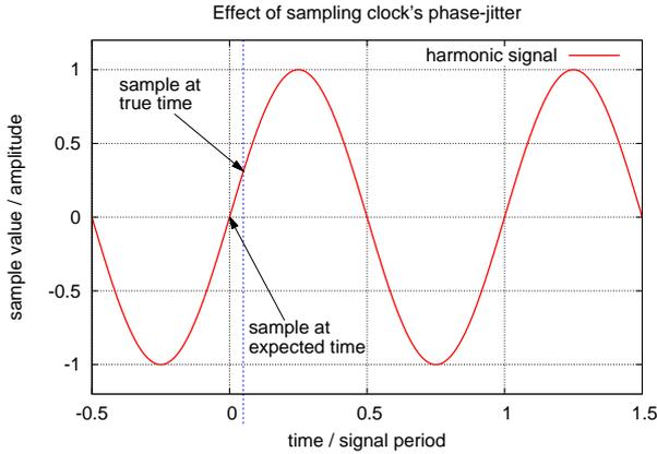
**Figure 1:** Jitter noise is a result from unstable sampling time.
