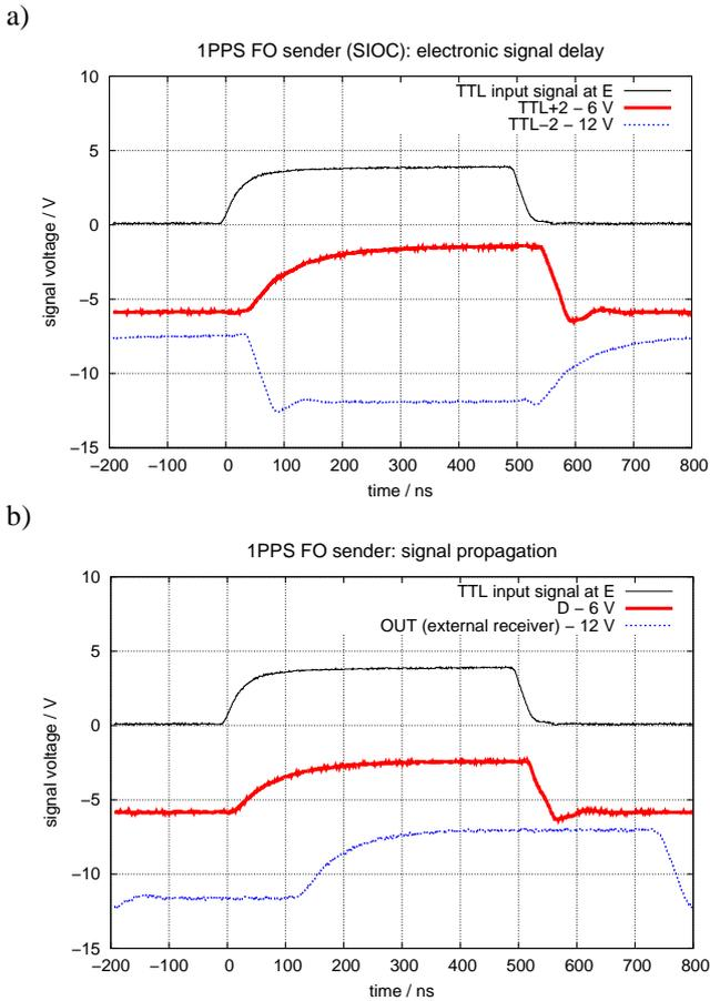
**Figure 3:** 1 PPS distributor: Internal signal propagation performance. a) Propagation of electric input signal (E, black) to positive (TTL+2, thick red) and inverted (TTL-2, blue dotted) electric TTL signal outputs. b) Propagation of TTL input signal (E, black) to switching circuit input (D, thick red) and to the output of an external receiver (blue dotted). Signals are offset intentionally for better visibility (see graph legend).
