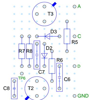
Signal input and TTL output circuit (SIOC):
