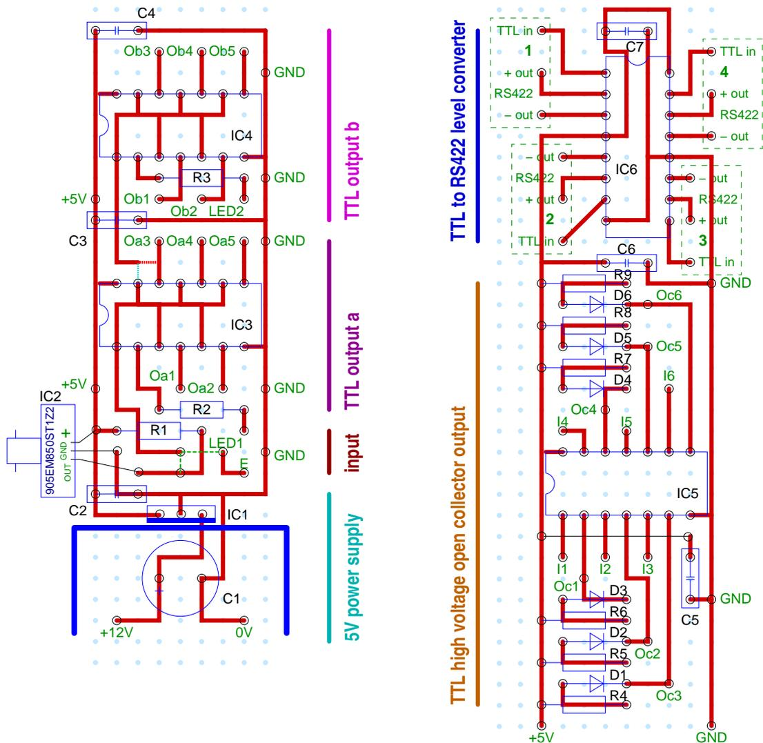
Figure 23: 1 PPS multifunctional receiver with RS-422 output: Board layout.
