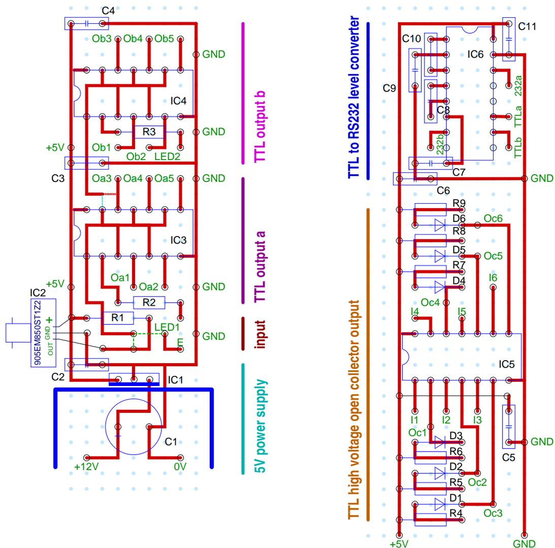
Figure 20: 1 PPS multifunctional receiver with RS-232 output: Board layout.
