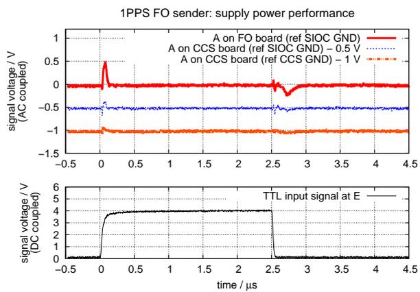
**Figure 7:** 1 PPS distributor: Supply voltage performance. The supply power (A) is recorded at different locations AC coupled. thick red: FO board with reference to GND on SIOC board. dotted blue: CCS board with reference to GND on SIOC board. thick dotted orange: CCS board with reference to GND on CCS board. The signals are offset intentionally for better visibility (see graph legend). In the lower panel the TTL input signal (E) is displayed for timing reference.
