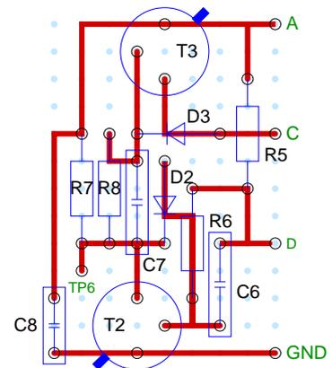
Signal input and TTL output circuit (SIOC):
