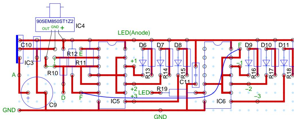
Figure 10: 1 PPS distributor: Board layout.
