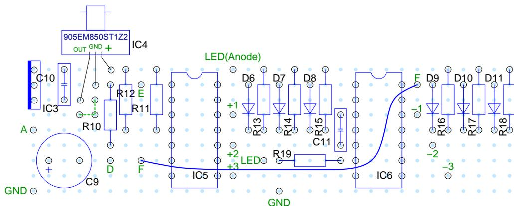
Figure 16: 1 PPS distributor: Board layout parts placement.
