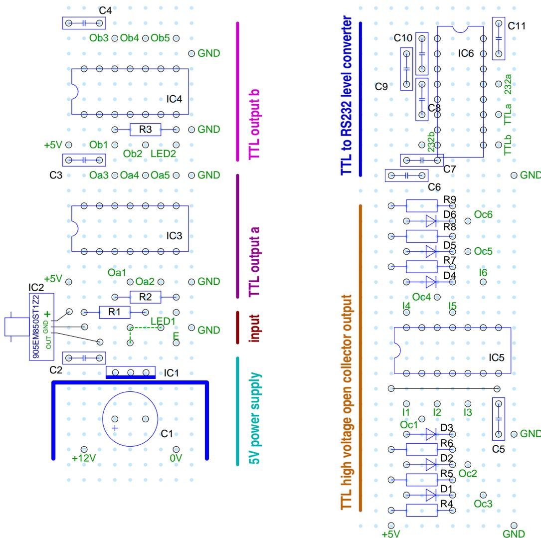
Figure 22: 1 PPS multifunctional receiver with RS-232 output: Board layout parts placement.
