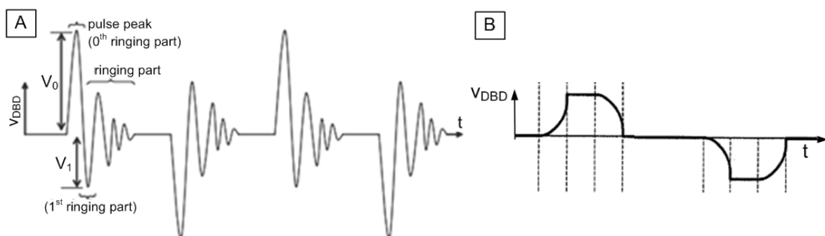
Figure 28: A: alternating bipolar pulse and determination of positive ( V_0 ) and negative ( V_1 ) voltage peak; chart basing on (Somekawa 2005), B: distributed bipolar pulse according to Park (2008). Pictures modified for clarity.
