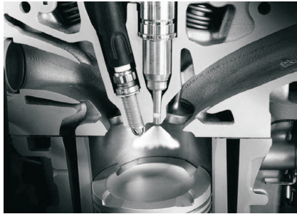
Figure 2.4: Second generation of direct injection engines with stratified mode: spray-guided concept [53]
