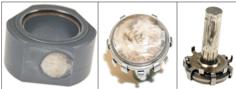
Figure 7.42: Pictures of a Bosch CP1 cam (left), pusher (middle) and piston (right) after investigation (sliding distance: 5,600 m)
