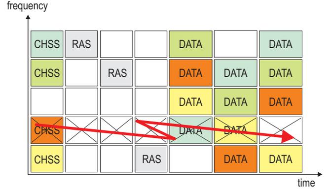
Fig. 2. Frequency hopping scheme with one interfered channel
