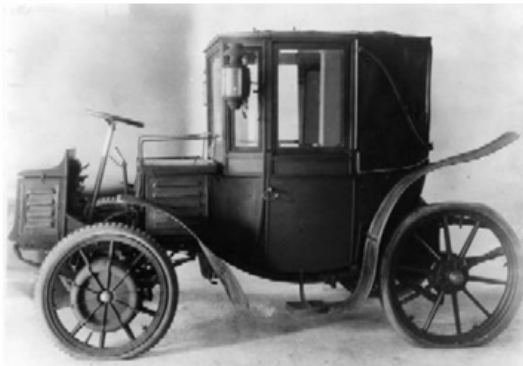
Figure I.85: The "Sailing Ship Effect" illustrated for a "hybrid car" combining a combustion engine and an electro-motor (Source: Hybrid-vehicle.org).
