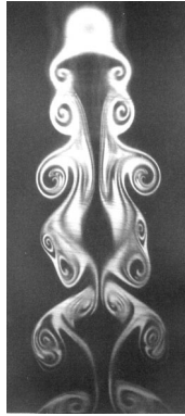
Figure 3.8: LIF visualization obtained by placing the laser sheet parallel and very close to the wall ( x/D = 0.2 , R = 2 ). Reproduced from [14].
