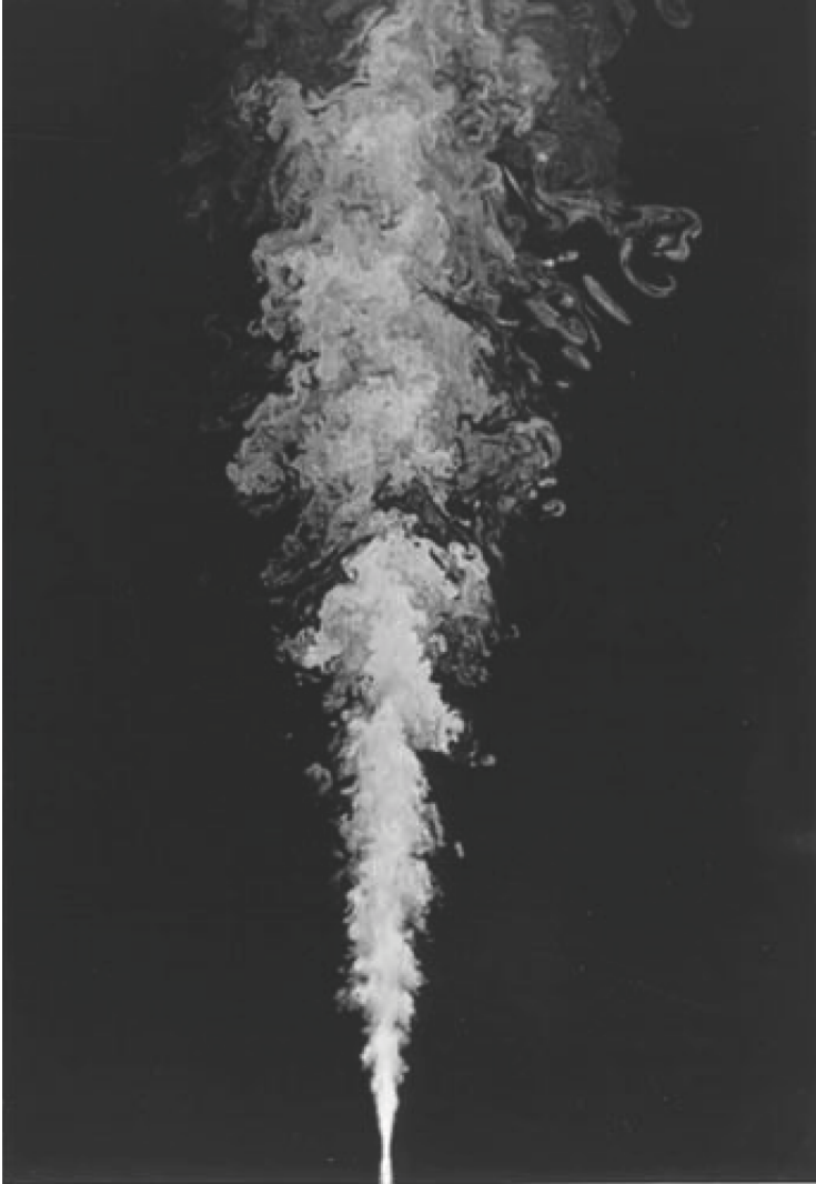
Figure 4.1: Liquid-phase turbulent jet symmetry plane slice. Gray scale codes jet-fluid mole fraction. Reynolds number approximately 10^4 . Reproduced from [23].
