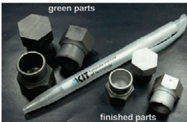
Fig. 3: Finished two-component mockups: green parts (left) and after heat-treatment (right).
