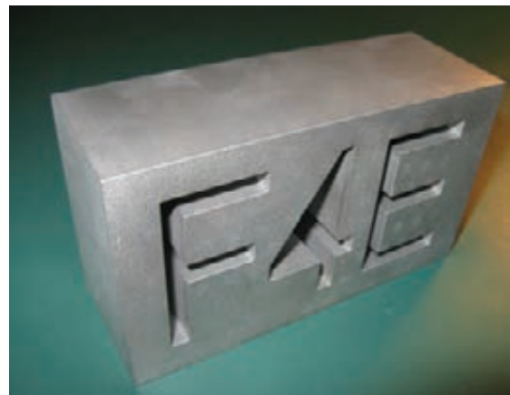
Fig. 4: Precision water cut of >F4E< Logo with 50mm P92 heat-resisting steel material.
