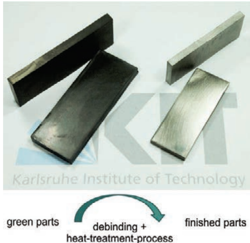
Fig. 1: Finished plates: green parts (left) and after heat-treatment (right). The shrinkage is nearly 20%.
