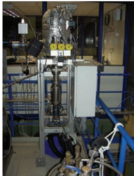
Fig. 2: Experimental set-up of a diffusion pump for proof-of-principle testing. The small dosing dome with the mass flow controller can be seen on top; the liquid nitrogen baffle and the diffusion pump are located below.
