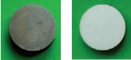
Fig. 4: Macroscopic view of cleaned tungsten disc (left) and Pd coated piece (right).
