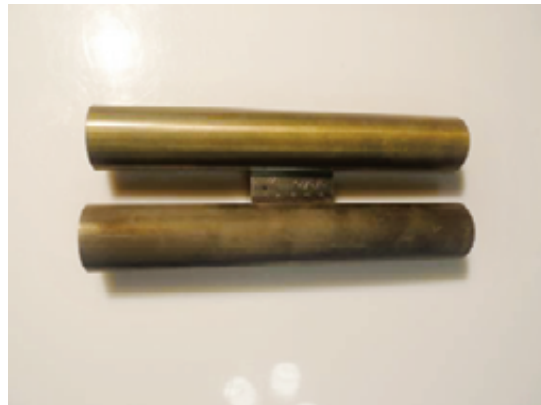
Fig. 3: SMST (top) surface is not that dark as POSCO (bottom) surface after heat treatment 2.
