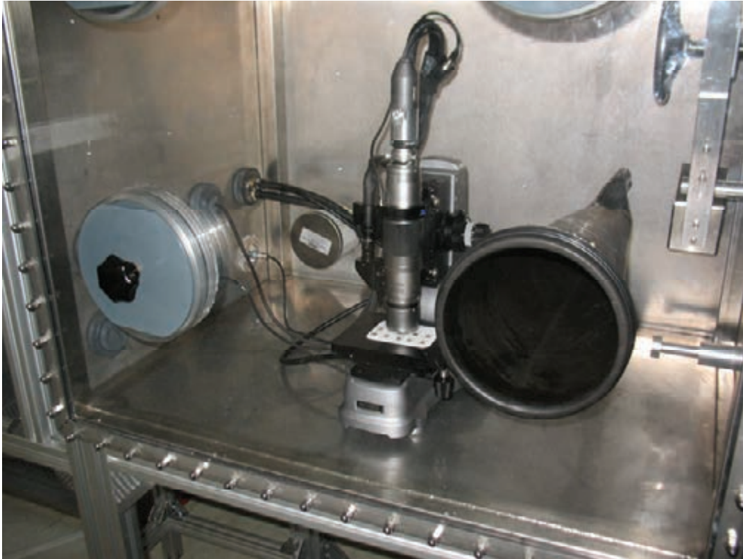
Fig. 2: KEYENCE digital microscope inside of a new-built glove-box.
