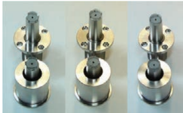
Fig. 6: Broken captive bolts V1-V2-V3.
