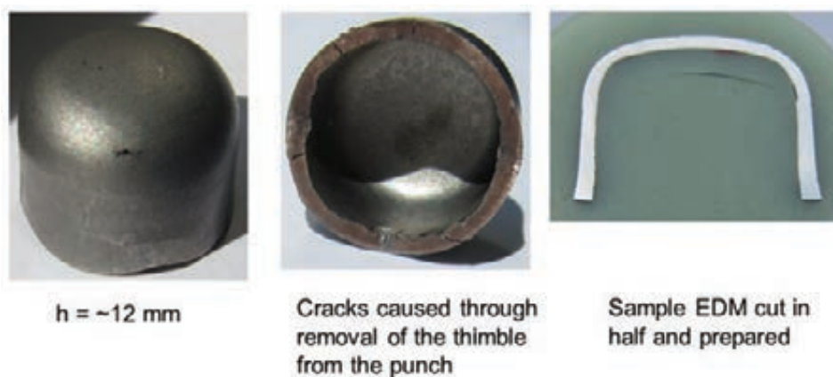
Fig. 2: Deep-drawn thimble from \varnothing 28 mm initial W slice with new flat tool.
