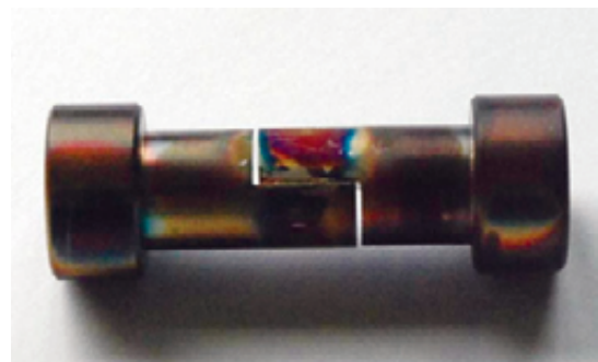
Fig. 3: Joint steel sample for shear testing with a central brazing zone of roughly 12 \times 12\ \text{mm}^2 .
