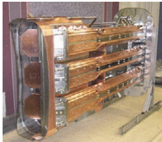
ECRH-plug-in launcher with adjustable copper mirrors (left) supporting 3 beams.
