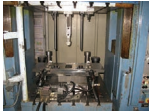
Fig. 2: Running process of HCPB TBM Cooling Plate MU with 30 cooling channels (length 300mm).
