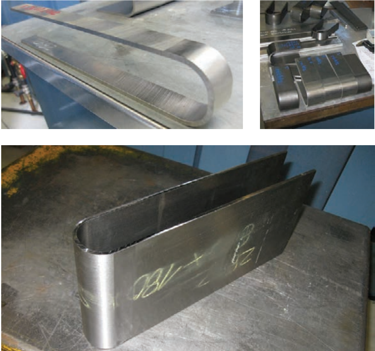
Fig. 5: Several HCPB TBM Cooling Plate bending experiments (until real scaled MU below).
