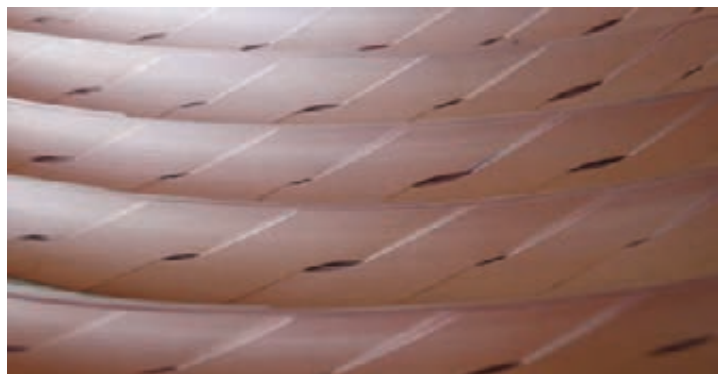
Fig. 6: Roebel cable with 4.5 m length and 12 mm width, consisting of 10 strands.
