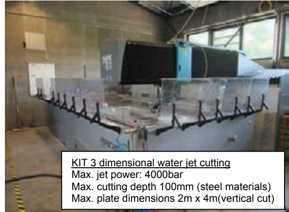
Fig. 2: KIT water jet cutting machine (installed August 2012).
