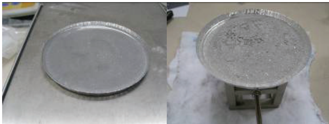
Fig. 2: Coarse Al dust after wet milling in ethanol during 1 hour. Final fineness is about 20 \mu\text{m} .
