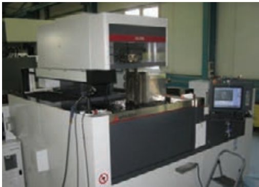
Fig. 2: Running process of HCPB TBM Cooling Plate MU with 30 cooling channels (length 300mm).
