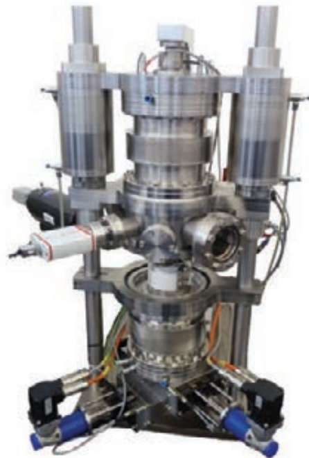
Fig. 5: Indentation device for indentation up to 200 N / 650 °C.
