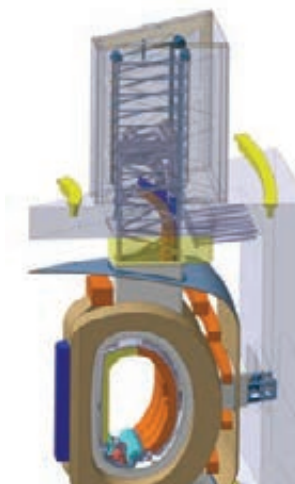
Vertical transportation cask settled on upper port extracting one OB-MMS
