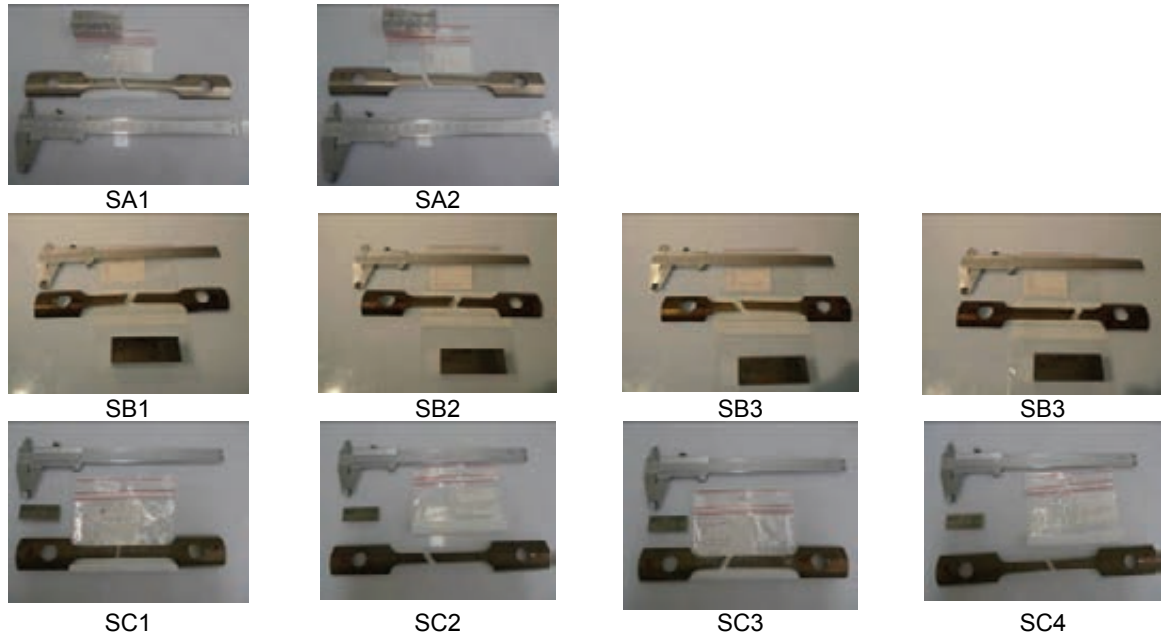
Fig. 4: Tested SMST TF jacket specimen according to Table 1.
