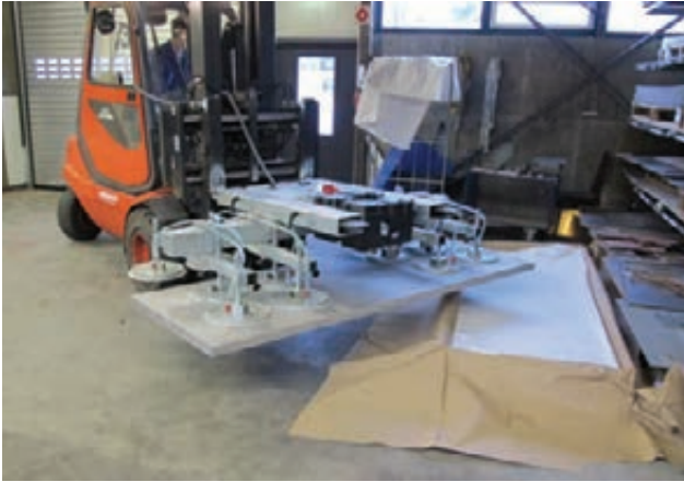
Fig. 1: Vacuum lifter gripping of 50mm plate EUROFER.
