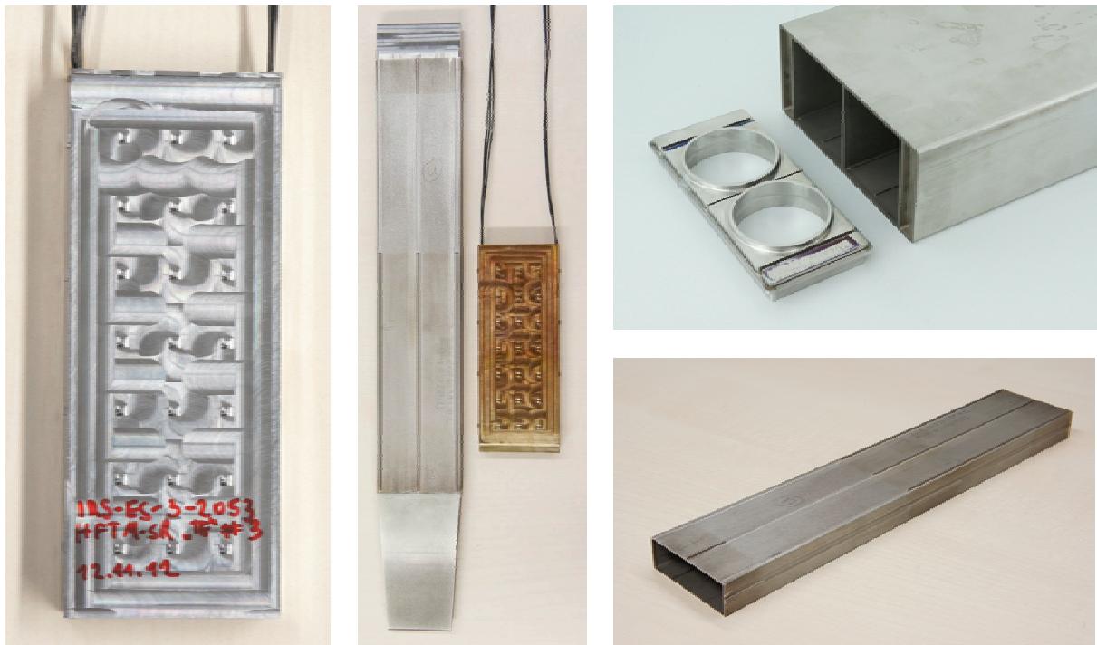
Fig. 2: Capsules with knop pattern, completed rig and HFTM container.
