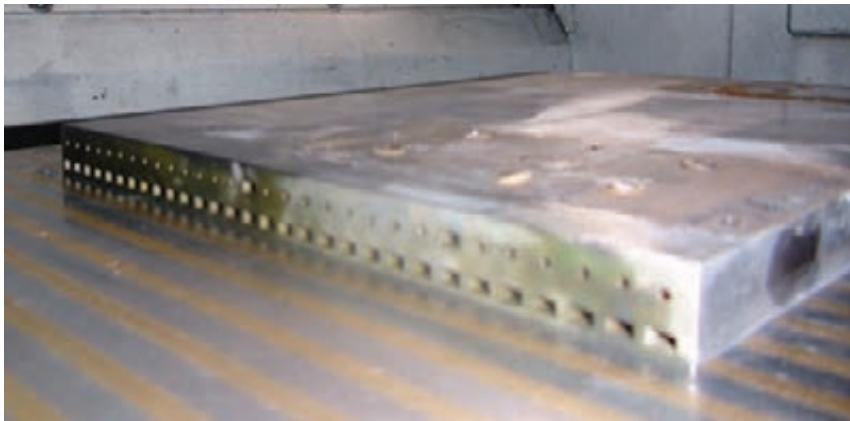
Fig. 2: Running process of HCPB TBM Cooling Plate MU with 30 cooling channels (length 300mm).
