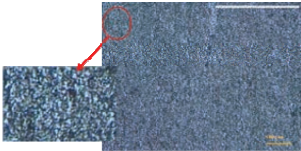
Fig. 7: W foil etched in solution of K_3[Fe(CN)_6] * KOH for 3 min.
