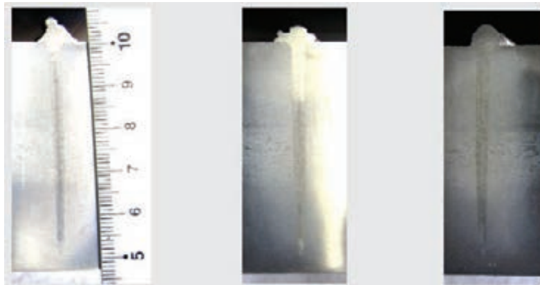
Fig. 8: EB test welds for the BSM prototype.
