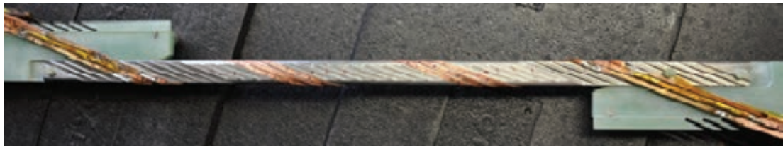
Fig. 9: CCRC demonstrator cable with 3 ROEBEL strands
