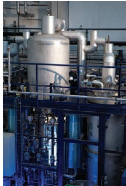
Fig. 1: He-purifier with a continuous purification rate of 14 g/s at 200 bar.
