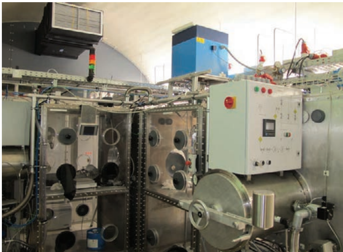
Fig. 1: Glove-box system consisting of three sections (electrical sintering oven is on the top of this system).
