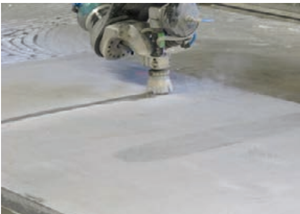
Fig. 3: Cut of 50mm EUROFER steel plate.
