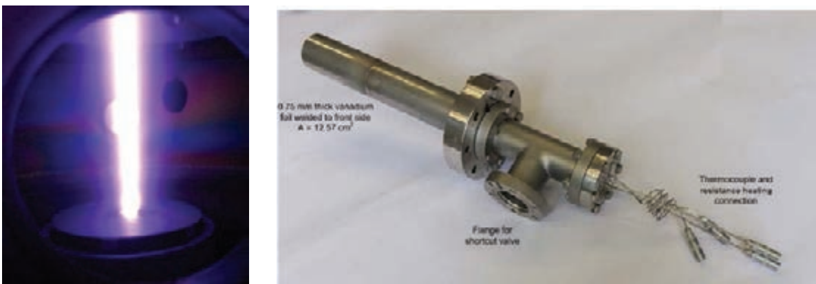
Fig. 4: Photograph of the hydrogen plasma test of a metal foil module (left) and the set-up of the test module itself.
