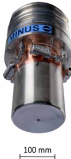
Fig. 2.3: Room temperature terminal of the W7-X HTS current lead prototype.
