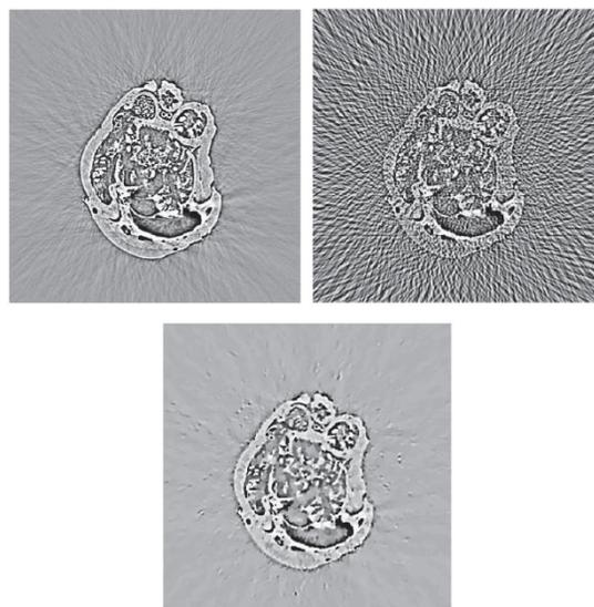
Top left: standard reconstruction with 1500 projections; Top right: standard reconstruction with 60 projections showing artefacts; Bottom: ART-CS reconstruction using 60 projections.
