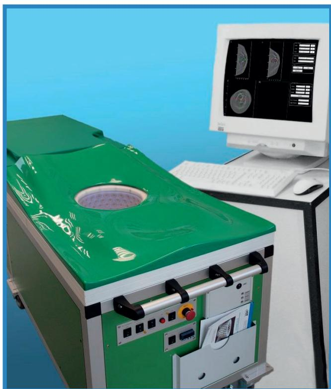
Figure 1: Current 3D USCT prototype which is used for first clinical studies.
