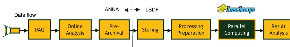
An automatic workflow of the data analysis: parallel computing, marked in dark, proves its efficiency and effectiveness; speedup for a data set reconstruction goes up to 120.
