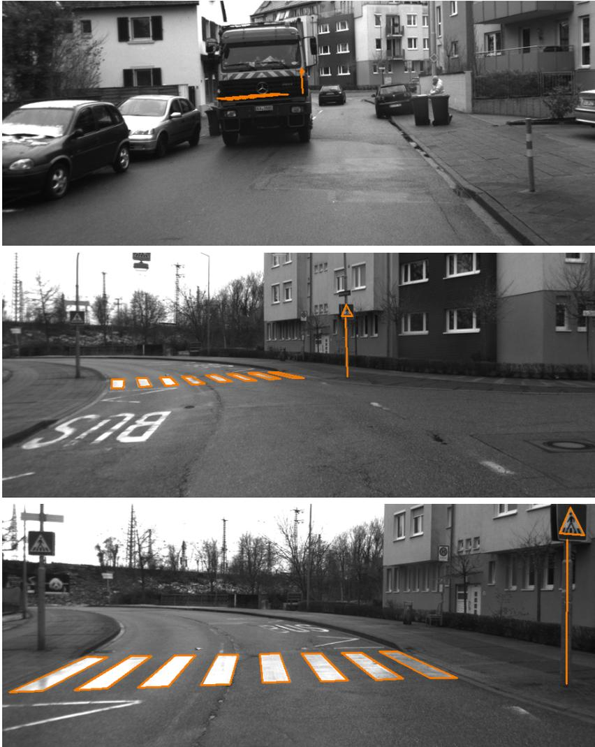
**Figure 5.12:** Results of our AR system are shown. The previously labeled pedestrian crossing is reliably made available during online localization. This approach allows to circumvent any problems caused by occlusion.
