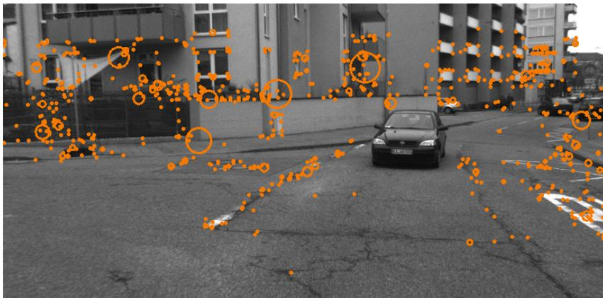
**Figure 4.13:** The pixel positions for which a landmark was estimated are shown for a backward facing camera configuration. All features on the car are correctly identified as non-stationary and are therefore not stored in the map.
