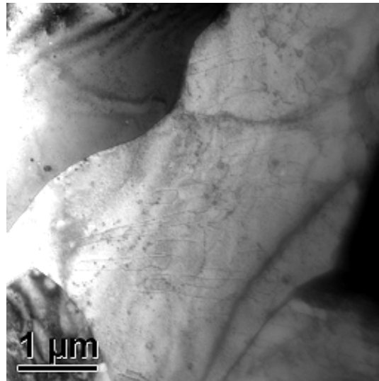
Figure 4.8: Bright field TEM images for the hipped ODS steel K2 (0 Ti).
