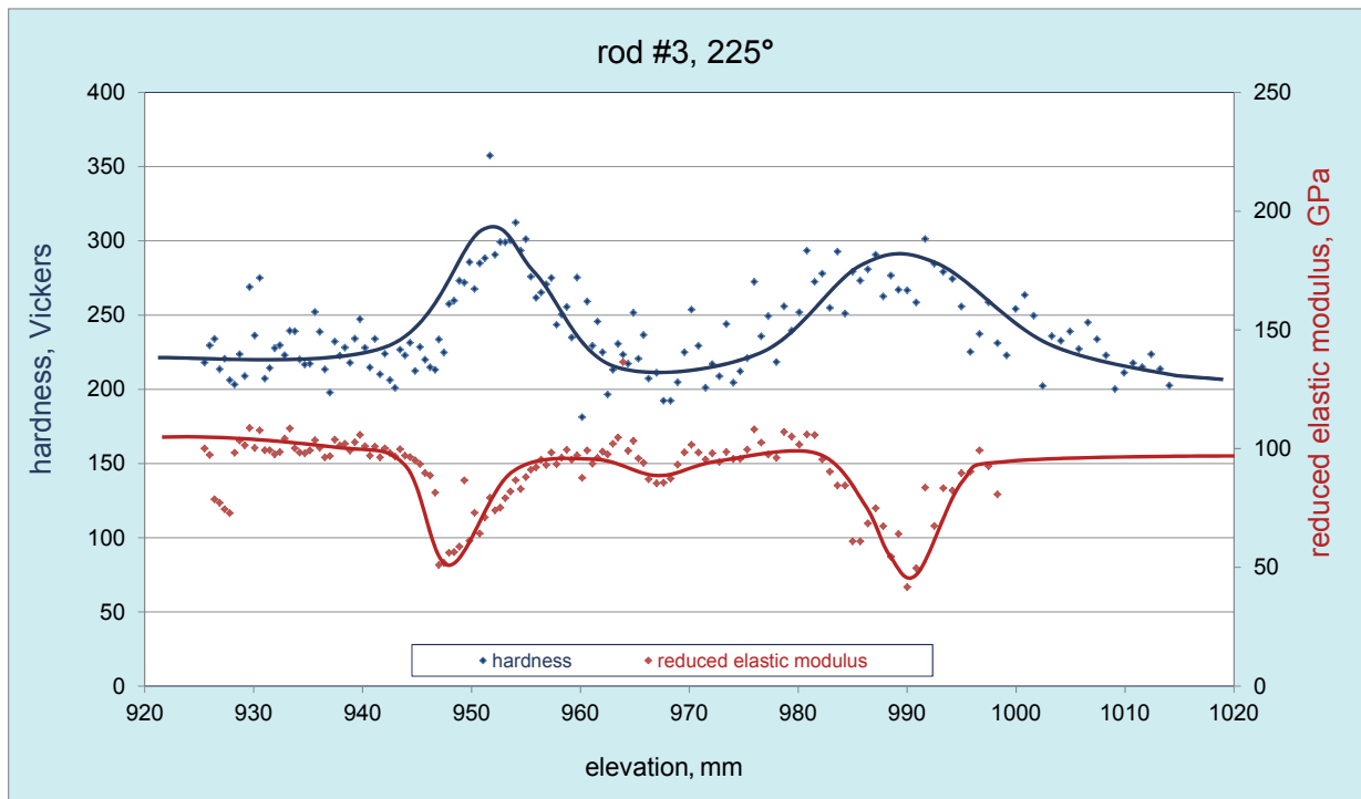
Fig. 109: QUENCH-L0; Microhardness and reduced elastic modulus of rod #3 at 225°.
