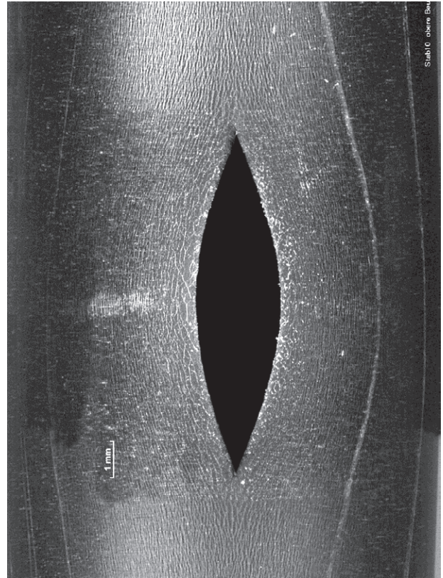
Rod #10 at 77°; p=45 bar, A_{burst}=13 mm 2
