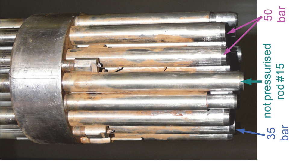
side view at 30°: axial shrinkage of claddings due to Zry anisotropy
