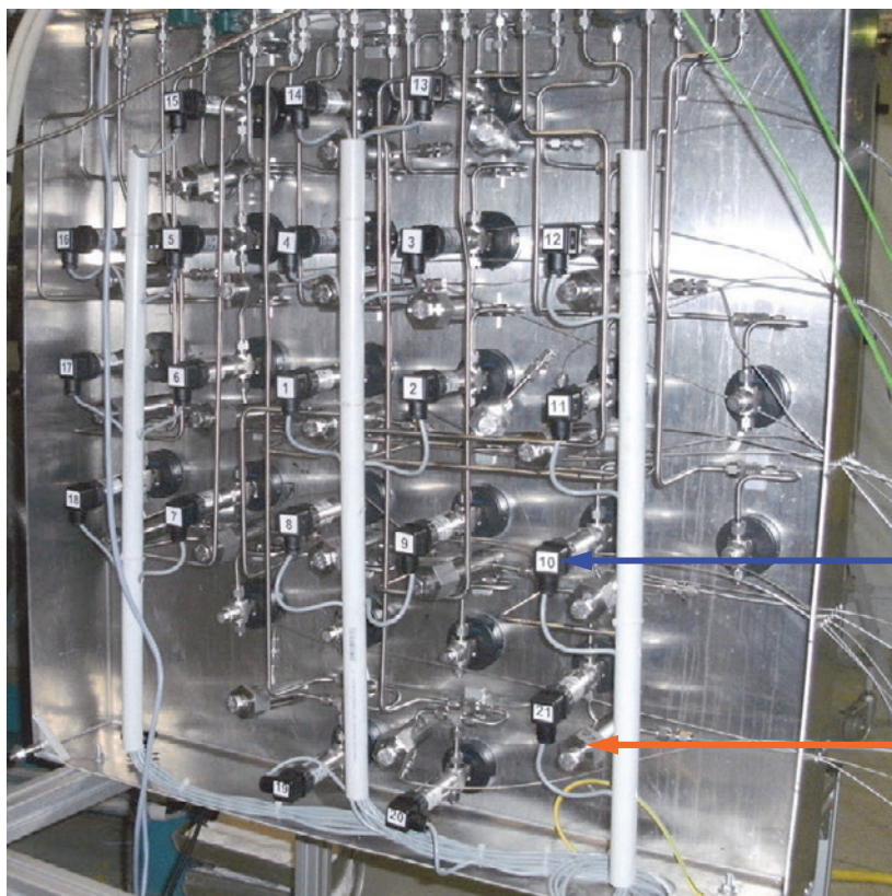
Fig. 7: QUENCH-L0; Rod pressure control and measurement panel.
