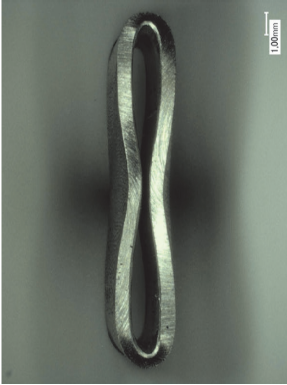
failure caused by plastic instability
