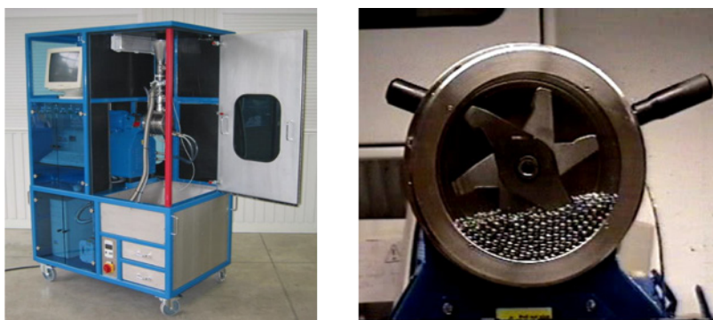
Figure 3.2: Milling equipment. a) High-energy ZOZ Simoloyer CM01 attritor; b) Milling container and milling balls.
