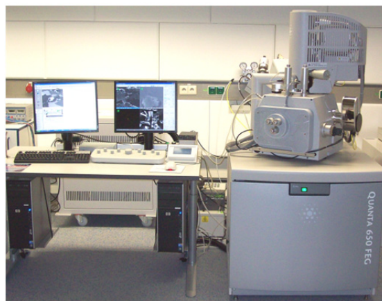
Fig. 1: Environmental scanning electron microscope station in the surface analysis lab in INE active laboratories. The ESEM itself is to the right; top: electron source and column, middle: analytical chamber with docking station for transfer vessel at far right.
