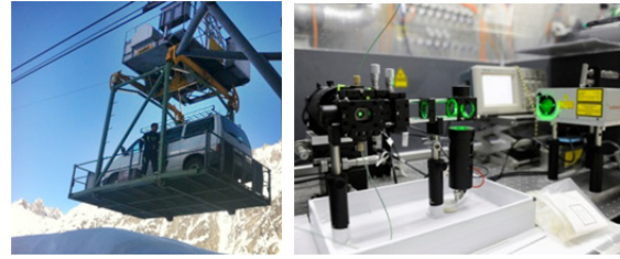
Fig. 2: (left) Transfer of LIBD bus via cable car to the Grimsel Test Site (GTS), (right) LIBD with flow through cuvette for colloid in-line monitoring during Run 12-02.
