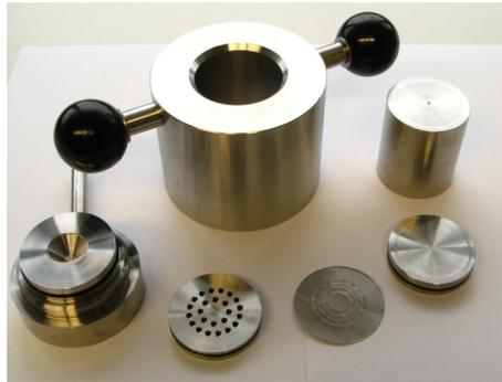
**Figure 5.1.:** Schematic vertical section and photo of the parts of the first press setup for the desalination experiments. The gel is placed in the chamber and squeezed from the top. The water is discharged through the sieve and drainage at the bottom. Fractions are collected while the polymer remains in the chamber.
