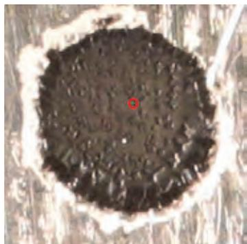
**Figure 8:** Magnetite sample for XPS. Red circle marks the place of analysis.
