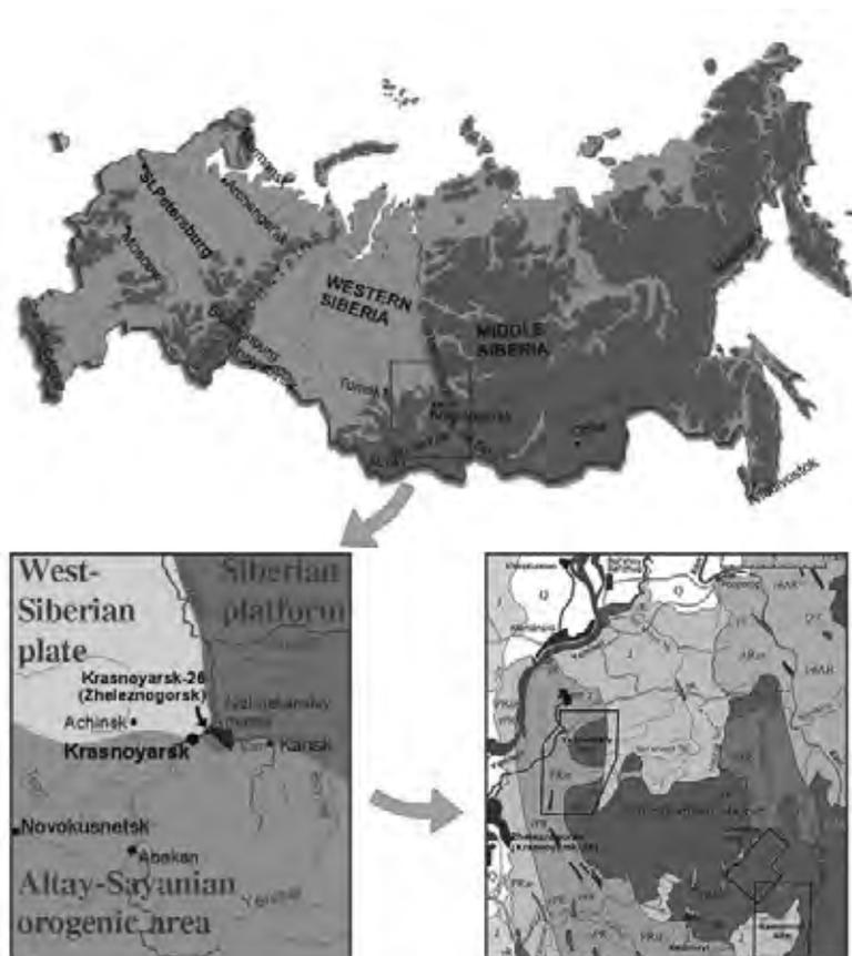
**Figure 1:** Location of Nizhnekansky granitoid massif and three proposed sites for SNF final geological disposal (Yeniseisky, Itatsky and Kamenny sites. Based on (Jardine, 2005).
