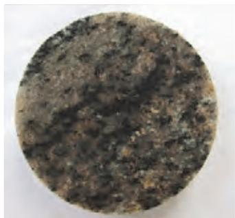
**Figure 1:** Sample AD-1 for electromigration measurement.
