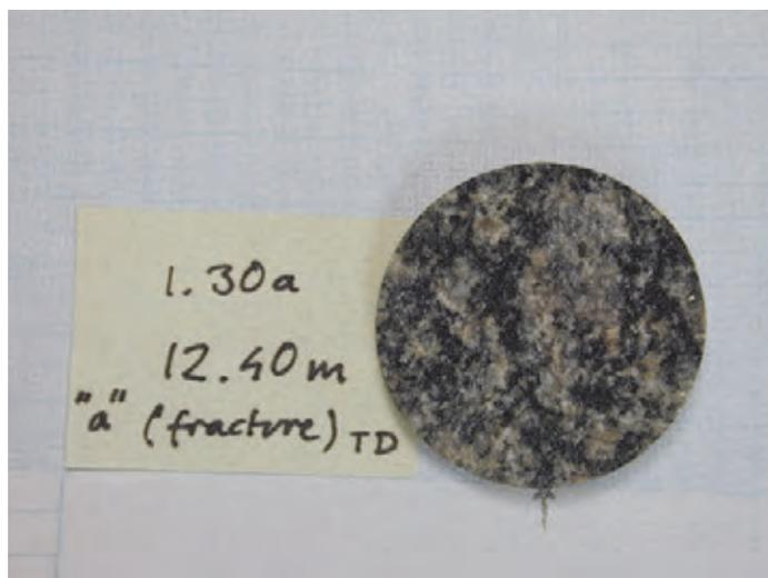
**Figure 2:** Fracture surface at the end of drill core section at 12.40m in borehole KA2368A-01, viewed in tunnel direction.
