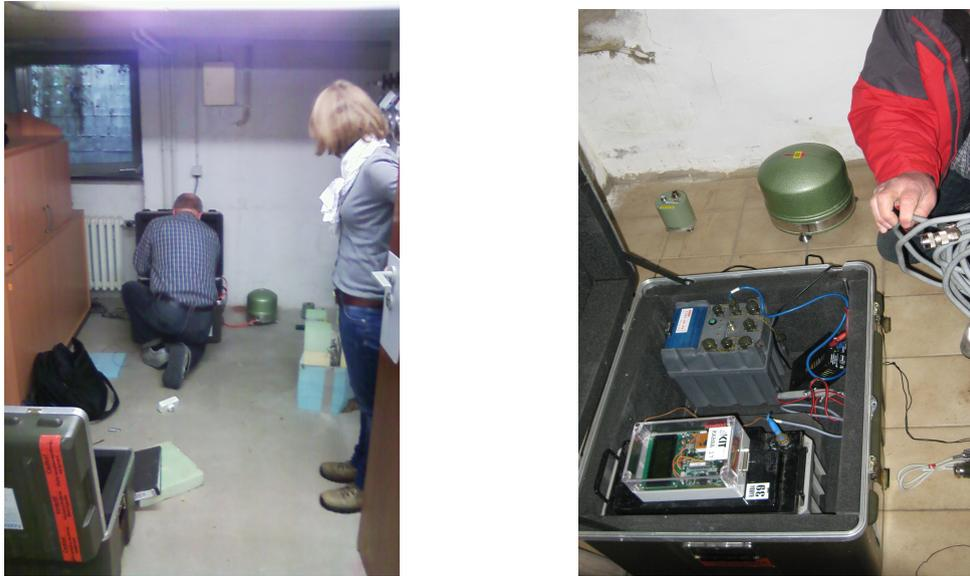
Figure 3.3.: Installation of TMO66 in the cellar of the Julius Kühn-Institute (left). Installation of the TMO67 station in the cellar of the Sportheim Eschbach (right). On both pictures you can see the big Streckeisen STS-2 and the smaller Trillium Compact broadband sensors.
