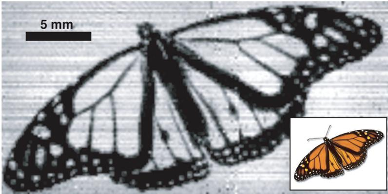
**Figure 8.3.:** Near-infrared shadow cast at 1310 nm of a transparent slide showing a monarch butterfly (cf. original slide in the inset).
