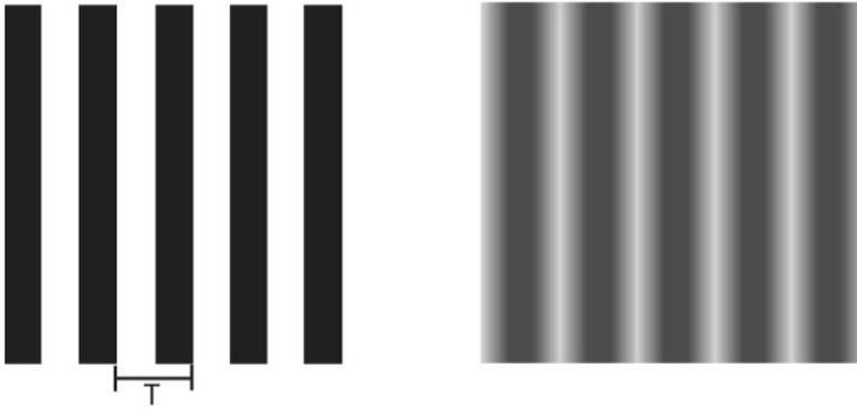
**Figure 3.13.:** Pattern for modulated transfer function measurements (**left**) and an expected reproduced pattern by the imager with fading the transition of the MTF pattern (**right**).
