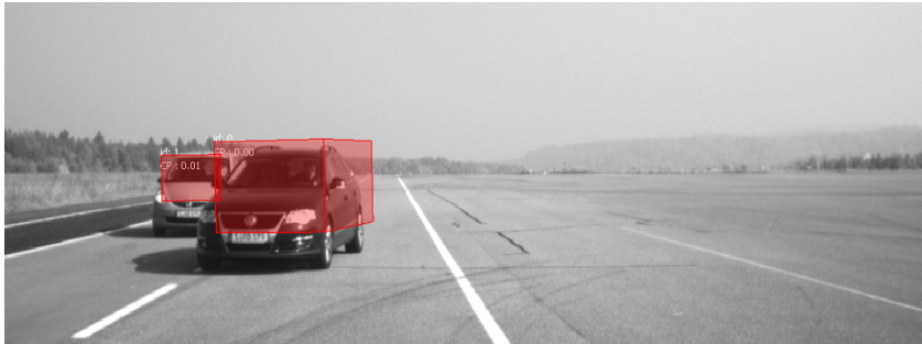
Figure 6.8: One of the scenes from use case 3 when a match with the query collision between two parallel moving objects is found. The distance between them is 4.4m .
