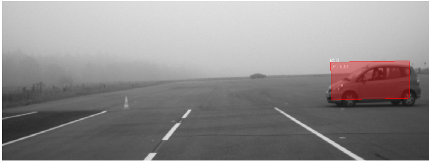
Figure 4.7: Example frame from the test sequence. Red filled rectangle represents the object that has high probability of collision with ego vehicle if both vehicles continue to behave in the same manner.
