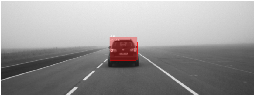
Figure 6.6: One of the scenes from use case 2 when a match is found. The distance of the ego vehicle to the other vehicle is 31m .
