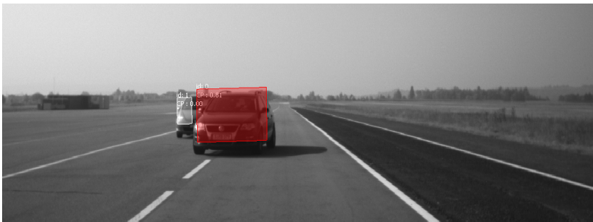
Figure 6.7: One of the scenes from use case 3 when a match with the query for collision between ego vehicle and object is found. The distance between them is 22m .
