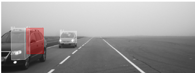
Figure 6.12: Example of a scene where an incorrect segmentation leads to incorrect recognition in “use case 3 q1”
