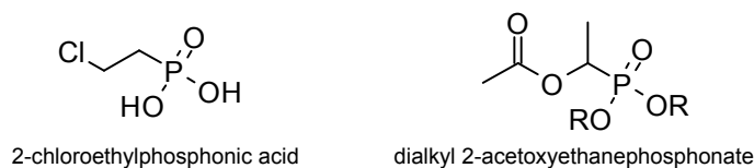
Figure 2.38: Chemical structures of 2-chloroethylphosphonic acid (left structure) and dialkyl 2-acetoxyethanephosphonates (right structure).
