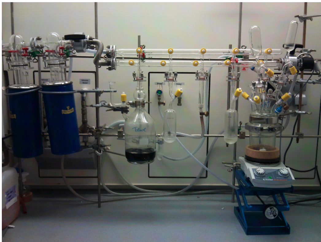
Figure 4.27: Apparatus for the living, anionic polymerization containing (from left to right) two cold traps and Dewar flasks, a 2-liter storage glass vessel for extra dry toluene, several flanges with Young taps and the reaction vessel with one connection to the Schlenk line and four access points for the connection of compound vessels.
