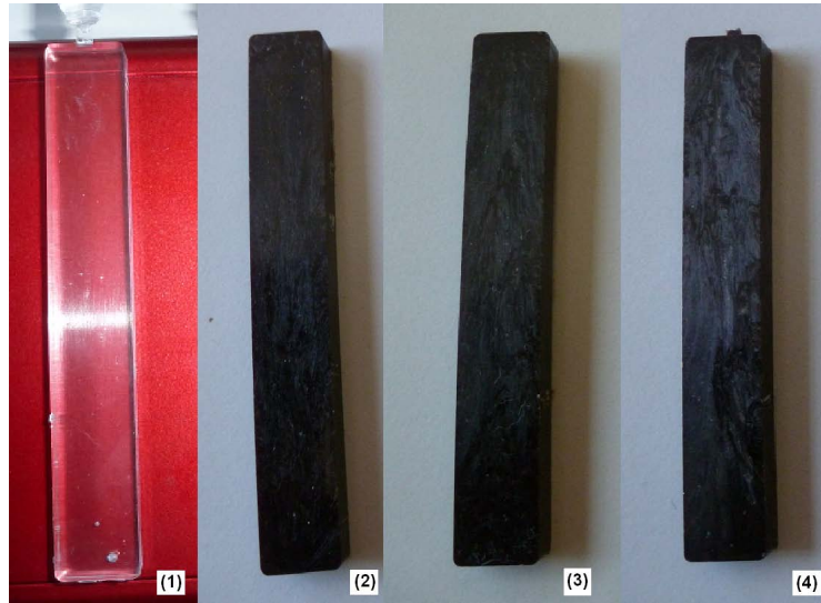
Figure 5.5: Pictorial representation of the molded pure polystyrene (1) and the molded flame retardant-polystyrene samples (PS-DPPP)-PS with flame retardant contents of 18.5 % (2), 37.3 % (3) and 41.2 % (4).
