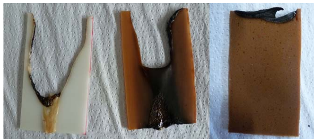
Figure 5.14: Pictorial representation of the reference pure polyurethane (PUR) sample (left) and the flame retardant (PS-DPPP)-PUR samples (middle = 10 parts PS-DPPP; right = 40 parts PS-DPPP) after LOI measurements at 19.2.
