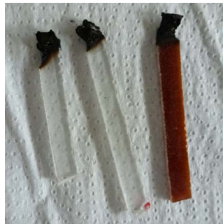
Figure 5.11: Pictorial representation of the polymerized epoxy resin (PEpo) (left & middle) and the flame retardant (PS-DPPP)-PEpo sample (right) after LOI measurements.
