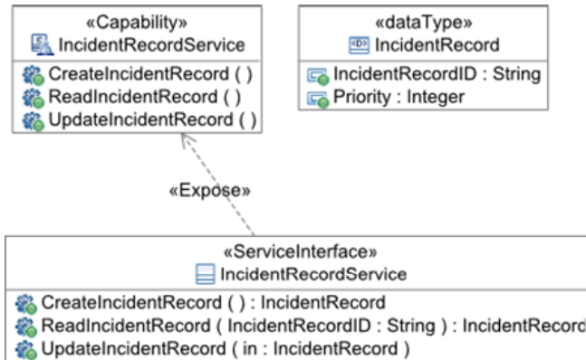
Figure 8. Domain-driven Design of a Management Service for Incident Management
