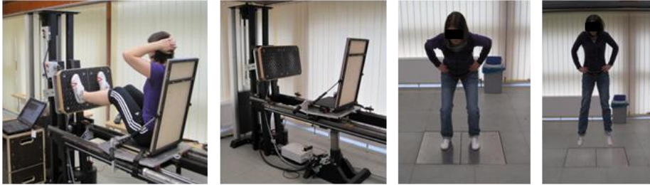
Figure 5: Female participants during isometric (leg press) and dynamic (counter-movement-jump) lower limb strength testing
