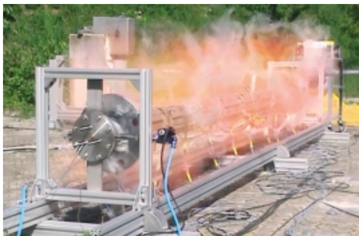
Wasserstoff-Explosionsversuch in der PET-Anlage (Partially vented Explosion Tube).
