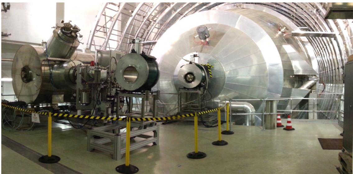
**Figure 3.11: Panoramic photo of pre-spectrometer setup.** Photo of the shifted pre-spectrometer. For measurements with the *Münster electron source*<sup>a</sup> the flux tube must be contracted. Hence, in this special case both magnets are operated in standalone mode.
