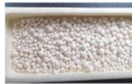
Obtained pebbles after sintering
