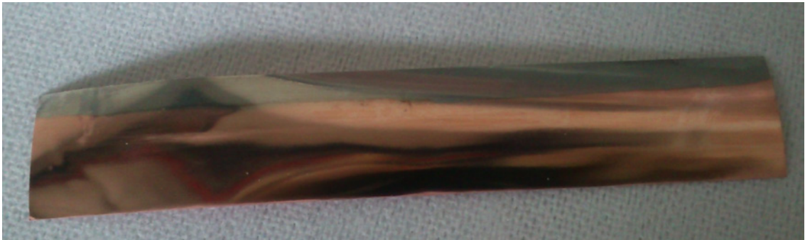
Figure 4.24: Stainless steel transition foil after brush plating with nickel and copper
