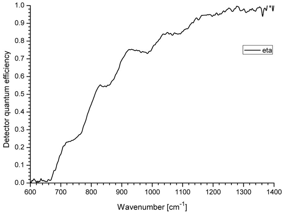
Figure 5.29.: Detector quantum efficiency for pixel (119,121) of detector II/2. The measurement was done for a detector integration time of  $34.1 \mu\text{s}$ .
