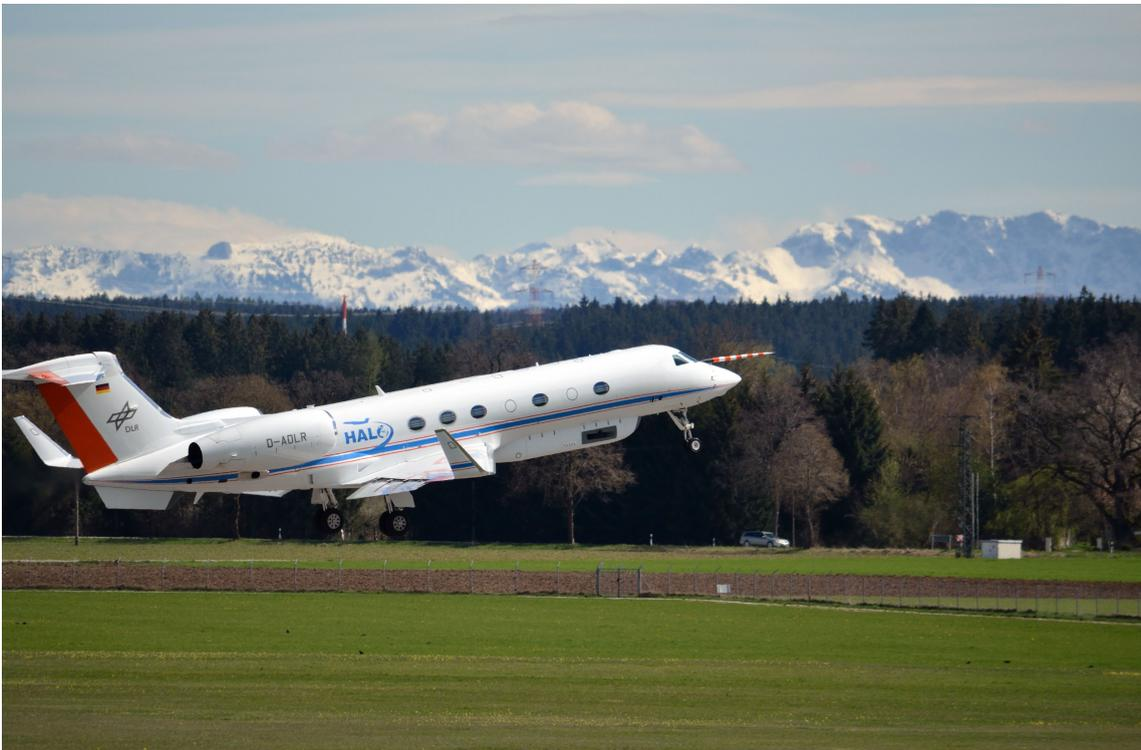
Figure 3.13.: HALO research aircraft with GLORIA in the belly pod. GLORIA is measuring in the limb mode looking to the right side of the flight direction.
