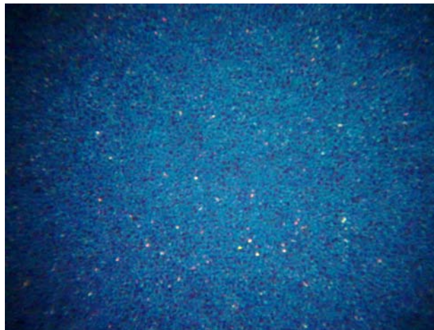
Figure 5.27: Example of reflection pattern from r-PUF, FoV \sim 10\text{mm} \times 8\text{mm}
