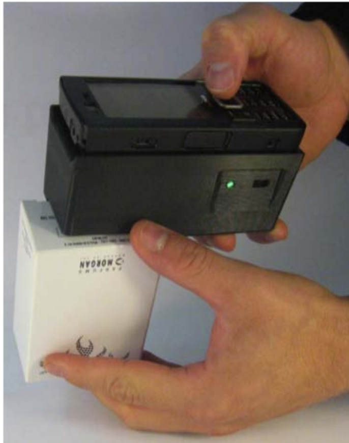
Figure 6.1: One of the early version of add-on in operation showing the positioning of the package for verification. Source: Informium AG
