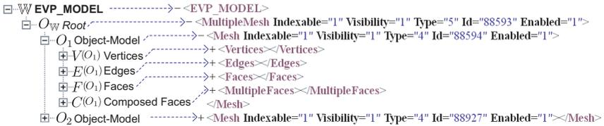
**Figure 3.31:** XML serialization of the world model representation. The arrows show the correspondence between mathematical concepts and implementations. This XML shows two object models from figure 3.23.
