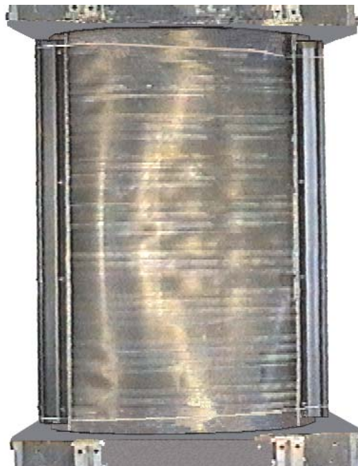
Figure 16: Experimental buckling state of the carbon fiber reinforced panel (from DLR)
